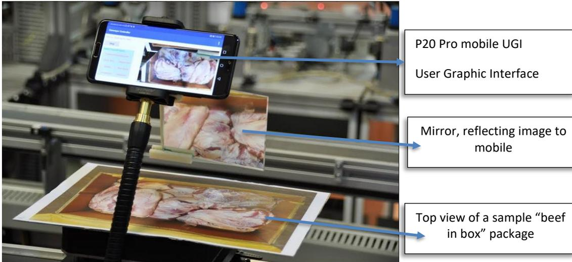
Figure 12. A close up view of, the conveyor loop with HUAWEI P20 pro system, mirror, holder, image of a beef in box.
