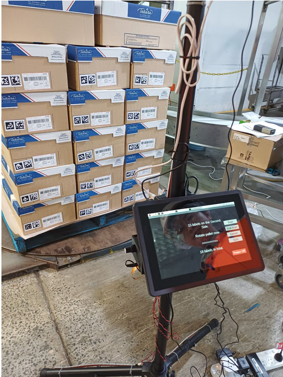
Figure 5 – Pallet Reader scanning pallet on the turntable.
