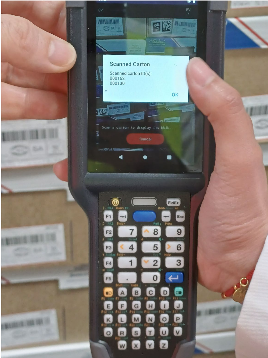
Figure 6 – CK65 handheld scanning cartons.
