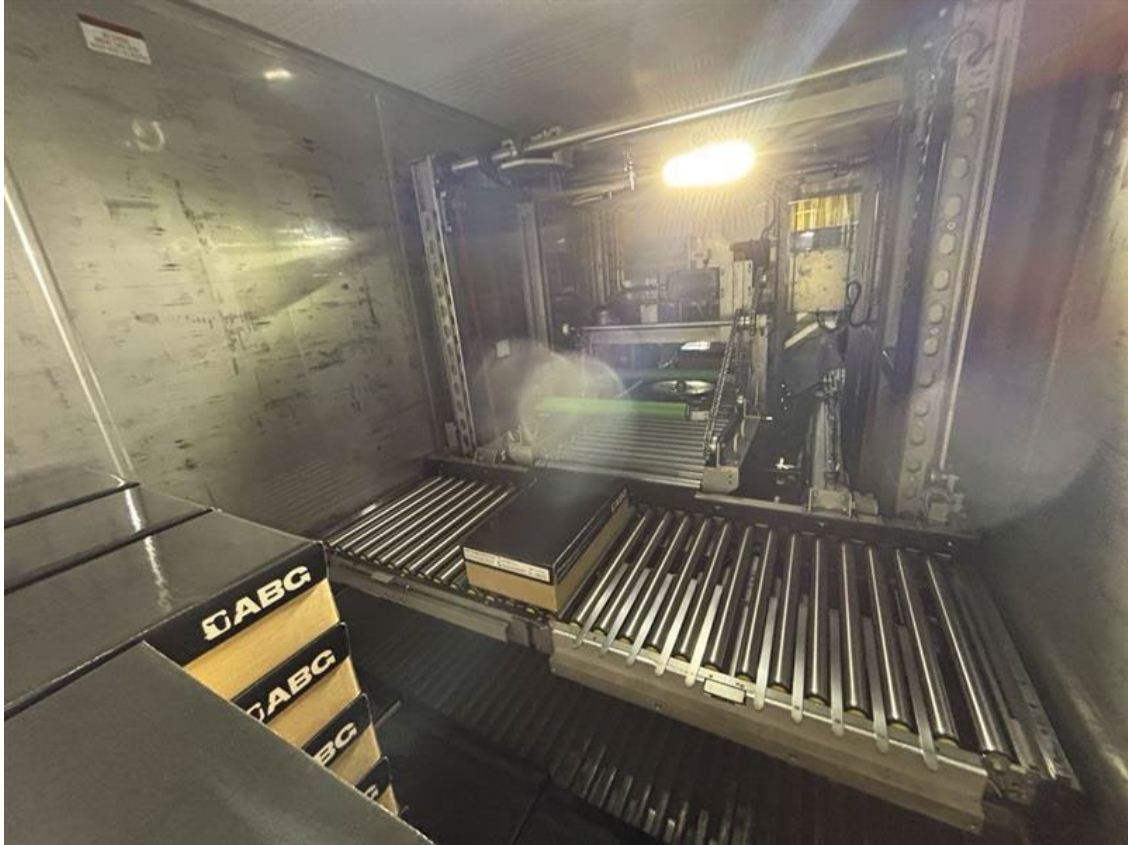
View of Loader from Carton Stack: tines retracted
