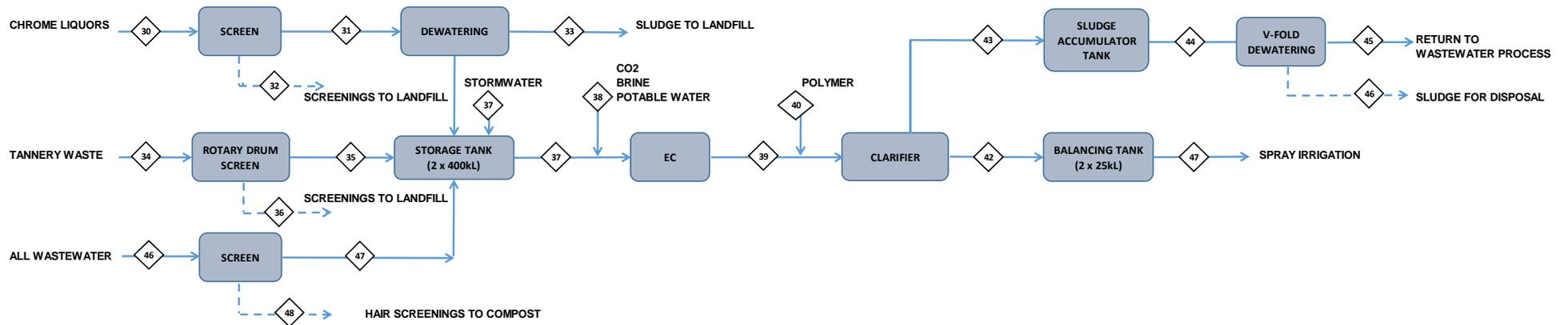
Fig 3 Tannery Process Flow Diagram
