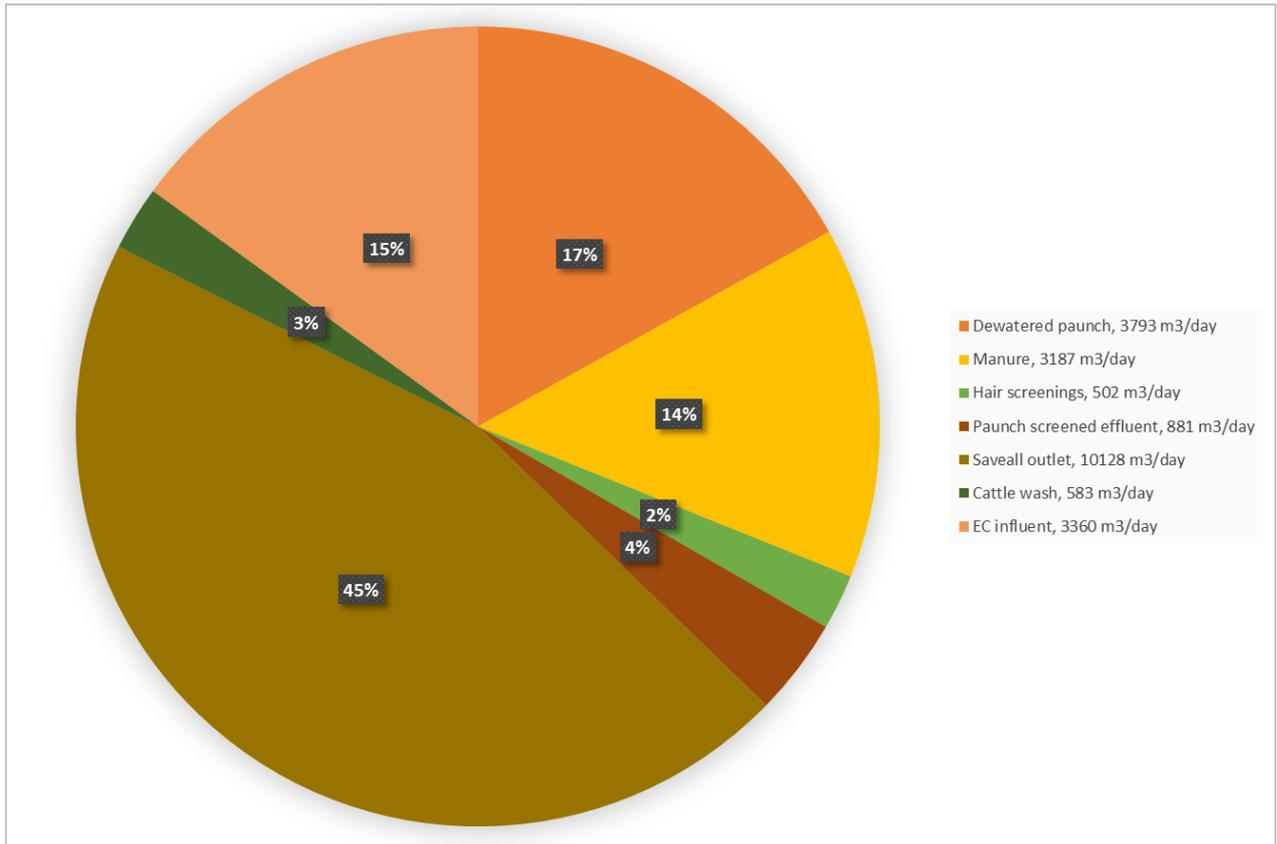
**Fig 5 Relative contribution of biogas production from each stream (Scenario 1b)**
