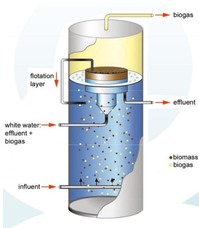
**Fig 8 Schematic of Anaerobic Flotation Reactor (Paques BIOPAQ®)**
