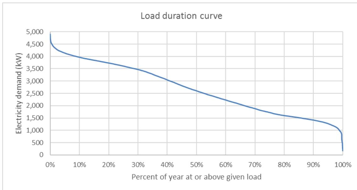
**Fig 16 Load duration curve**
