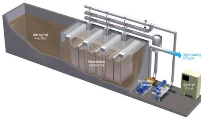
**Fig 9 Anaerobic Membrane Reactor (Membrane Europe Ltd.)**
