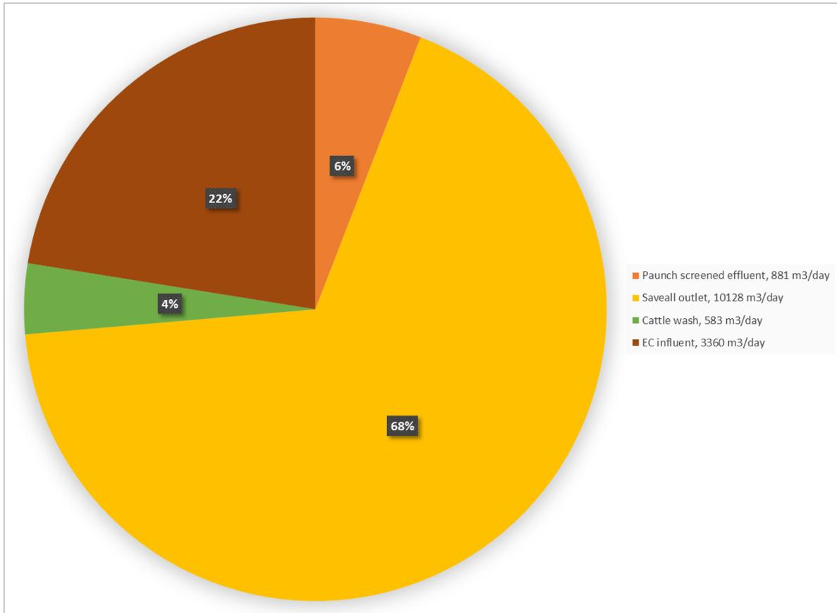
**Fig 6 Relative contribution of biogas production from each stream (Scenario 1c)**
