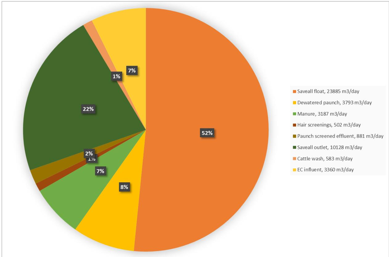
**Fig 4 Relative contribution of biogas production from each stream (Scenario 1a)**
