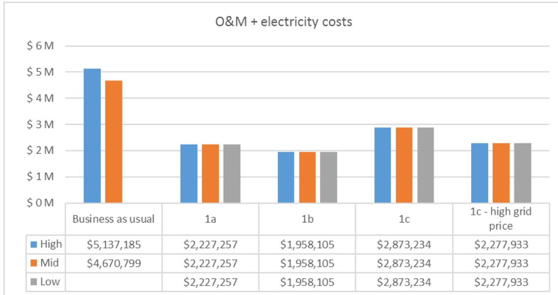
**Fig 21 Annual O&M and electricity cost comparison**
