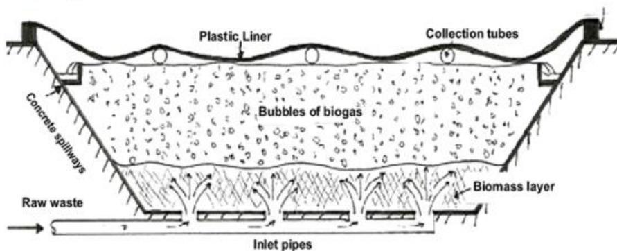
**Fig 7 Schematic of Covered Anaerobic Lagoon**
