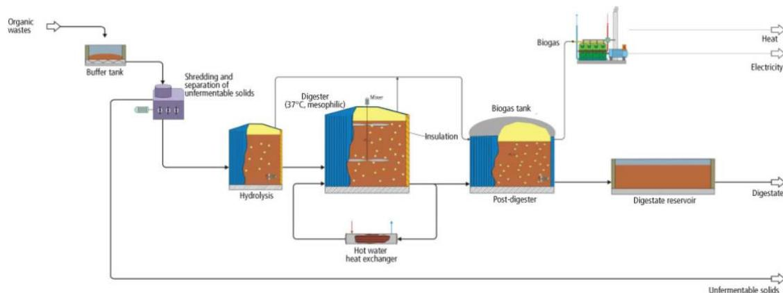
**Fig 10 Schematic of Continuously Stirred Tank Reactors (CSTR) - Generic**
