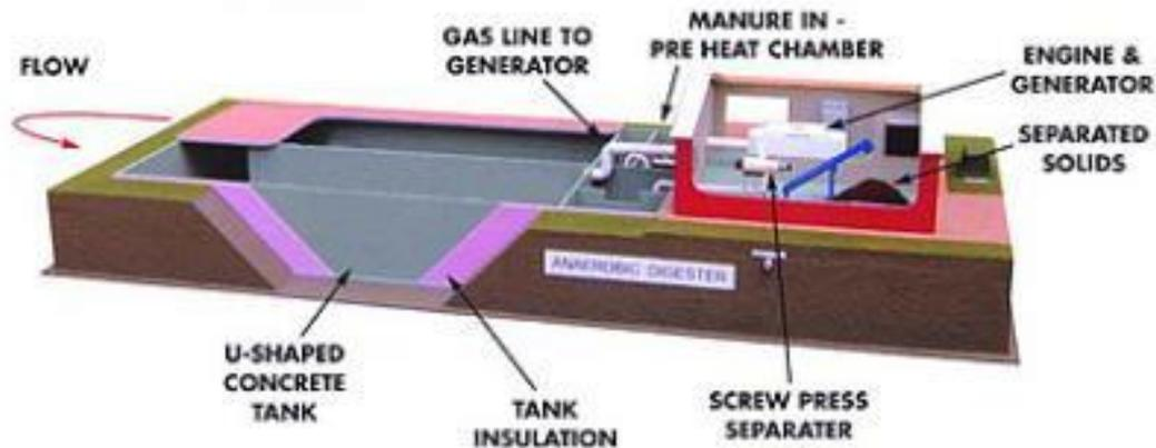
**Fig 12 Schematic of Mixed Plug Flow Reactor (DVO)**
