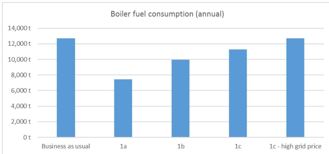
**Fig 26 Annual boiler fuel consumption comparison**
