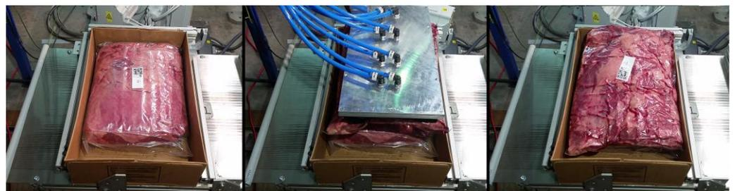
Figure 4: Flat packing process (left to right) for Clod
