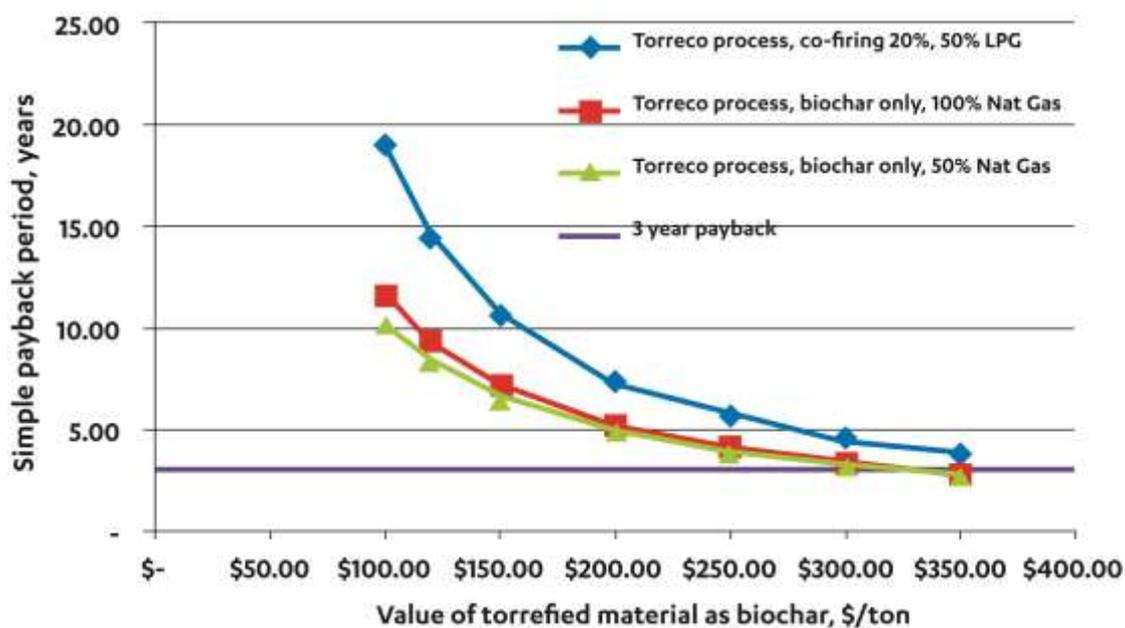
**Figure 7.** Effect of sale price of torrefied material as biochar on simple payback period for the project.
