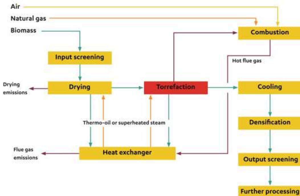
Figure 5. Typical process flow sheet – Indirect heating (From [8])
