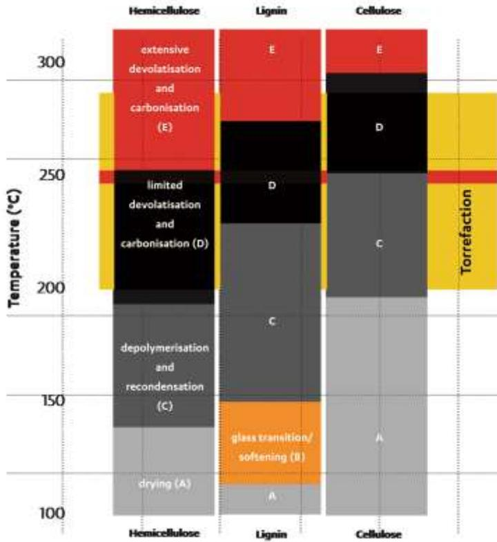
**Figure 3.** Physiochemical changes in biomass during torrefaction (From [9])
