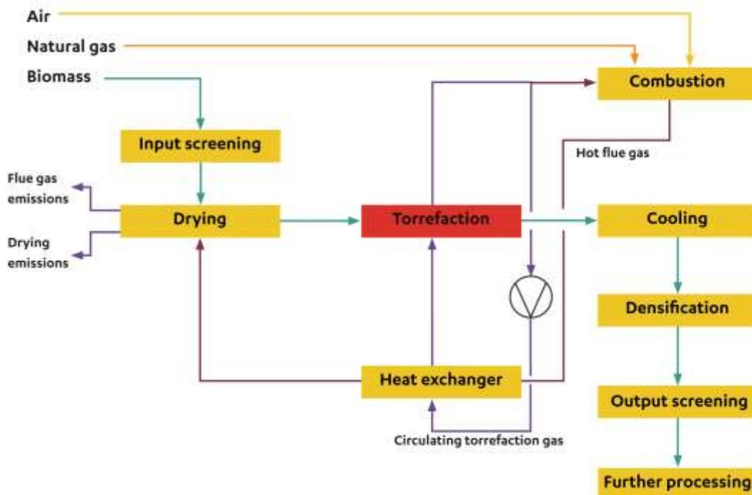
Figure 4. Typical process flow sheet – Direct heating (From [8])
