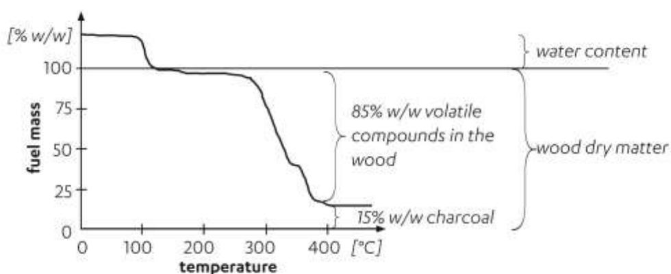
**Figure 1.** Typical thermal gravimetric analysis of wood undergoing pyrolytic decomposition (From [8])
