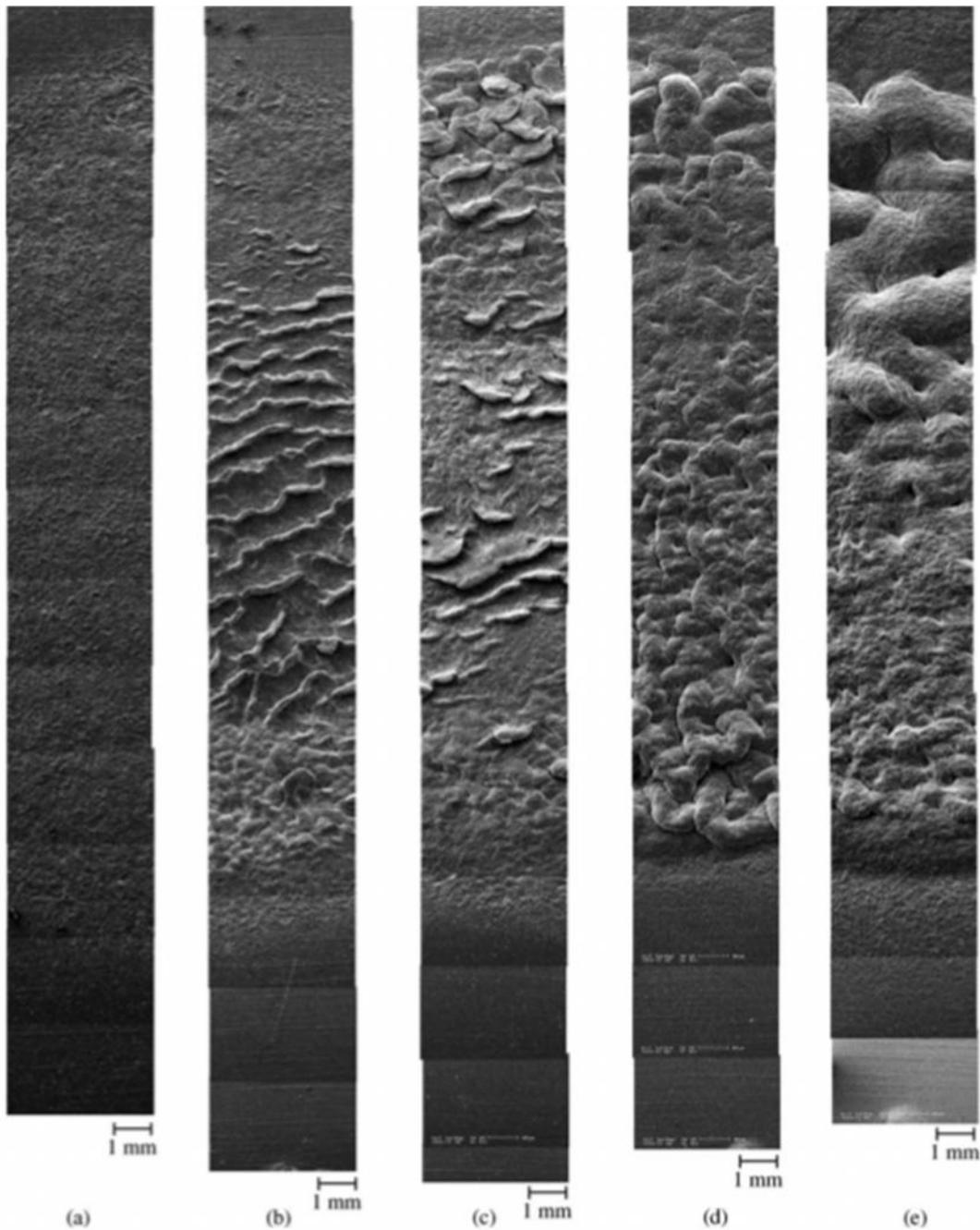
Figure B1. SEM composites of wear scars on polypropylene from Western et al (2005). Figures (b) and (c) provide examples of the precursor of potential flaking, as an indicator of possible failure.
