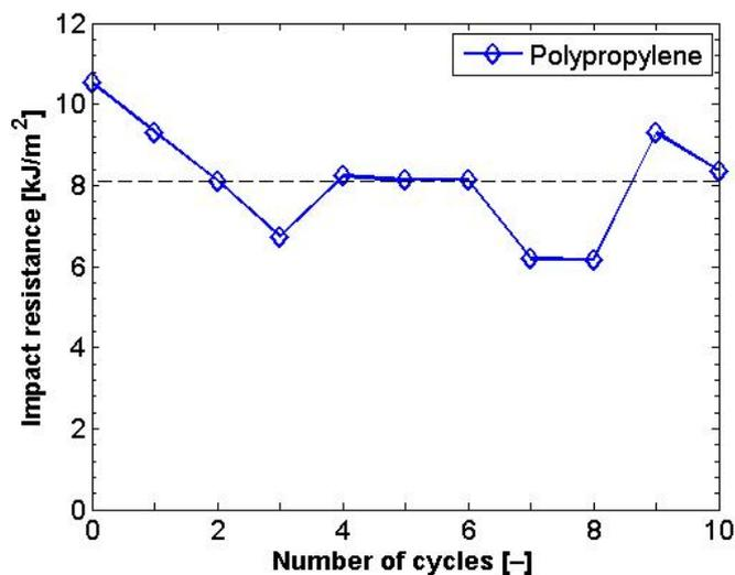
**Figure 1:** Impact resistance of polypropylene as a function of the number of thermal-loading cycles.
