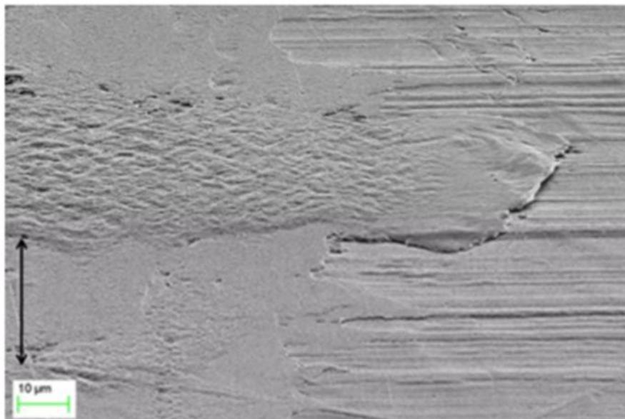
Figure B3. SEM of surface defects, including ploughing (left hand side of image) and flaking (right hand side of image) (Lind *et al.*, 2015).
