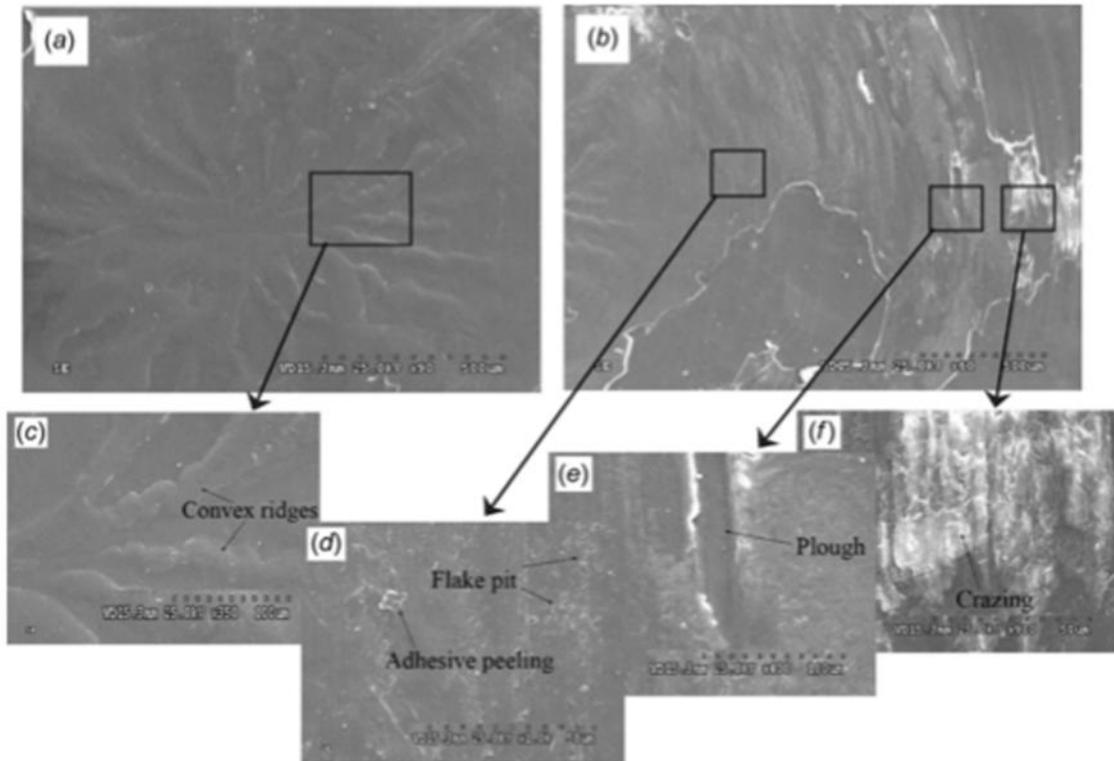
Figure B2. SEM morphologies of surface defects, including ridges (c), flaking/adhesive peeling (d), pitting/flake pit (d), pitting/plough (e) and crazing (f) (Liu *et al.*, 2019).
