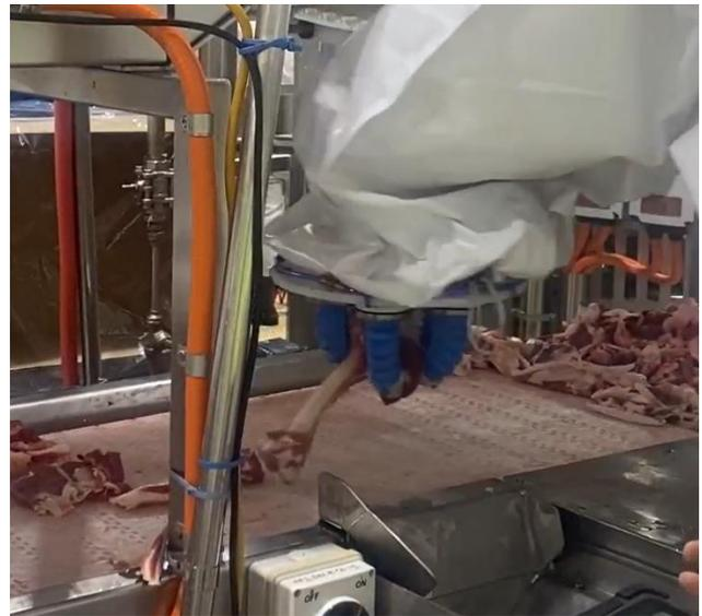
The remote, operator-controlled shadow robot picking from a conveyor belt.
