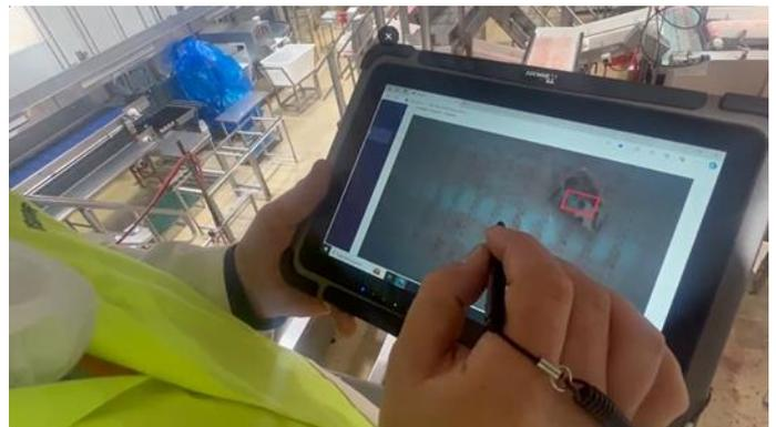
Photo showing an operator selecting parts for the robot to pick from the conveyor. Here the shadow robot operator is in the boning room but remote from the robot.
