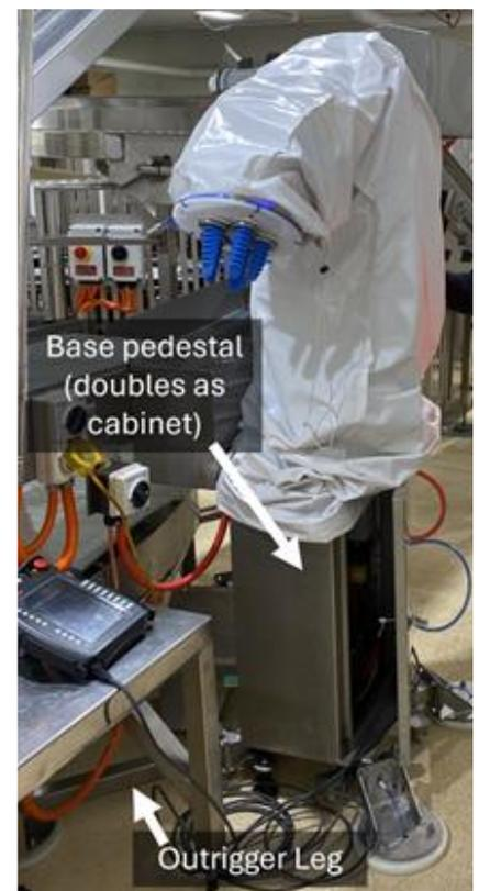
Photo of the shadow robot and associated base where the pedestal cabinet and outrigger legs are visible.
