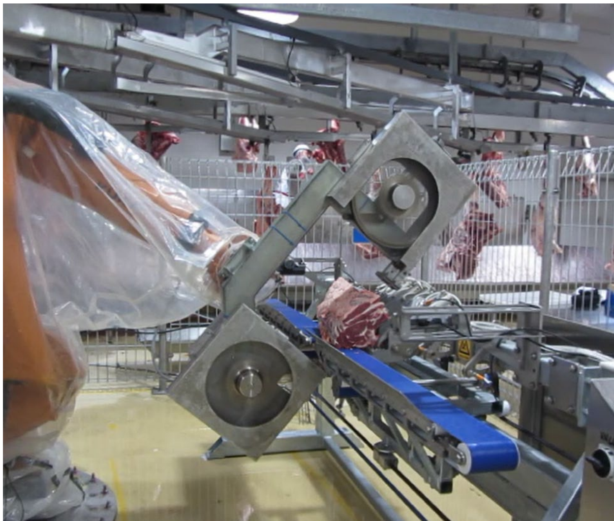
Figure 16: Striploin chine bone removal concept prototype cell at an Australian processor.
