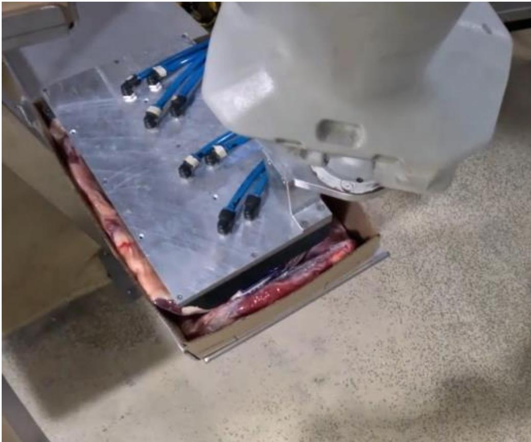
*Figure 18a: Robot flat packing to lower carton location.*
