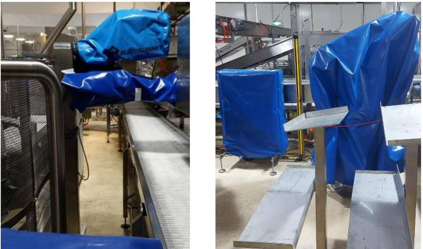
Figure 10: Washdown covers for camera and lights (left), control cabinet and robot (right)
