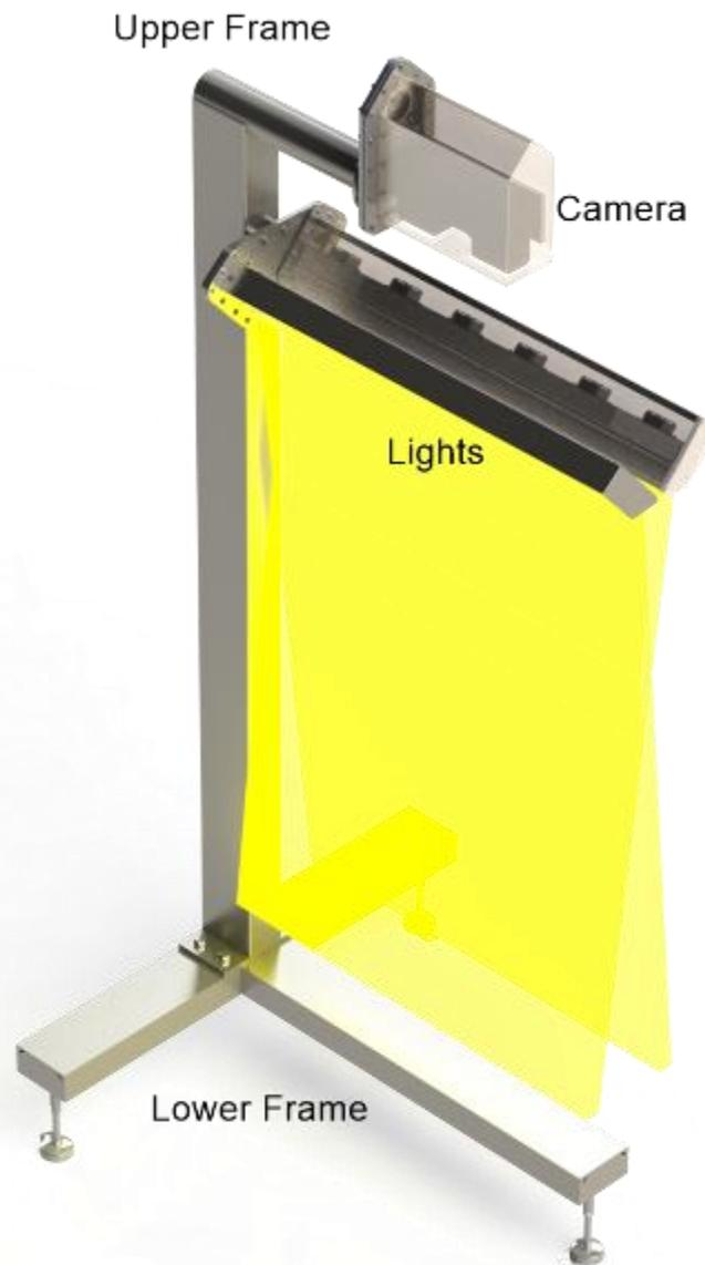
Figure 8: Rendering of camera and lights frame design. Camera and light covers are transparent to show details of the camera and lights respectively.
