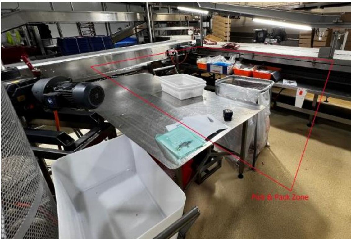
Figure 2: Proposed robotic cell packing region.
