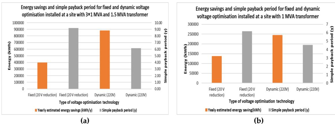
**Figure 27: Annual energy savings and simple payback period when applying fixed voltage optimisation and dynamic voltage optimisation with a set voltage of 220V installed at a abattoir in (a) WA and (b) QLD**
