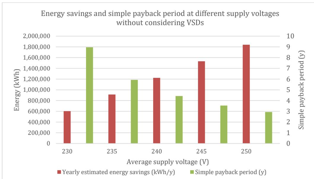
**Figure 22: Annual energy savings and simple payback period when applying dynamic voltage optimisation (3 x 1 MVA and a 1.5 MVA unit) with a set voltage of 220V installed at a medium-sized abattoir without considering the effect of VSDs on the load for a range of supply voltages**
