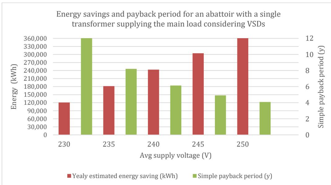
**Figure 25: Annual energy savings and simple payback period when applying dynamic voltage optimisation (1 MVA unit) with a set voltage of 220V installed at an abattoir with a single transformer supplying the main load with consideration of the effect of VSDs on the load for a range of supply voltages**
