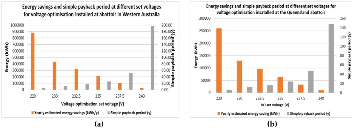
**Figure 26: Total site energy savings for different VO set voltages when the supply voltage is 240 V for abattoir in (a) WA and (b) QLD**
