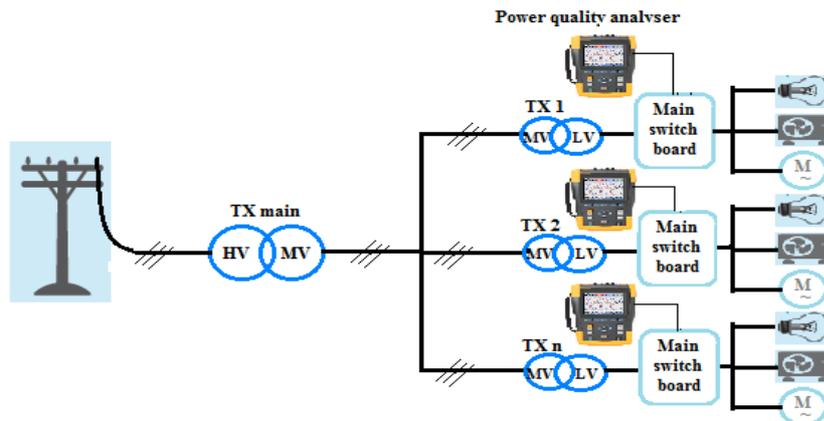
Figure 6 – Data collection from case study 1 abattoir using a Fluke Power Quality Analyzer
