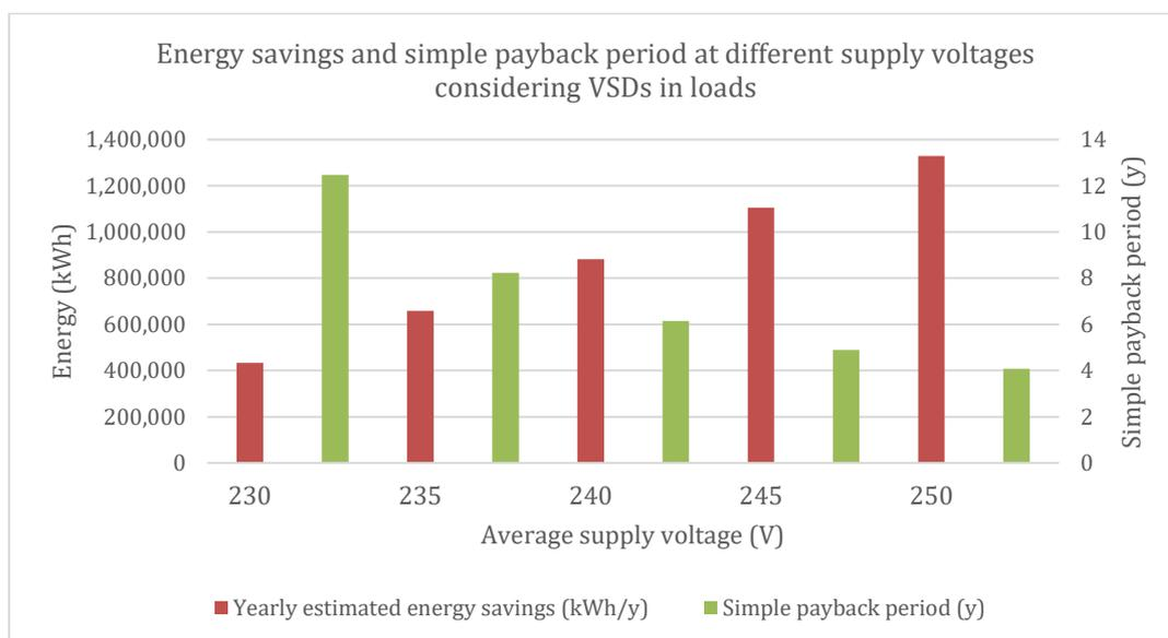
**Figure 23: Annual energy savings and simple payback period when applying dynamic voltage optimisation (3 x 1 MVA and a 1.5 MVA unit) with a set voltage of 220V installed at a medium-sized abattoir with consideration of the effect of VSDs on the loads for a range of supply voltages**
