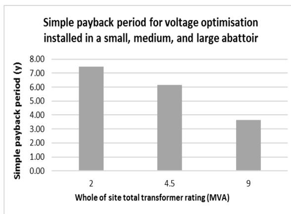
**Figure 29: Simple payback period when applying dynamic voltage optimisation with a set voltage of 220V installed at small, medium, and large abattoir with VO units of 2 MVA, 4.5 MVA, and 9 MVA respectively**
