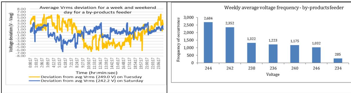
**Figure 13: Deviation from the average  $V_{RMS}$  on a week and weekend day for a transformer with a by-products load at a medium-sized abattoir**
