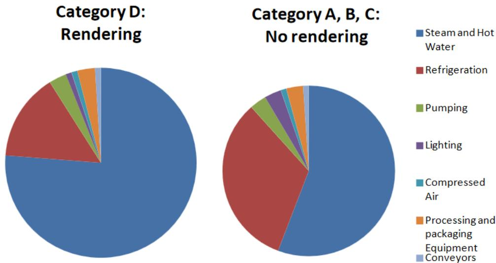
**Figure 2: Breakdown of energy consumption by major energy service or equipment for rendering and non-rendering sites [reproduced from 1]**
