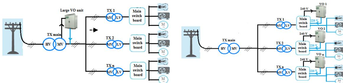
**Figure 5: Possible location of VO unit installation in a typical abattoir (a) with main transformer and (b) with individual LV transformer**
