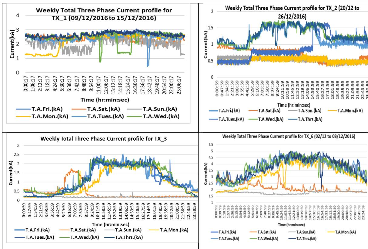
Figure 7 – Weekly current profiles for refrigeration (TX1), kill floor (TX2), by-products (TX3) and general distribution (TX6) feeder transformers
