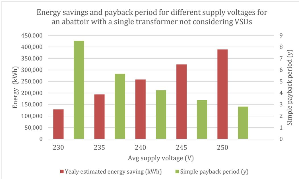
**Figure 24: Annual energy savings and simple payback period when applying dynamic voltage optimisation (1 MVA unit) with a set voltage of 220V installed at an abattoir with a single transformer supplying the main load without considering the effect of VSDs on the load for a range of supply voltages**
