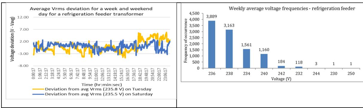
**Figure 9: Deviation from the average VRMS on a week and weekend day for a transformer with a mostly refrigeration load at a medium-sized abattoir**
