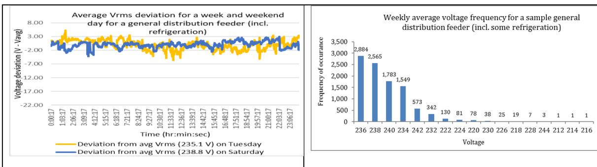
**Figure 15: Deviation from the average  $V_{RMS}$  on a week and weekend day for a transformer with a general distribution load (including some refrigeration) at a medium-sized abattoir**
