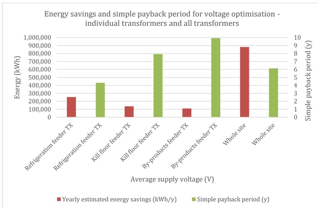
**Figure 21: Annual energy savings and simple payback period for voltage optimisation units installed at refrigeration, kill floor, and by-products feeder transformers (1 MVA units) as well as at the whole site**
