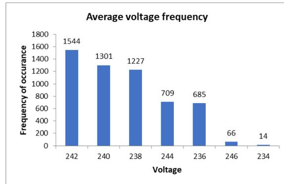
**Figure 20: Average voltage frequency for a transformer connected to the main load**
