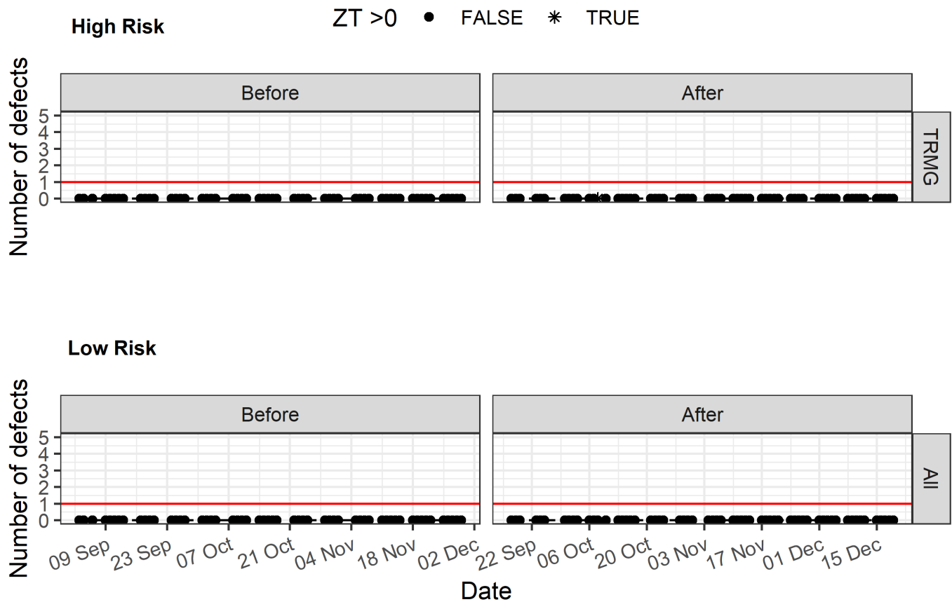
Figure 3.3: Time plot of daily defects for high and low risk carton products; stars indicate detection of ZTs and the red line indicates the unacceptable limit.
