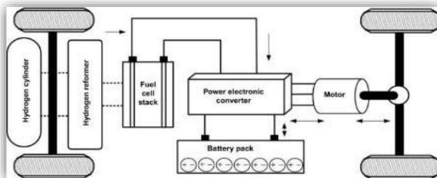
Figure 3: Schematic of a Fuel Cell-Electric Vehicle (FCEV)<sup>10</sup>.
