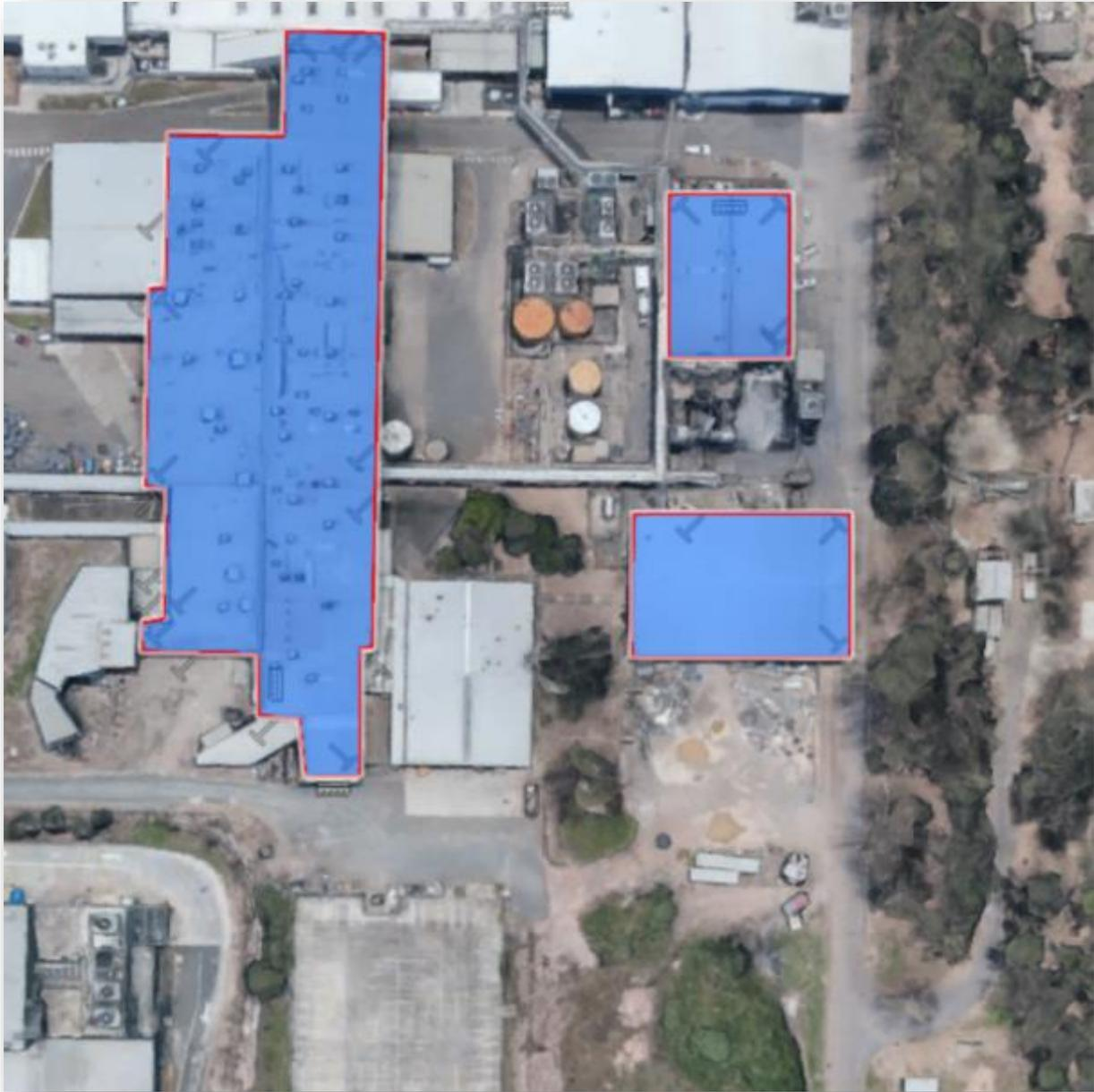
Figure 12: Indicative area requirement for PV array to power 1 MW electrolyser
