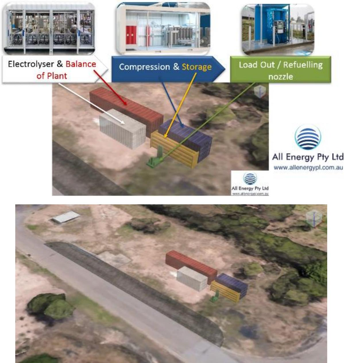
Figure 11: 1 MW electrolyser indicative Option 1 layout orthographic views.
