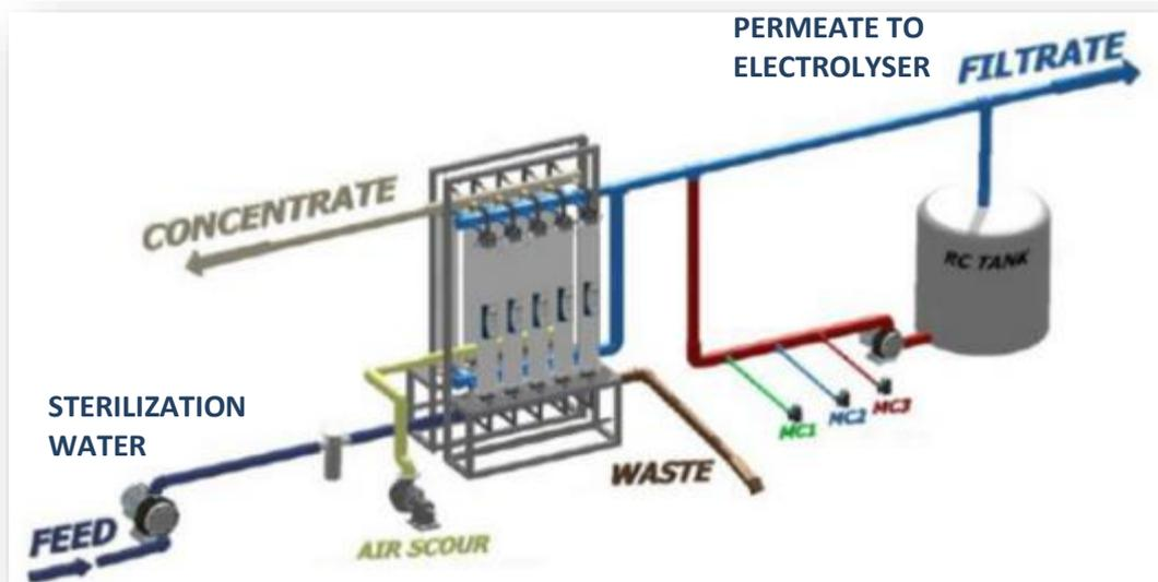
Figure 38: MAK Electrolyser Feedstock Water Pre-Treatment Schematic
