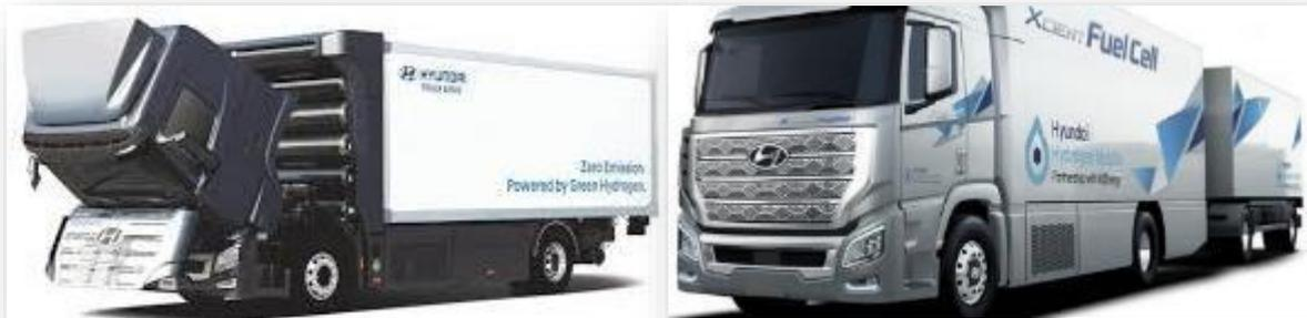
Figure 9: Hyundai Hydrogen Truck in rigid and semi-trailer configuration.
