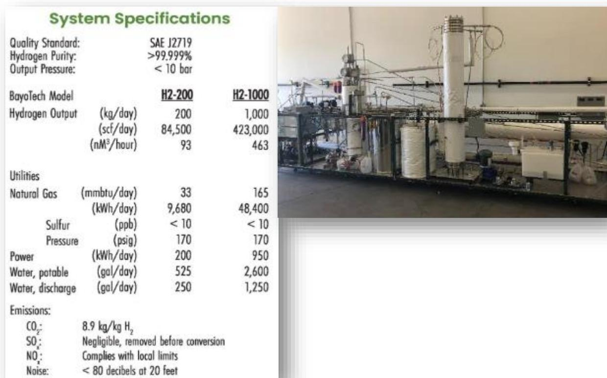
Figure 21: Hazer modular biogas reformer system specifications
