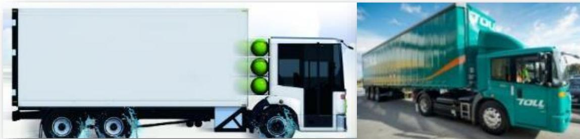
Figure 11: Econic refrigerated box option showing the H<sub>2</sub> storage (green Fibre Reinforced Polymer tanks or FRPs) and the Econic in a semi-trailer format.
