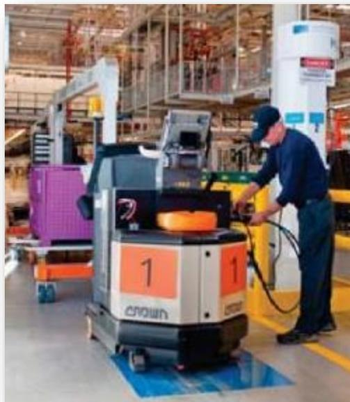
Figure 6: A FCEV forklift is refueled with hydrogen at BMW's South Carolina manufacturing plant (USA)<sup>15</sup>.
