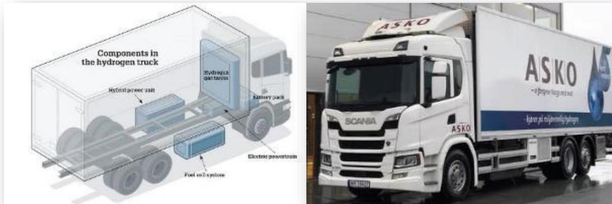
Figure 12: Scania H<sub>2</sub> fuel cell truck.
