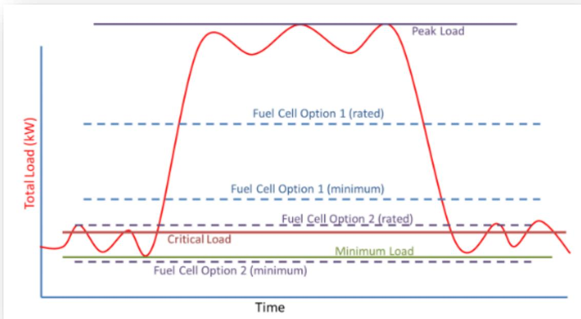
Figure 39: Stylized RMP load during a production shift with impact of embedded generation via a fuel cell.
