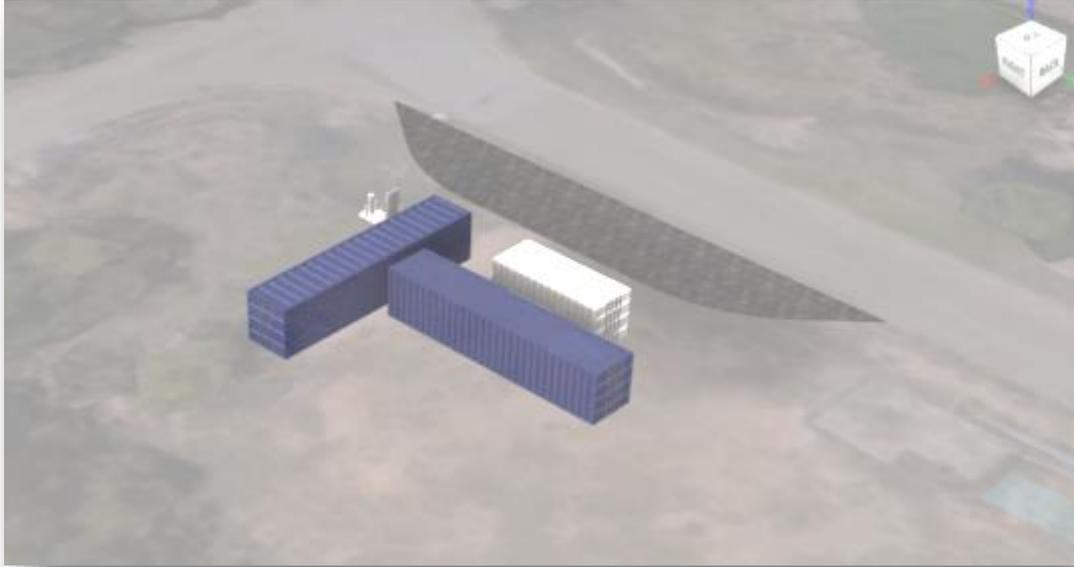
Figure 11: 1 MW electrolyser indicative Option 1 layout orthographic views.
