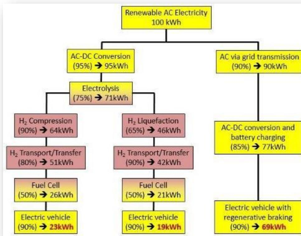
Figure 52: H<sub>2</sub> and electric vehicle production routes, energy efficiency comparison
