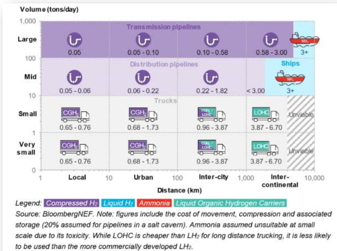
Figure 5: H<sub>2</sub> transportation costs by volume and transport vehicle
