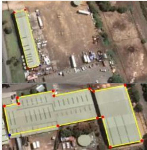
*Figure 47: PV Solar Array Layout Option for supporting a 1MW Hydrogen Electrolyser.*
