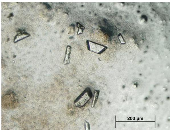
*Photo 2: Individual Struvite Crystals*
