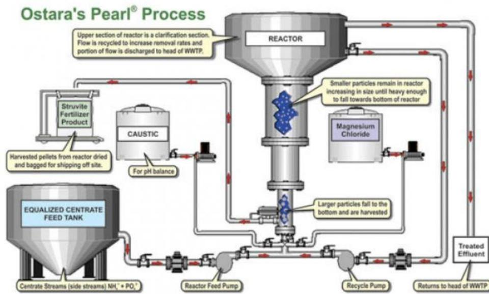
Figure 8: Schematic of Ostara Pearl Process (Hazen and Sawyer)
