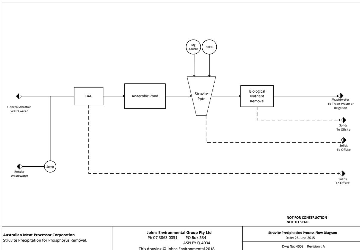
Figure 4: Process Flow Diagram specifying struvite crystallization placement in WWTTP
