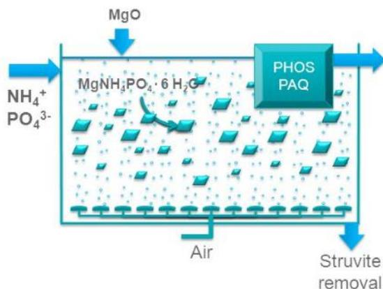
*Figure 9: PhosPAQ Schematic*
