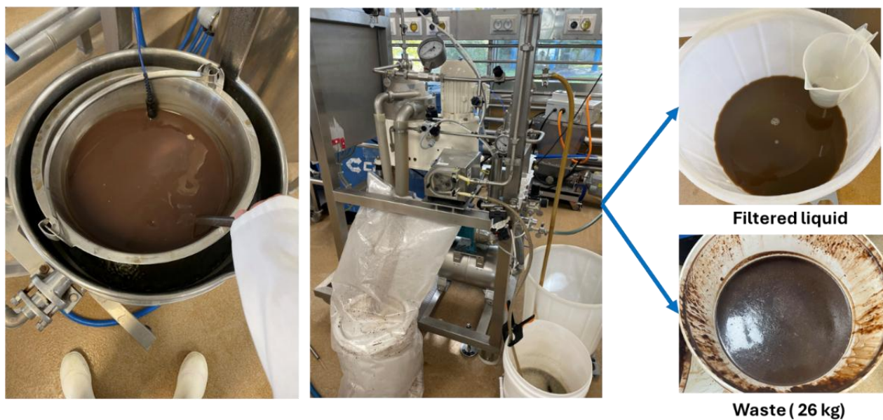
Supplementary Figure 1A-3. Photographs of the clarification step 15 to remove suspended solids from liquid.
