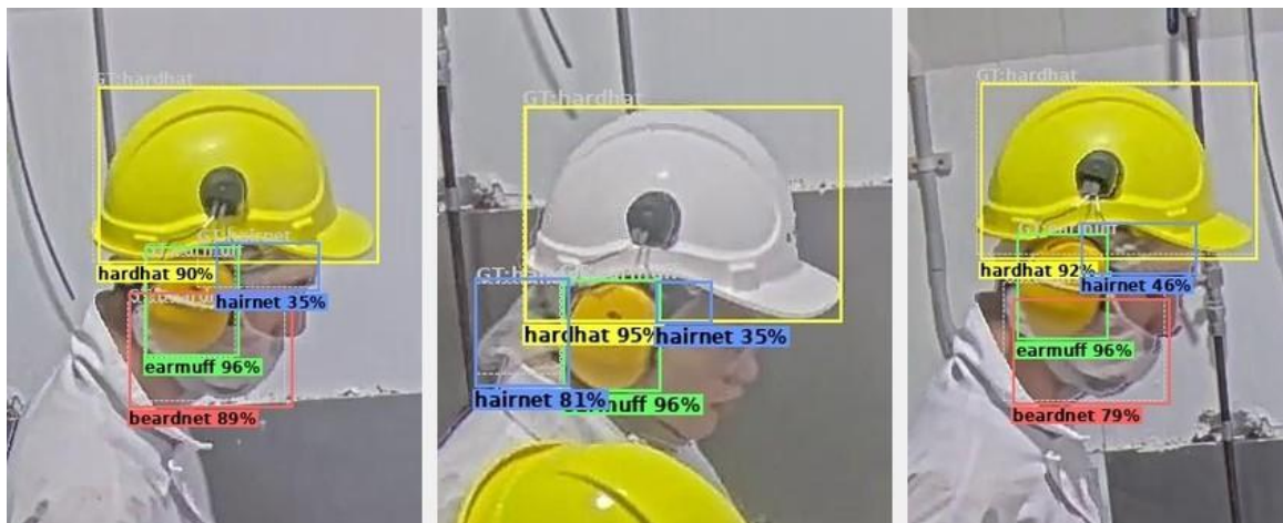
Figure 6.3.1: Example PPE detection results on anonymised head-region crops, showing simultaneous detection of multiple PPE indicators with associated confidence scores.
