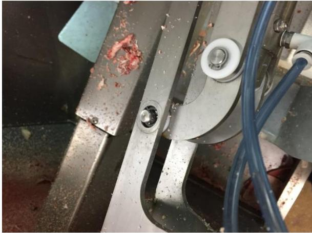
*Figure 9: Dislodged circlip*
