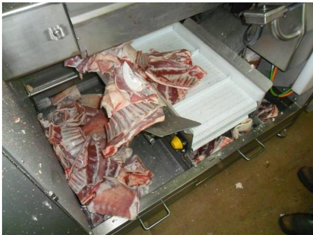
*Figure 11: Accumulation of rack caps and flaps*
