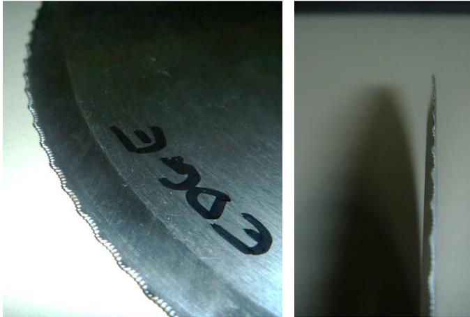
*Figure 5: Cutting blade burring damage*
