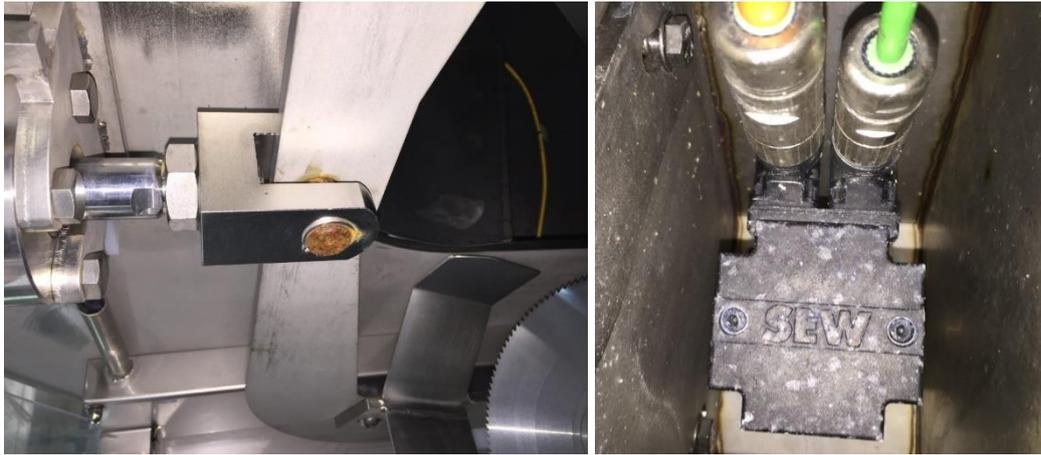
*Figure 12: Corrosion of parts*
