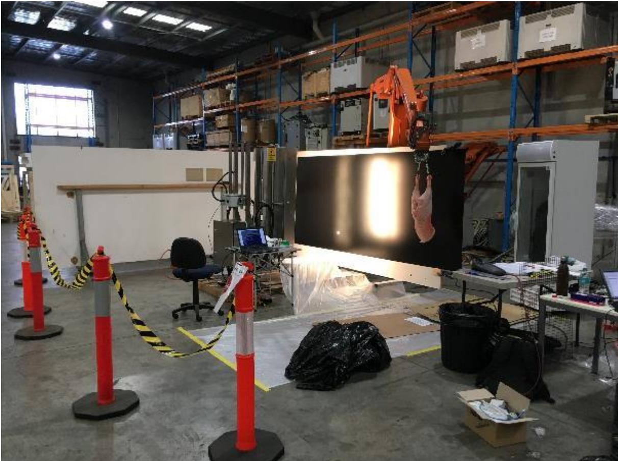
Figure 42: Photo showing a carcass suspended from a pelletizing robot, moving past the hyperspectral rig to simulate the movement of an abattoir overhead conveyor.
