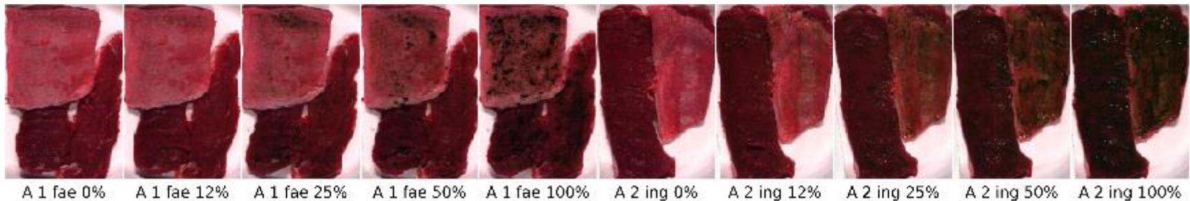
Figure 9: Camera B images of lamb contaminated with varying levels of faeces and ingesta.
