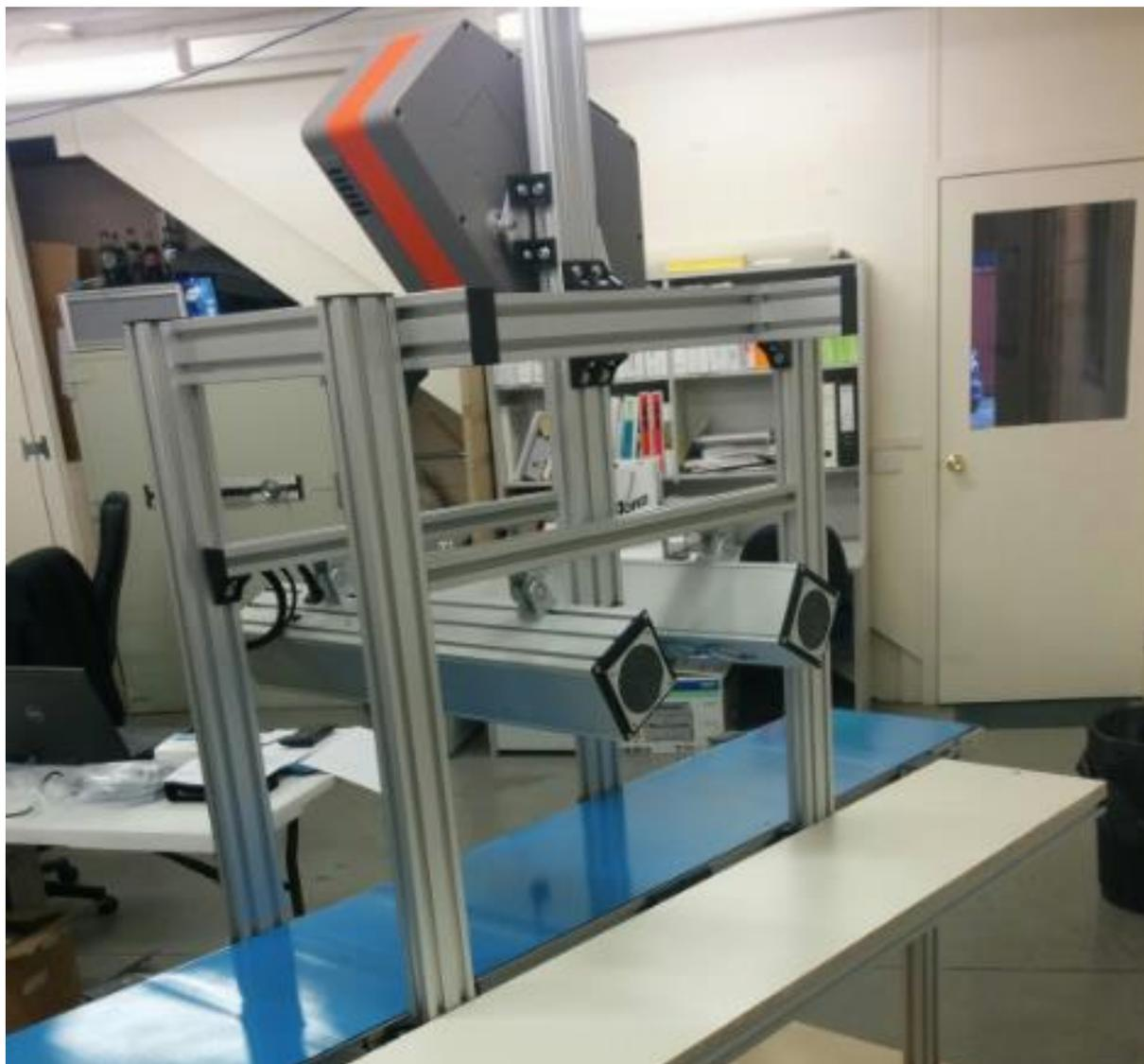
Figure 4: Camera A lighting and conveyor setup.
