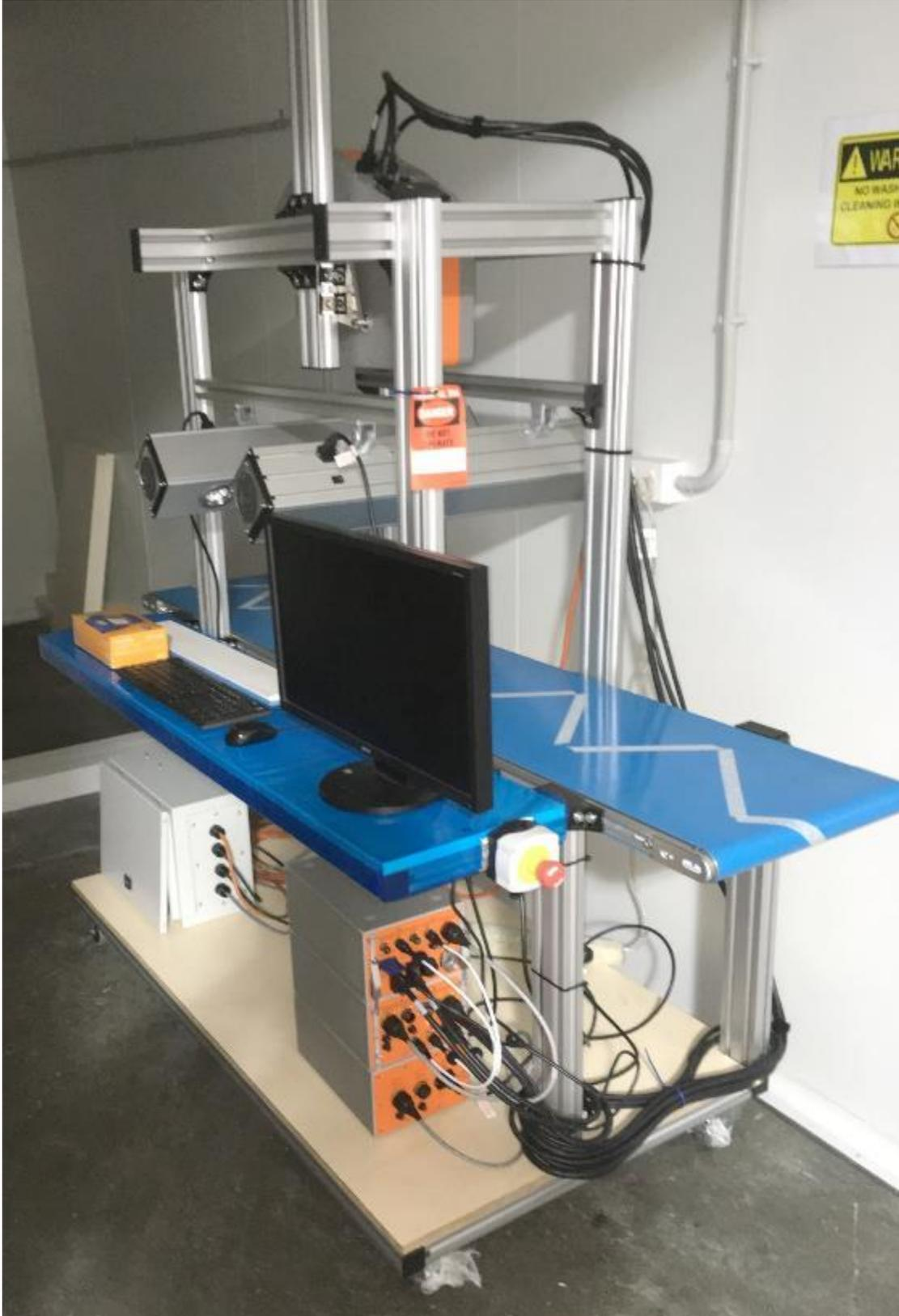
Figure 30: Hyperspectral contaminant detection system in Scott CT room at JBS Brooklyn.
