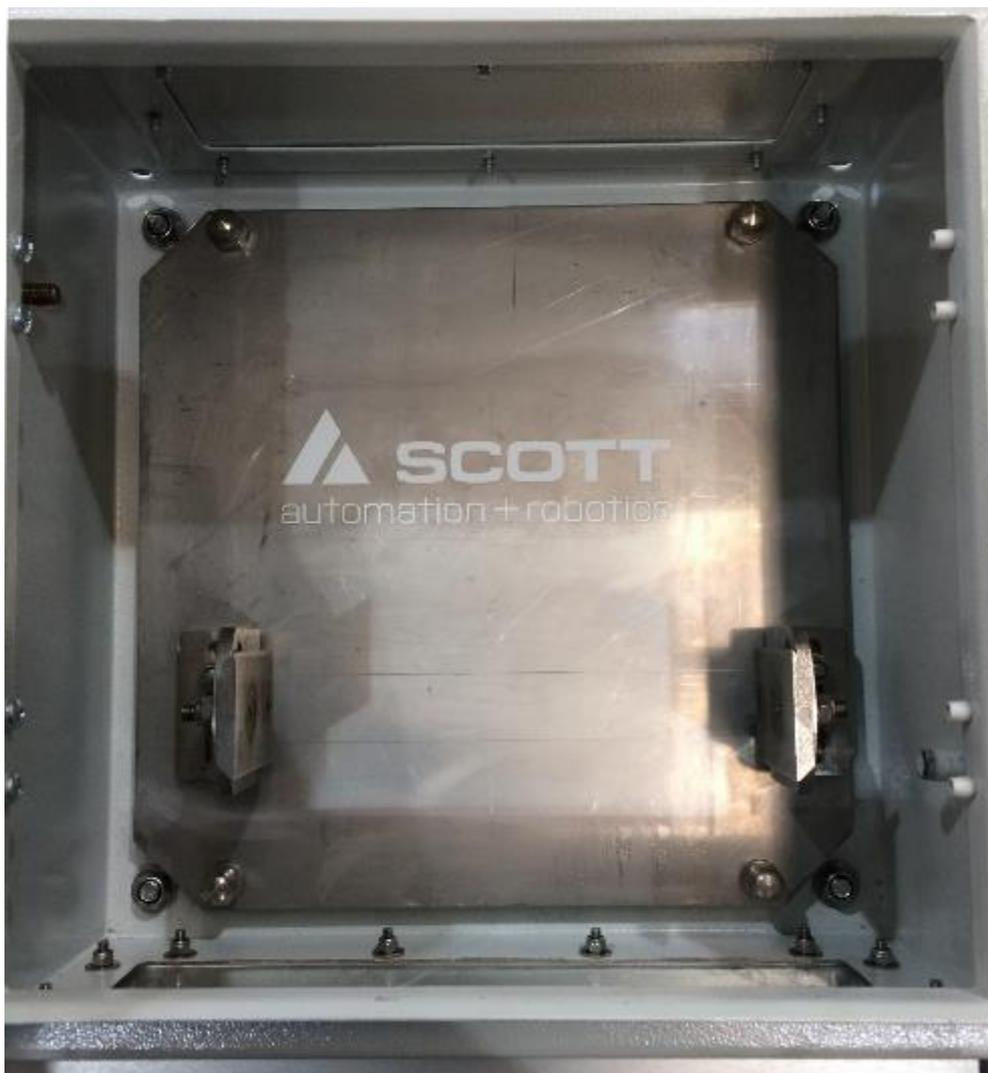
Figure 36: Inside view of camera enclosure showing mounting brackets.
