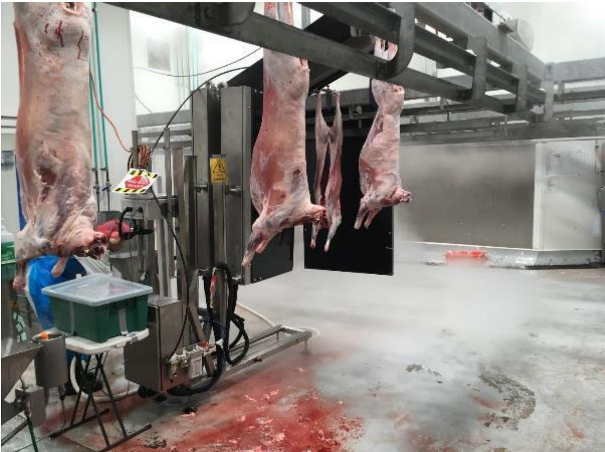
*Figure 58: Contaminant detection system with overhead screen shown above the carcass.*
