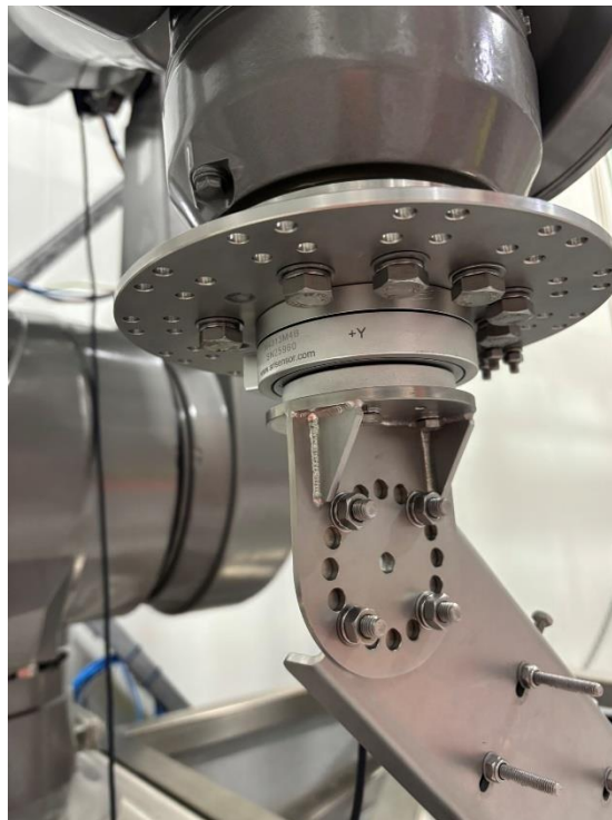
Figure 2 - Force torque sensor mounted to robot (left) and calibrated robot setup (right)
