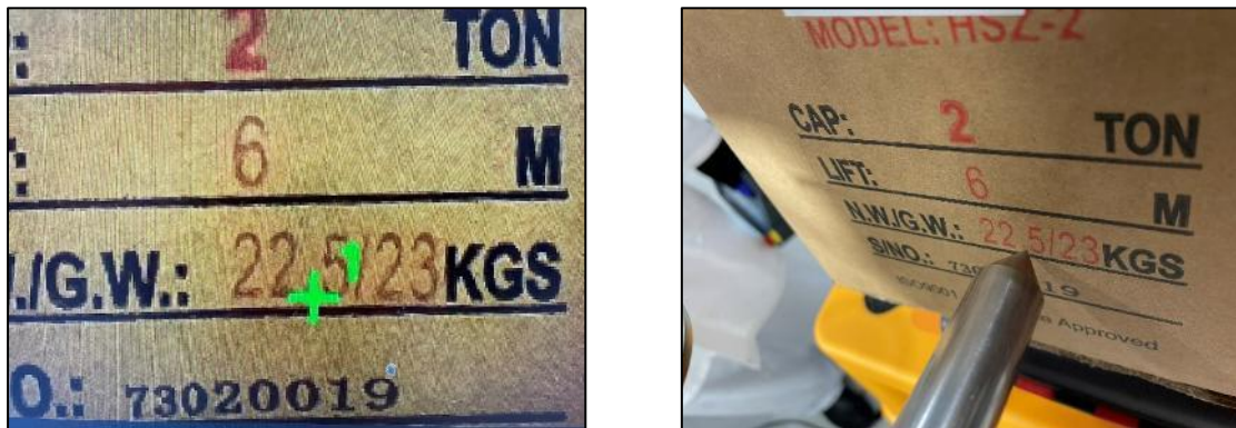
Figure 8- Calibration Touch Test - Clicked Point (left) and Point touched by robot (right)
