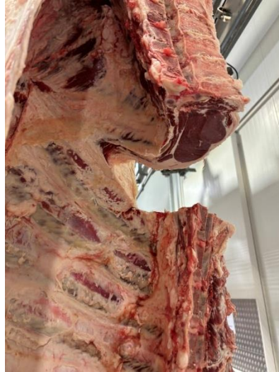
Figure 5 - Trial with hitting rib during grading cut and tilting up rib
