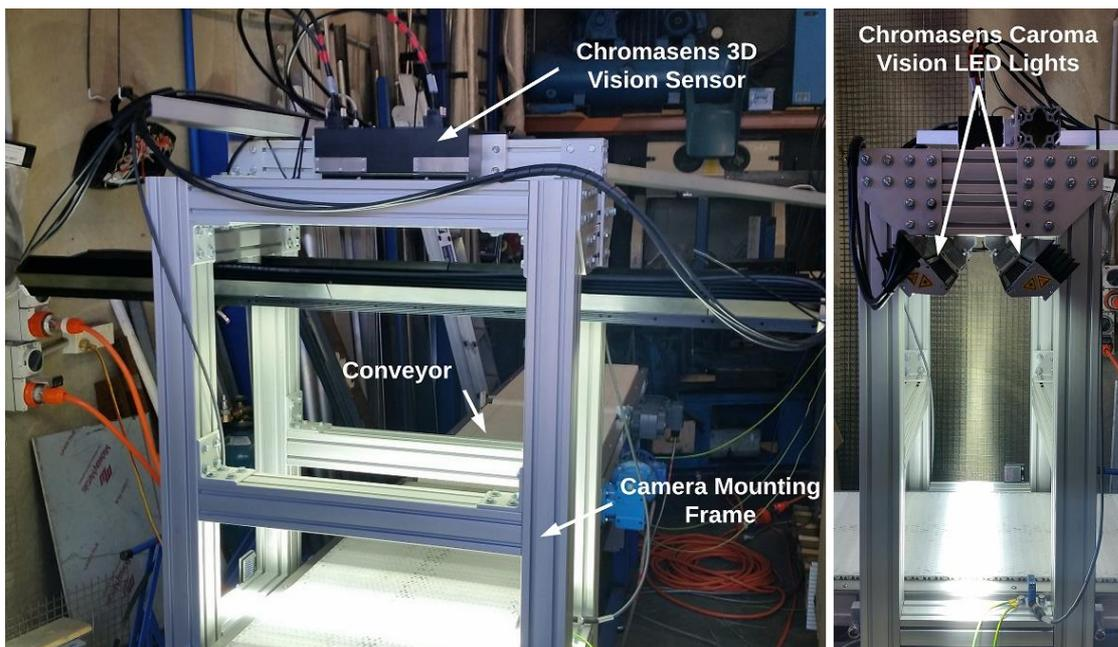
**Figure 8: The completely integrated vision system, consisting of the vision sensor, lights, and mounting frame.**
