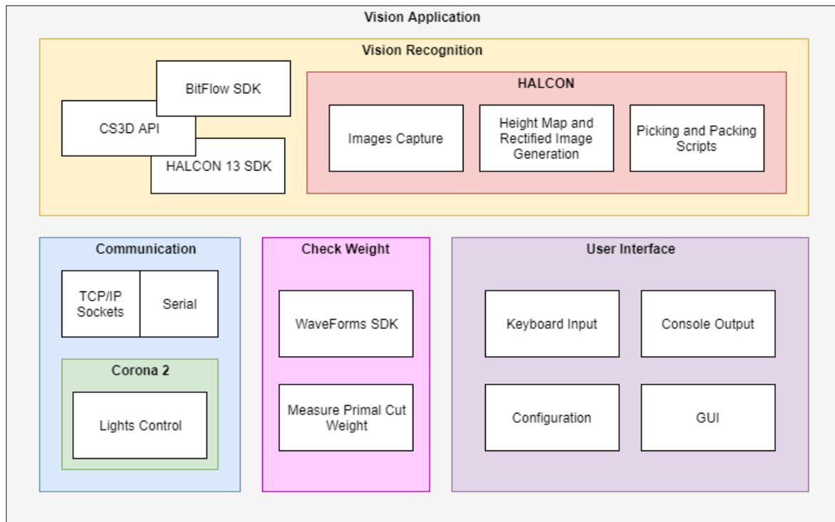
**Figure 20: Vision application architectural diagram**
