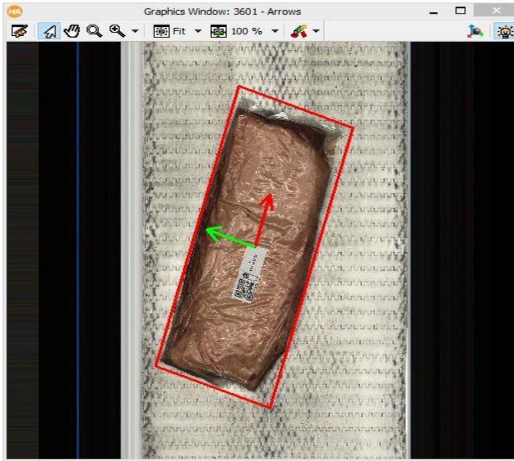
**Figure 17 - Bounding Box and Pick Point**
