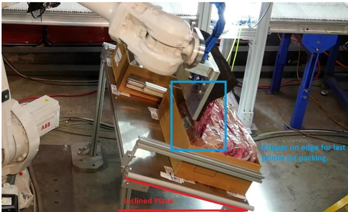
**Figure 27: Side packed (long) inclined plane, gripper on edge of cut for last striploin.**
