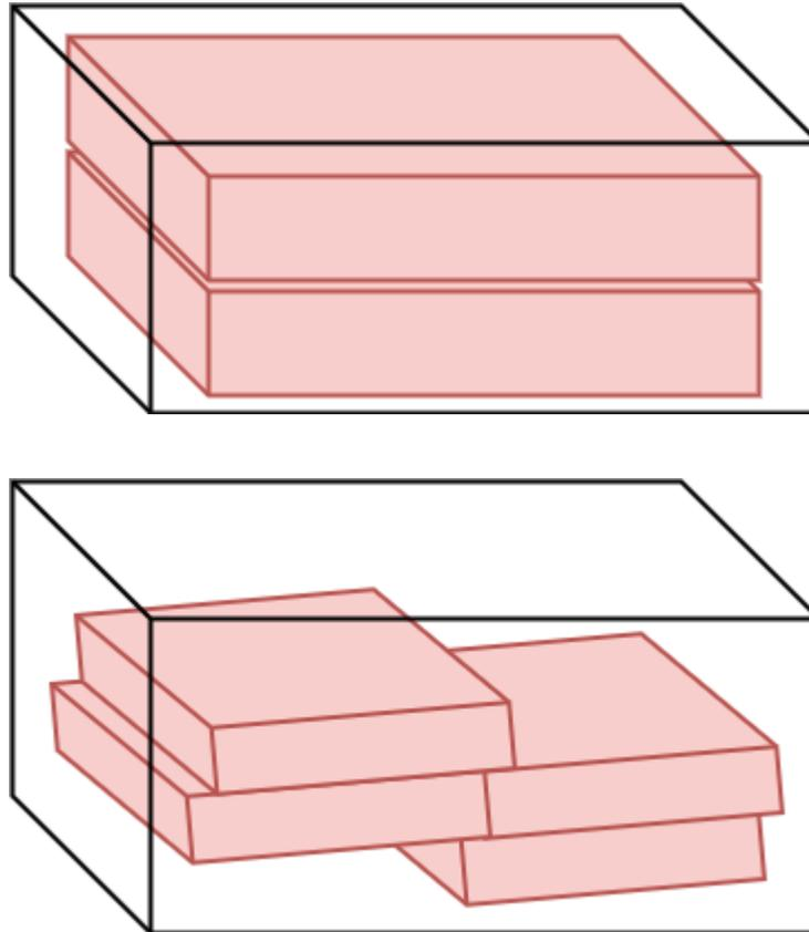
Figure 25: Flat (Top) and shingled (Bottom) packing diagram
