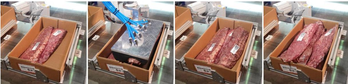
Figure 39: Shingled packing of Tenderloin
