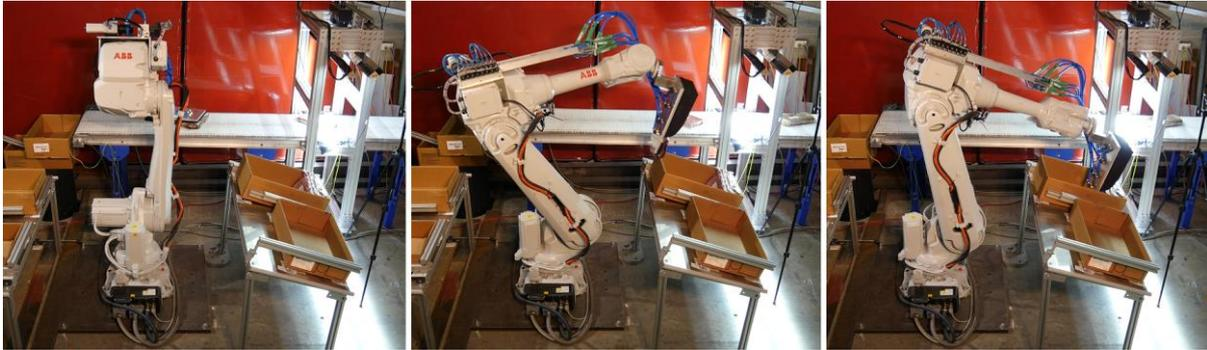
**Figure 40: In-house trial system overview highlighting the pick, intermediary, and pack positions for sideways packing.**
