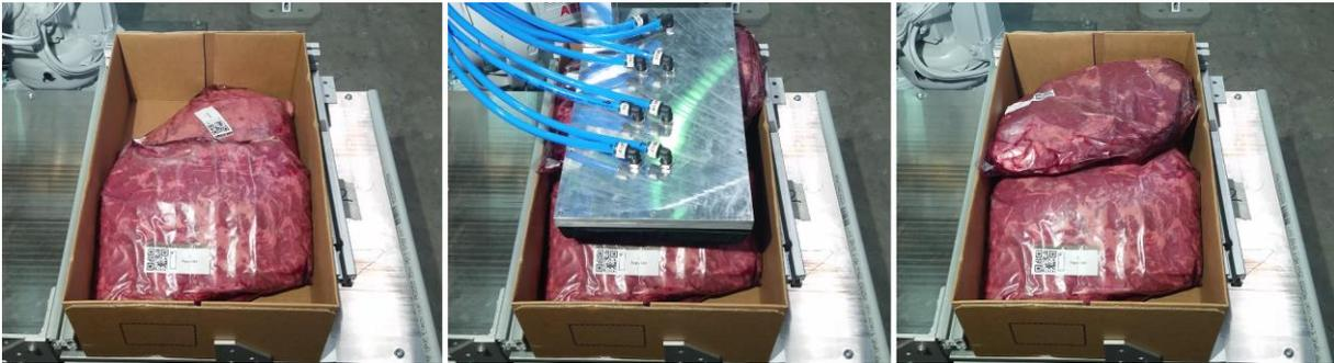
Figure 32: Shingled packing of Topside
