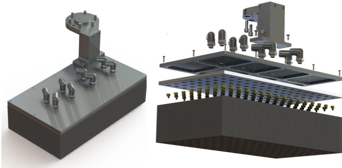
**Figure 4: Rendering of the gripper design; isometric and exploded views.**
