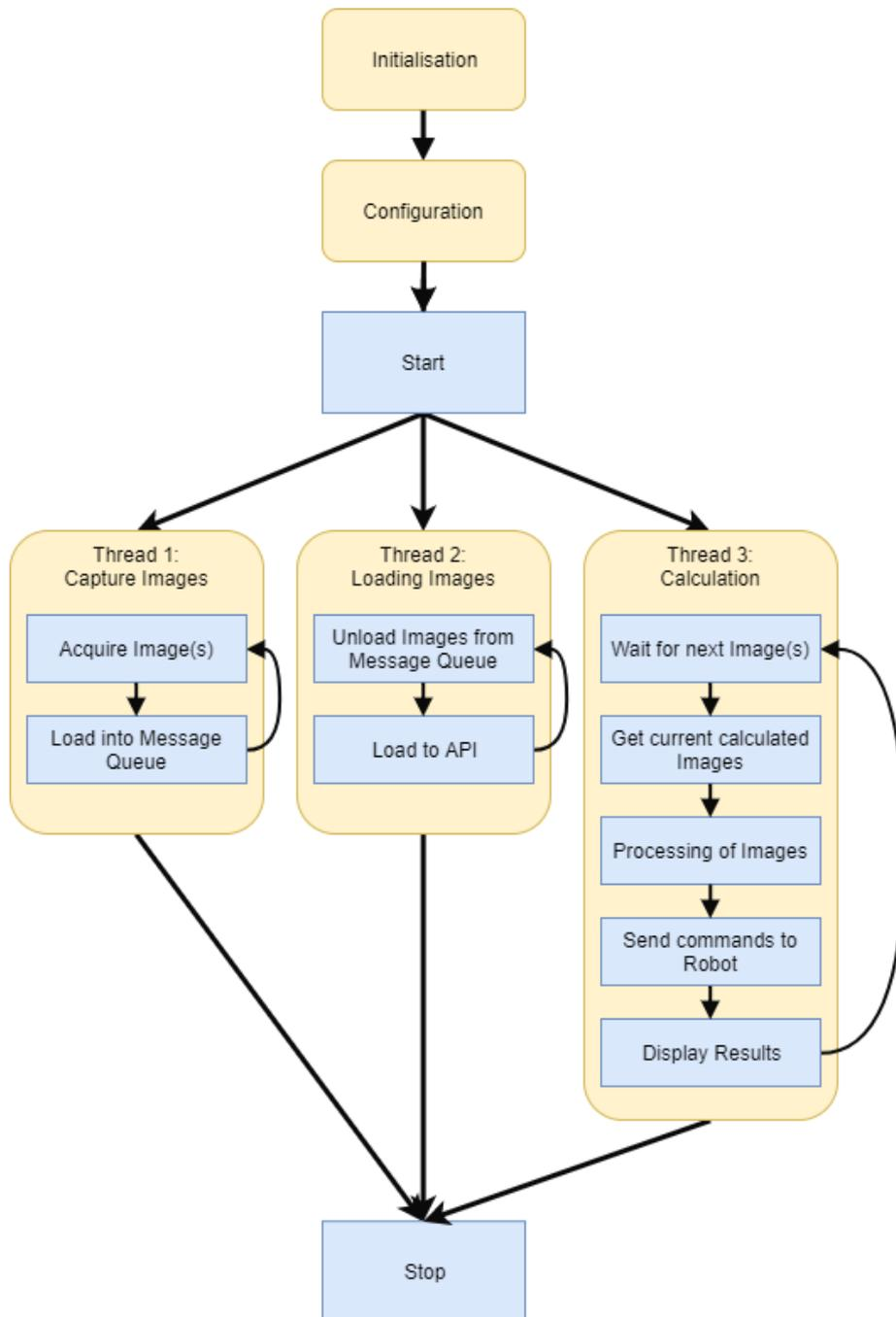
Figure 21: Diagram of application program flow
