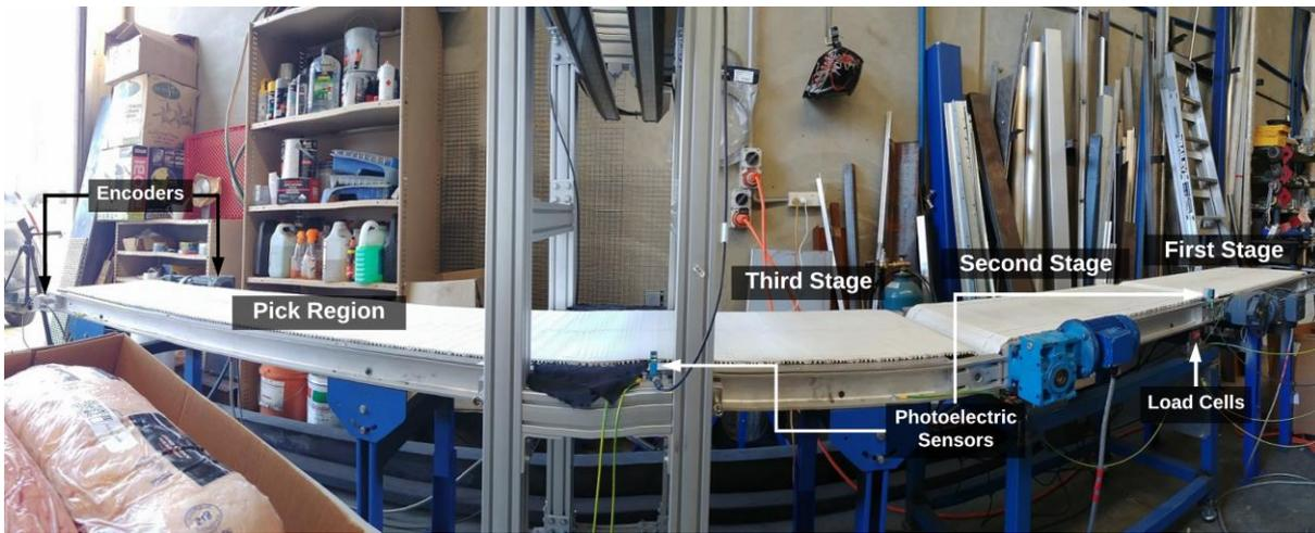
**Figure 9: Annotated view of the developed three stage conveyor system.**
