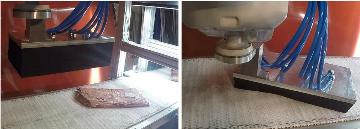
**Figure 22: Rotation when picking primal cut on angle**
