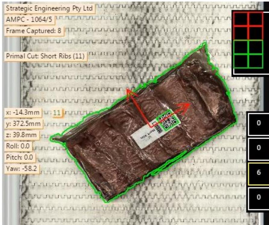
**Figure 23: Snapshot of Vision System output detailing pick coordinates and yaw rotation (left), gripper modules to activate (top right), and destination carton and current number of primal cuts in carton (bottom right).**
