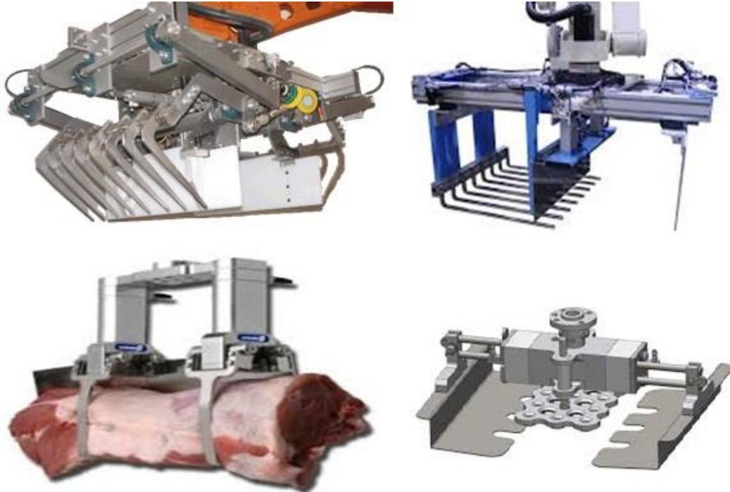
**Figure 2: Various mechanical grippers. Their large size and inherent limited placement dexterity can be seen.**
