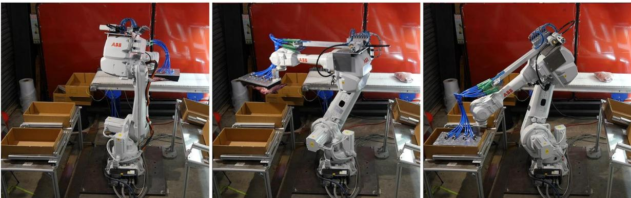
**Figure 31: In-house trial system overview highlighting the pick, intermediary, and pack positions for flat and shingled packing.**
