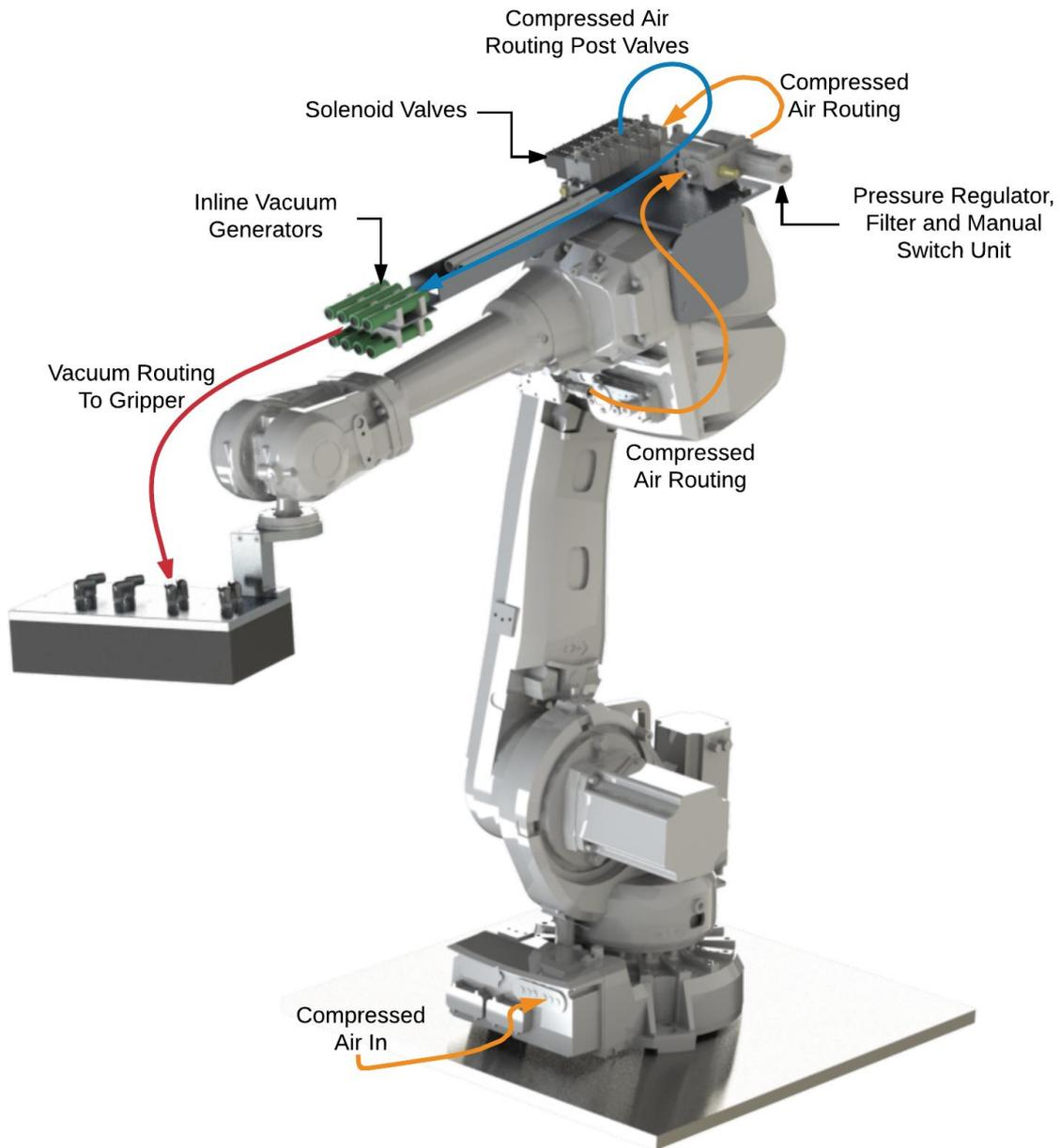
Figure 6: Rendering and diagrammatic overview of robot pneumatic system. The routing tubes, pressure regulator, solenoid valves, and inline vacuum generators are highlighted.
