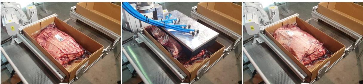
Figure 35: Flat packing of Bolar Blade
