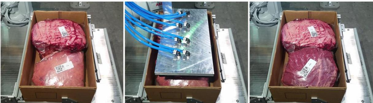
Figure 37: Shingled packing of Rump
