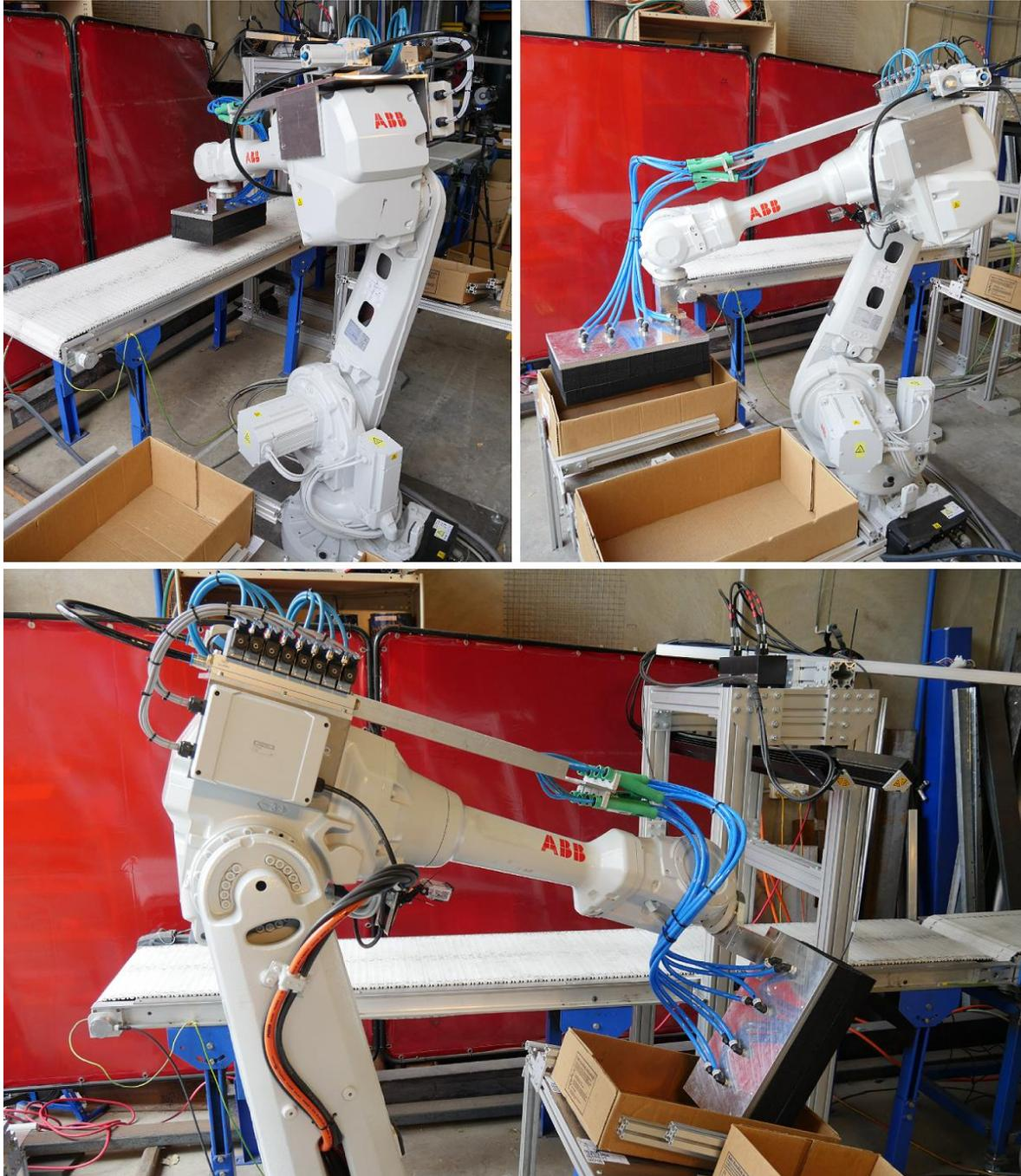
Figure 7: Fully integration pneumatic vacuum gripper system with the ABB IRB 4600 six-axis robot. Pick off and pack positions are shown.
