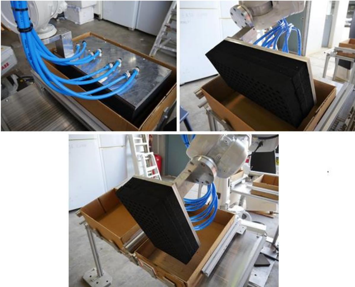
**Figure 30: Flat packing arrangement (Top Left) side-long packing (Top Right) side-short packing (Bottom) robot gripper orientations without primal cuts.**
