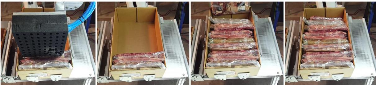
**Figure 42: Side-short packing of Short Ribs**
