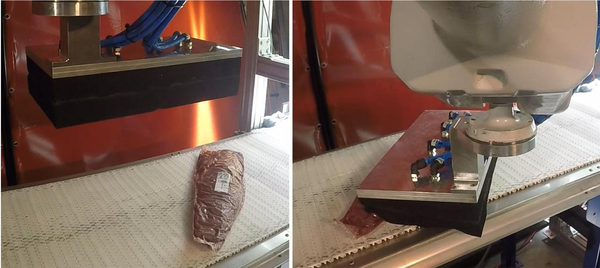
Figure 24: Tenderloin head first and offset on pick up
