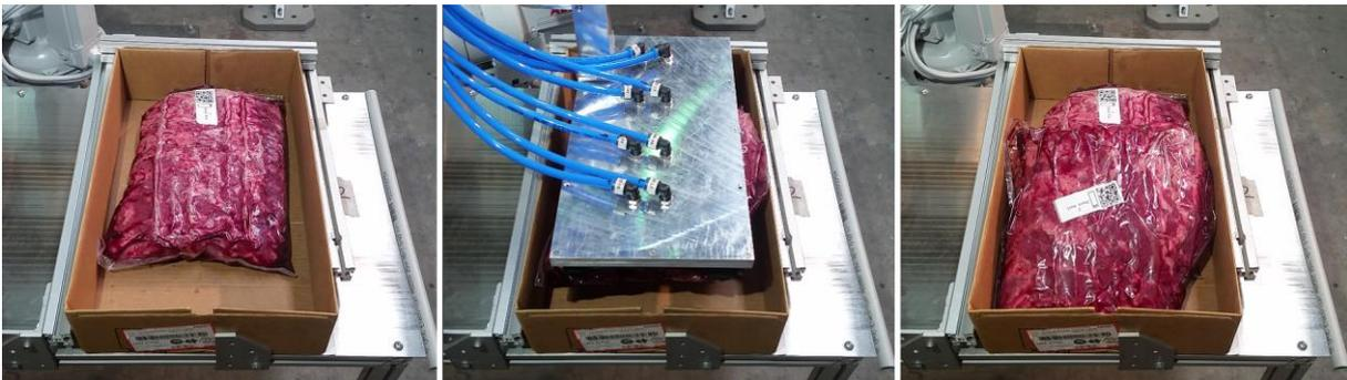
Figure 33: Shingled packing of Chuck Roll
