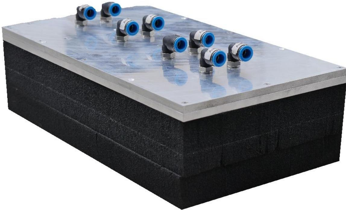
Figure 5: Fully assembled vacuum pad gripper with 120mm thick foam.
