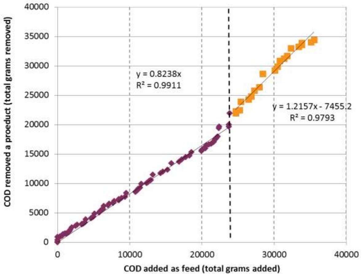
Figure 17: COD balance in the AnMBR pilot plant operated at 37°C. The slope of the linear regressions indicates the fraction of Feed COD that leaves the AnMBR as product (biogas and permeate).
