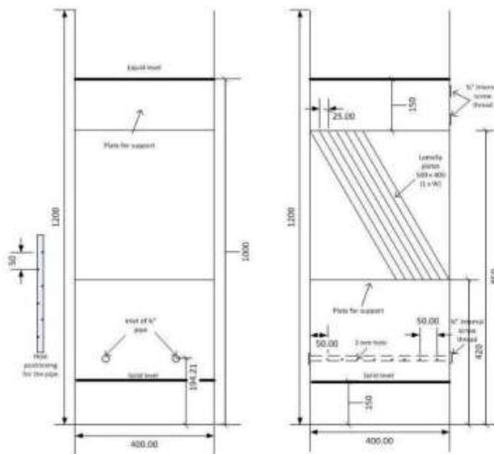
**Figure 3: Design of struvite crystallizer used to extract phosphorus and nitrogen from processing plant wastewater**
