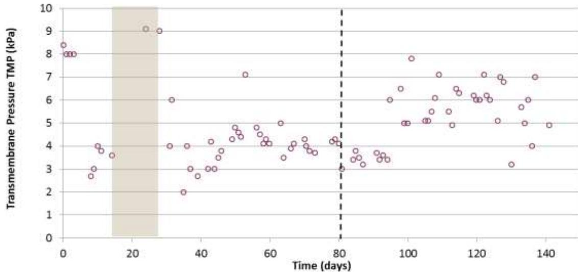
Figure 11: Transmembrane pressure in AnMBR pilot plant is stable indicates sustainable fouling.
