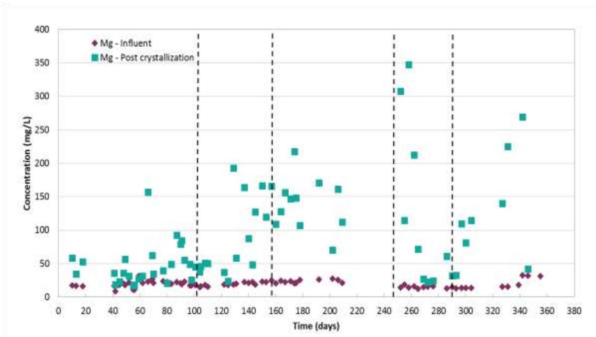
Figure 15: Magnesium concentrations in struvite crystallisation plant installed at an Australian meat processor treating anaerobic lagoon effluent.
