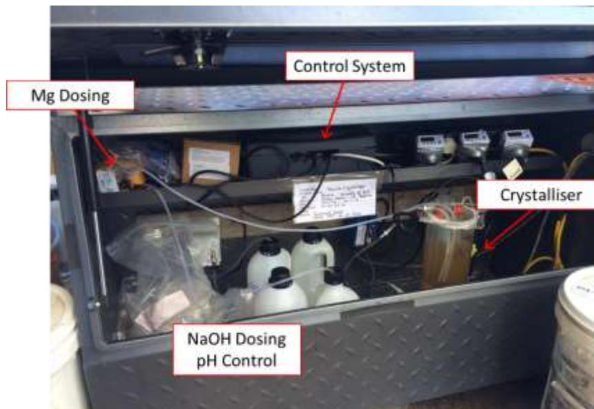
**Figure 4: Design of struvite crystallizer used to extract phosphorus and nitrogen from AnMBR treated effluent**
