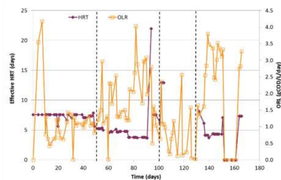
**Figure 6: Effective hydraulic retention time (HRT) and Organic Loading Rate (OLR) during the pilot plant operation at 37°C**
