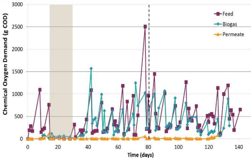
**Figure 10: COD loading to the AnMBR pilot plant during operation at 55°C with corresponding COD removal as permeate and biogas**
