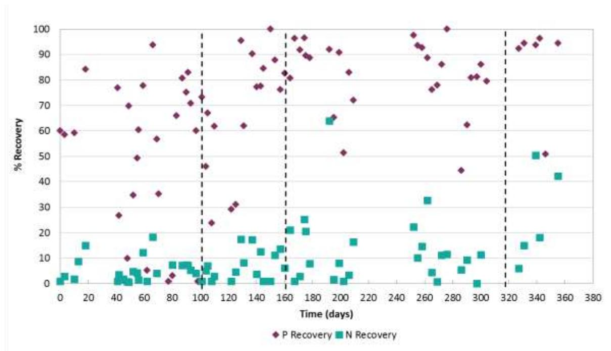
Figure 16: Summary of Phosphorus recovery and Nitrogen Recovery from the struvite crystallisation plant installed at an Australian meat processor treating anaerobic lagoon effluent.
