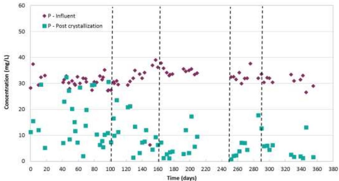
**Figure 13: Phosphorus removal in struvite crystallisation plant installed at an Australian meat processor treating anaerobic lagoon effluent.**
