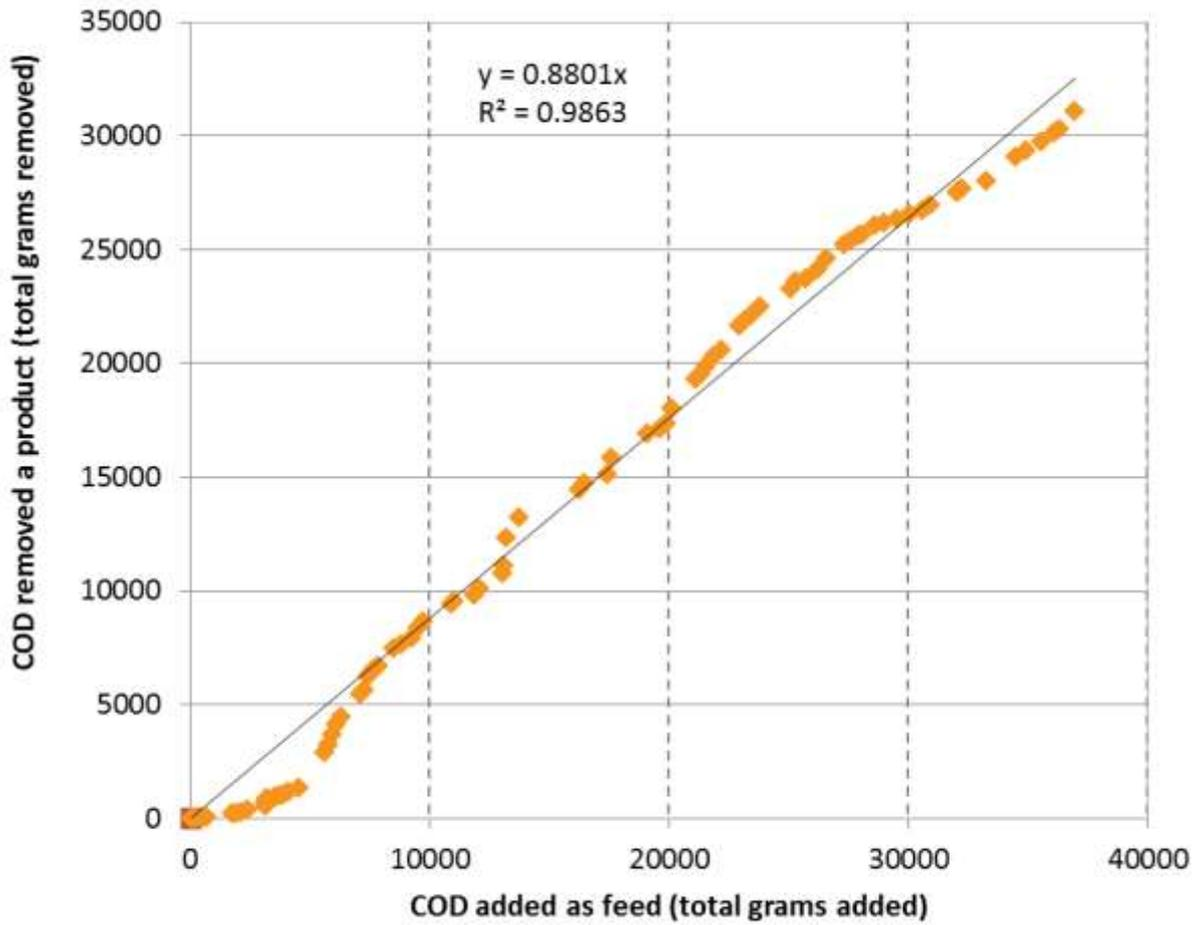
Figure 18: COD balance in the AnMBR pilot plant operated at 55°C. The slope of the linear regressions indicates the fraction of Feed COD that leaves the AnMBR as product (biogas and permeate).
