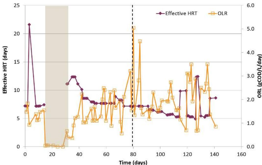
**Figure 9: Effective hydraulic retention time (HRT) and Organic Loading Rate (OLR) during the pilot plant operation at 55°C. Shaded area represents process shut-down due to overload inhibition**
