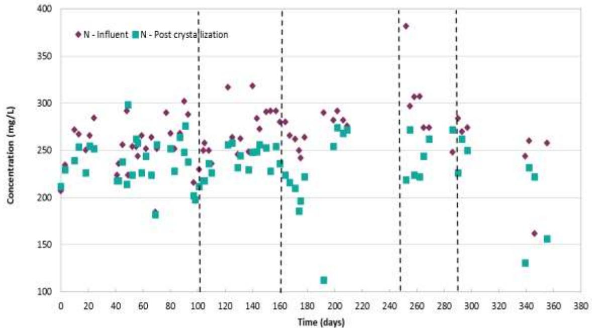
**Figure 14: Nitrogen removal in struvite crystallisation plant installed at an Australian meat processor treating anaerobic lagoon effluent.**
