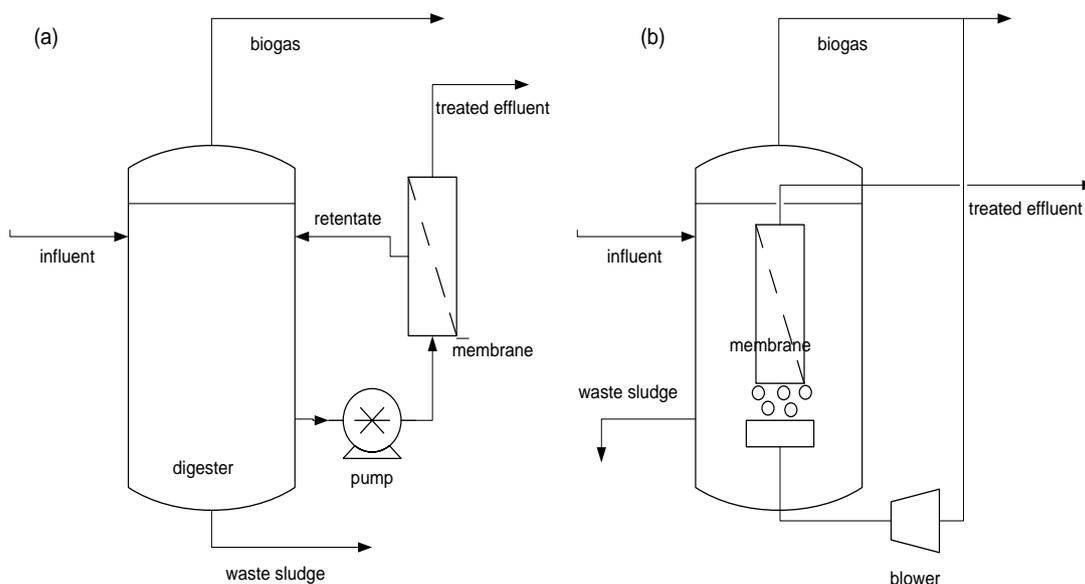
**Figure 1: MBR configurations, including (a) Sidestream membrane bioreactor (sMBR) and (b) Immersed membrane bioreactor (iMBR).**
