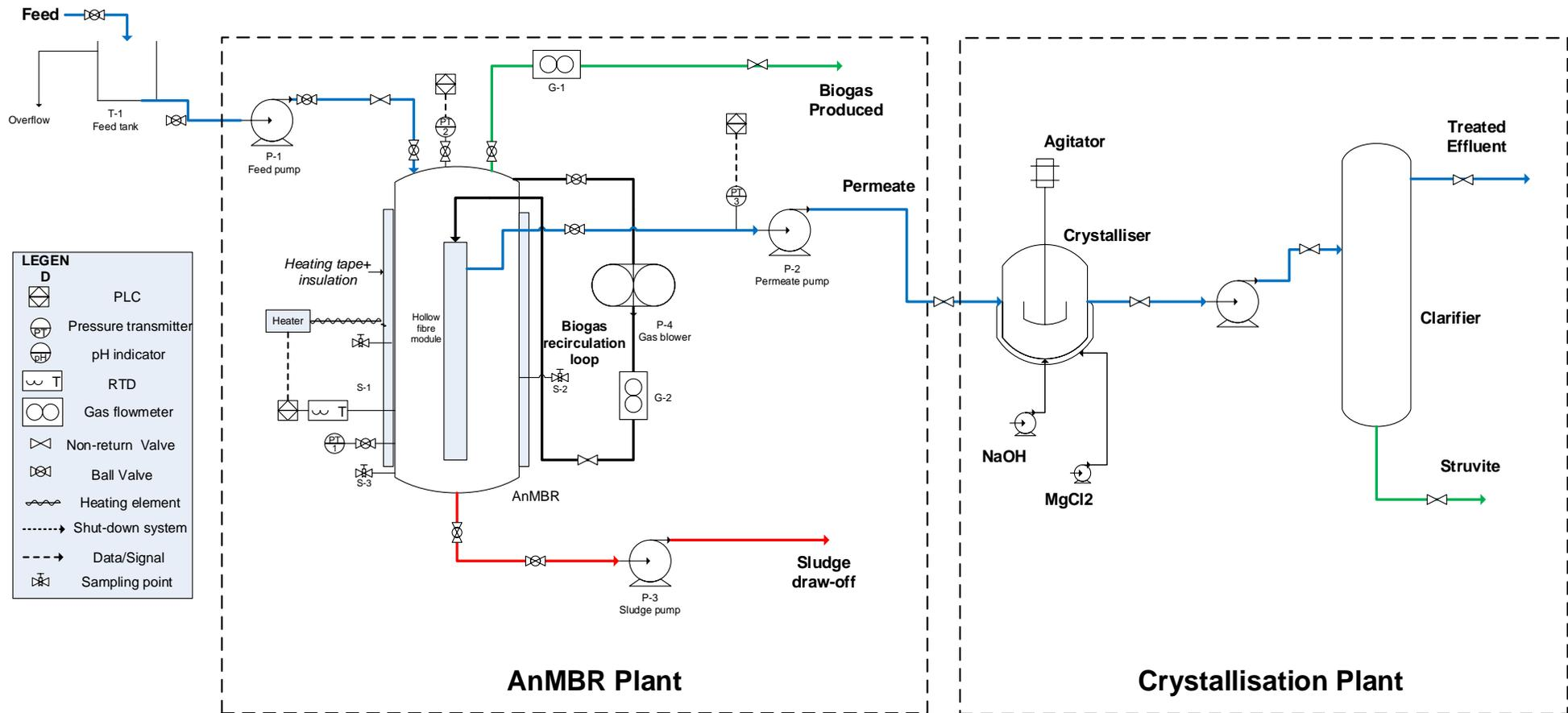
Figure 5: Detailed piping and instrument diagram of the integrated treatment process consisting of anaerobic membrane pilot plant and struvite pilot plant.
