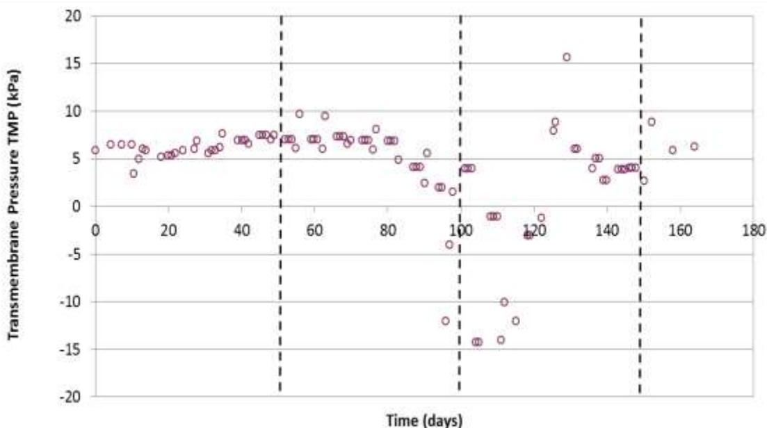
**Figure 8: Transmembrane pressure in AnMBR pilot plant is stable indicates sustainable fouling.**
