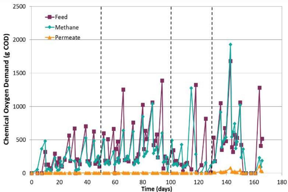
**Figure 7: COD loading to the AnMBR pilot plant during operation at 37°C with corresponding COD removal as permeate and biogas**
