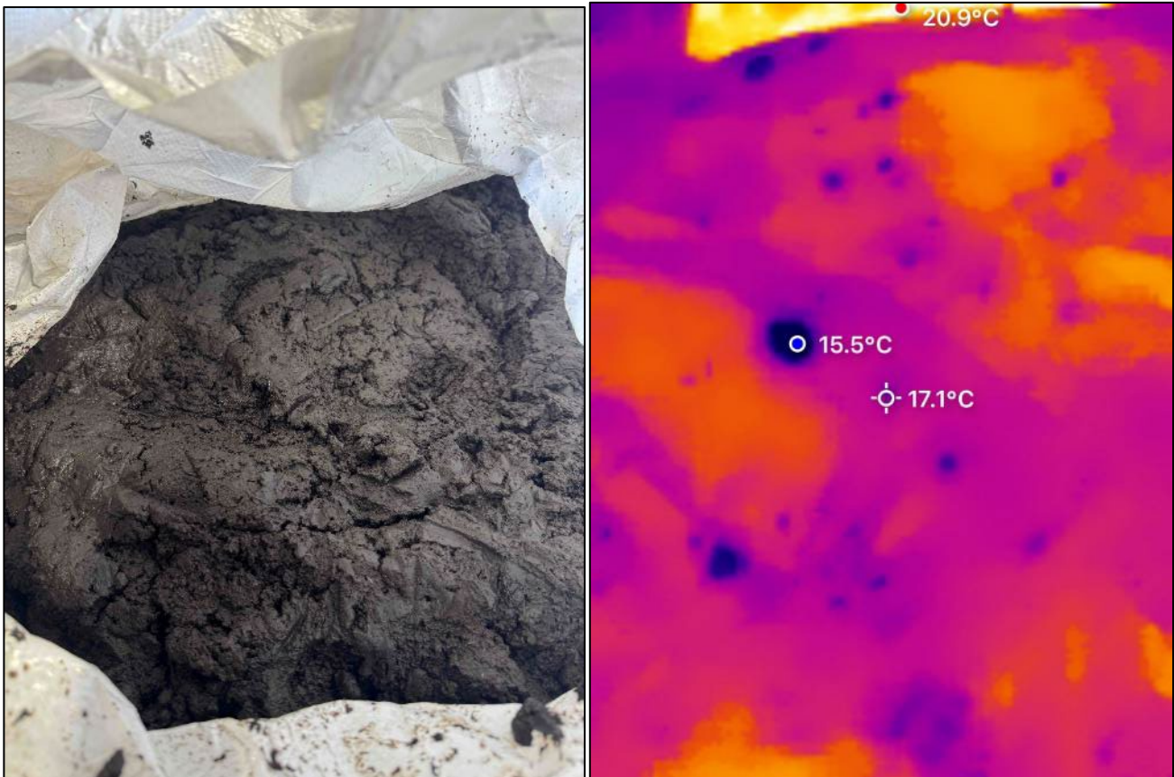
Figure 15: Sludge feedstock sample, 17 th June 2026. The thermal image shows that the sludge temperature is close to that of the wet bulb temperature.
