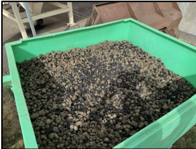
Figure 8: Pellet / coal mix prepared on 18 June 2026 ready for the burn test on 24 th June 2026.
