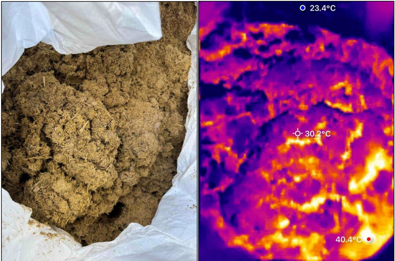
Figure 16: Paunch feedstock sample 17 th June 2026. The thermal image shows that the temperature has reached 40.4 DegC. The paunch would have high microbial activity as evidenced by the temperatures shown in the thermal image.
