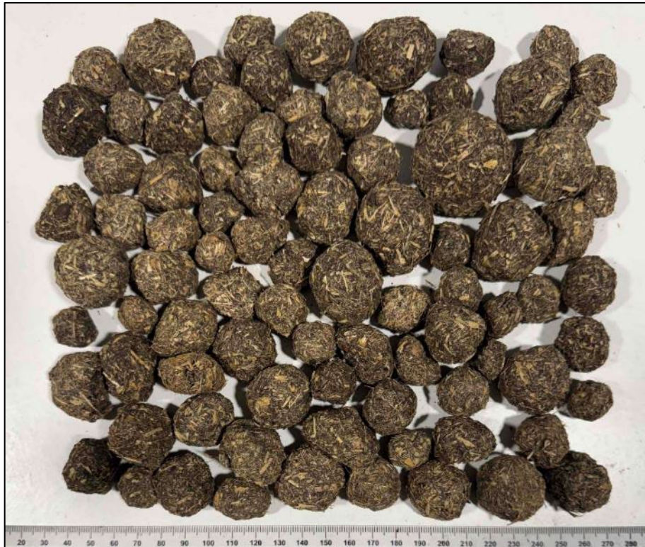
Figure 17: PAUNCH/SLUDGE PELLETS used in the burn test showing particle diameters of 9 to 40 mm, with the median range being 20 to 30 mm. Fines were less than 0.4% by mass.
