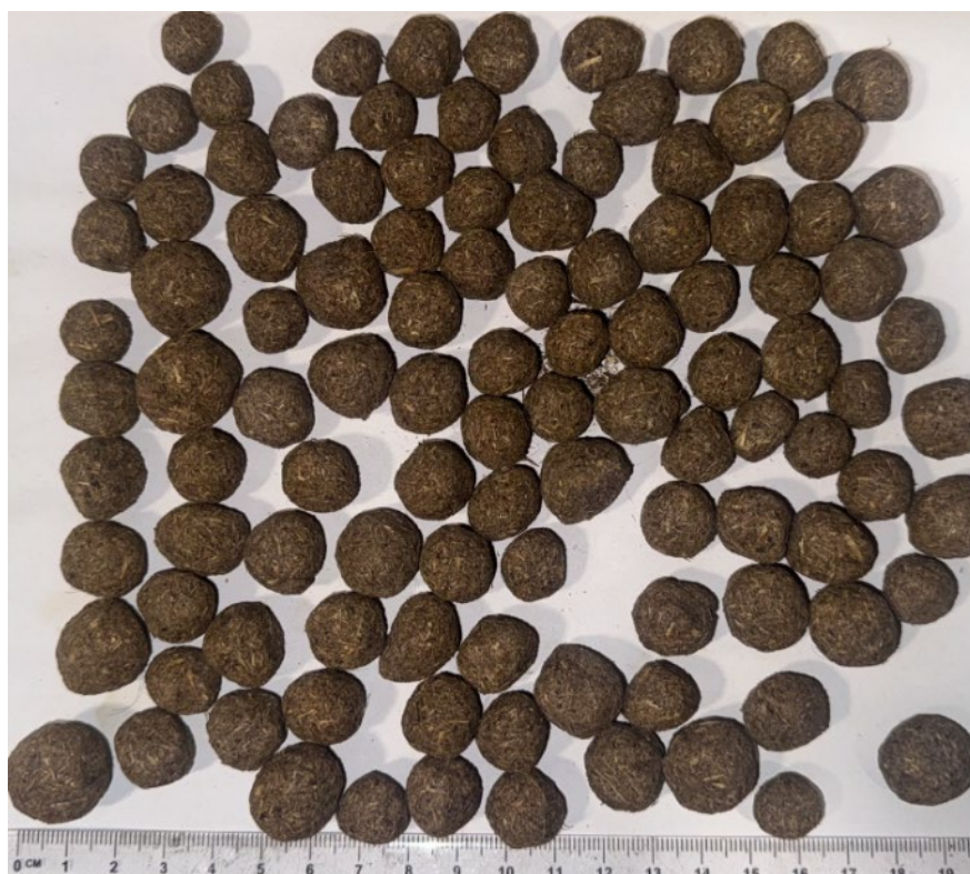
Figure 18: PAUNCH/SLUDGE/20% SAWDUST PELLETS developed after findings from the burn test showing particle diameters of 11 to 23 mm.
