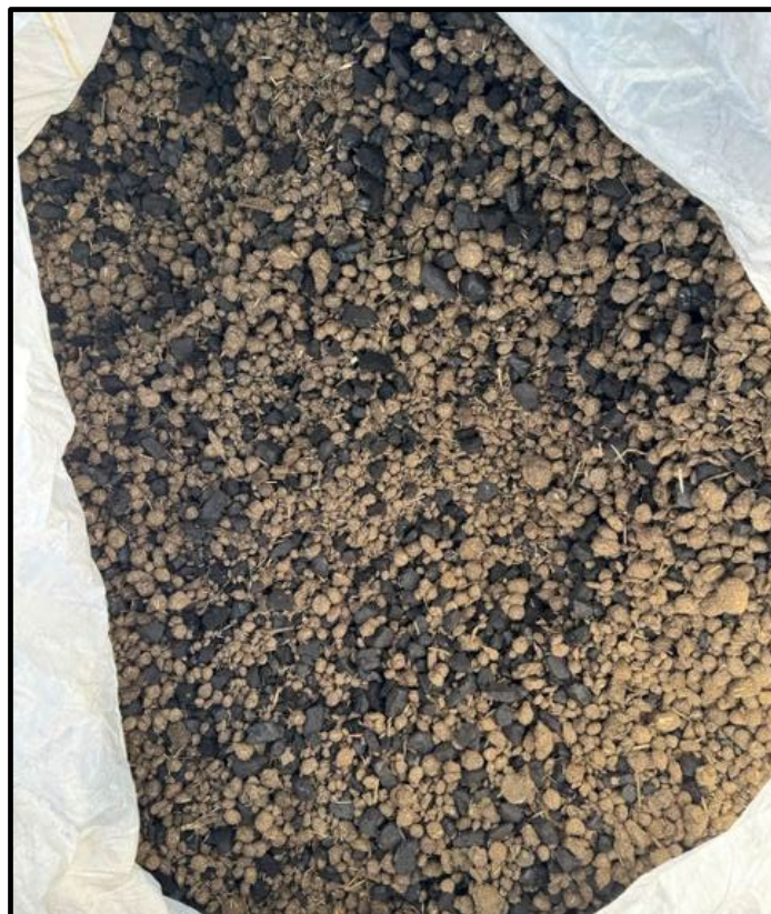
Figure 9: an additional 0.28 tonnes of pellet / coal mix (1 hour of fuel) was prepared on 23 June 2026 as reserve fuel ready for the burn test on 24 th June 2026.
