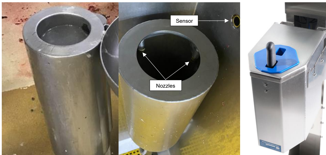
Figure 29: Steriliser types: [Left] Continuous flow dunk steriliser; [Middle] Reduced flow sensor activated nozzle spray steriliser; [Right] High efficiency Econoliser.
