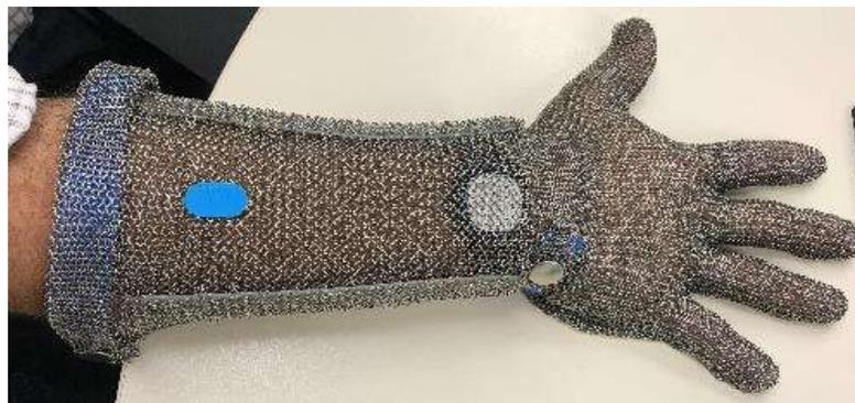
Figure 1: IIoT Meta sensor (Watch Device) worn under protective mesh glove.
