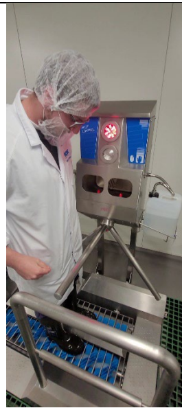
Staff using the bottom tread scrubber and sanitizer application
