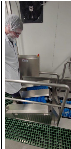
Staff using the side boot scrubber and sanitizer application
