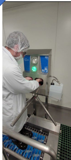
Application of sanitizer to both hands (note: green light now allows the employee access through turnstile to Retail ready room)
