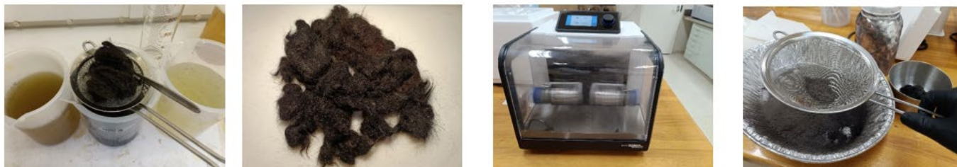
Figure 1. Sample preparation steps for native bovine hair and Sirolime hair waste prior to keratin extraction. From left to right: washing and decontamination, cleaned and dried hair fibres, ball milling, and sieving of milled hair powder.
