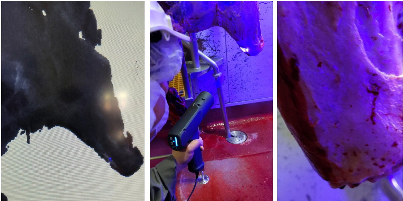
Figure 24: BluMax detection as invisible [left] and BluLine validation [middle]. Visual check [right] was inconclusive.
