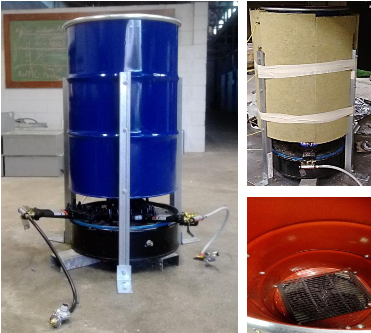
Figure 15: Steel drum (left), insulation (top right) and internal structure (bottom right)
