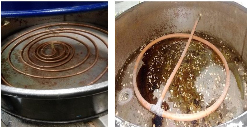
Figure 17: The two air diffuser configurations tested: (left) spiral copper pipe and (right) hose ring
