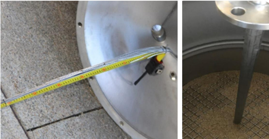
Figure 25: Thermocouples through the lid of the drum (left) and thermowell (right) used to place the thermocouples vertically, inside, and in the centre of the reactor.
