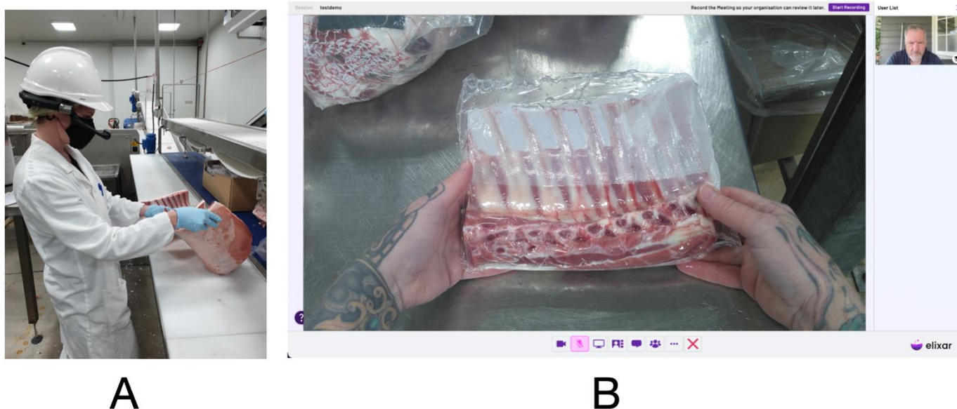
Fig5. (A) Onsite QA officer wearing Realwear smart glasses inspecting a cut of meat while connected to, and receiving instruction from, a remote food safety auditor in an Elixar session (B). Remote auditor gets an I-see-what-you-see image from the QA smart glasses
