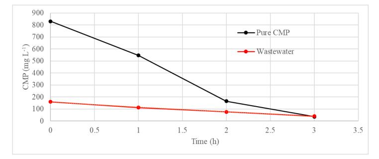
Figure 2. Concentration of the pure test POC 4-chloro-3-methylphenol (CMP) and CMP in tannery wastewater over time at an O<sub>3</sub> dose rate of 0.5 g h<sup>-</sup>.
