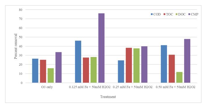
Figure 8. Removal of COD, TOC (total organic carbon), DOC (dissolved organic carbon), and the test POC 4-chloro-3-methylphenol (CMP) in the venturi delivery trials.
