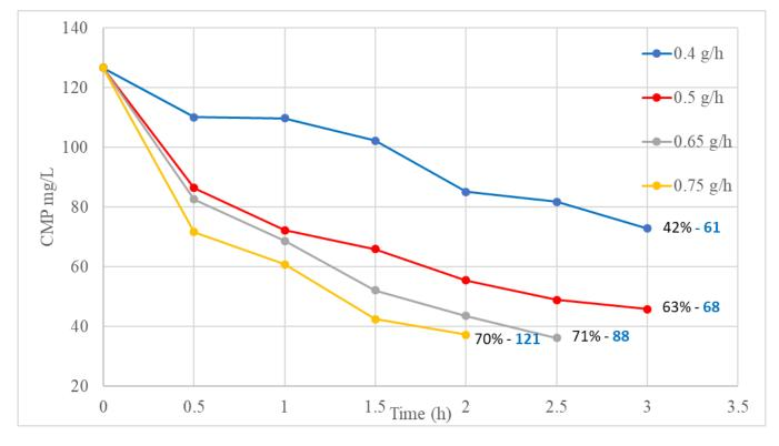
Figure 6. Degradation of the test POC 4-chloro-3-methylphenol (CMP) in 4 L tannery wastewater at different  $O_3$  dosing rates of 0.4, 0.5, 0.65, and 0.75 g h<sup>-1</sup> over 3 h. Percent reduction is also shown in units of mg POC g<sup>-</sup>  $O_3$  h<sup>-1</sup> (bold blue numbers).
