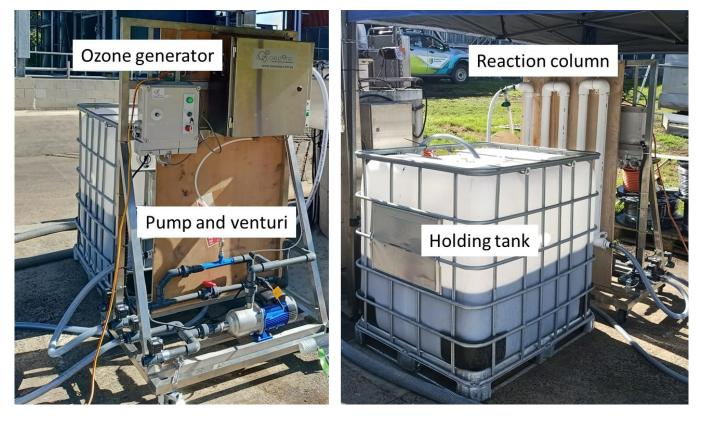
Figure 4. Pilot venturi reactor system set up at Casino Hide Tanners.
