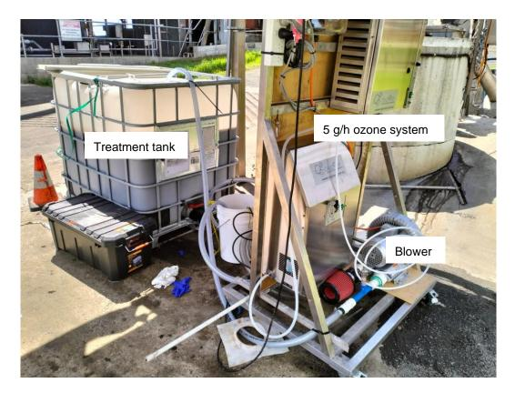
Figure 5. Pilot blower reactor system set up at Casino Hide Tanners.
