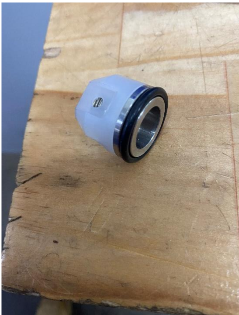
Image 1: Udor Teflon Cage Valve Replacement
