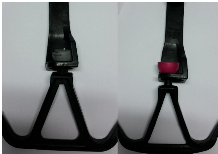
Figure 1: Carcase gambles used for system, (left) Wedge transponder, (Right) Glass transponder.
