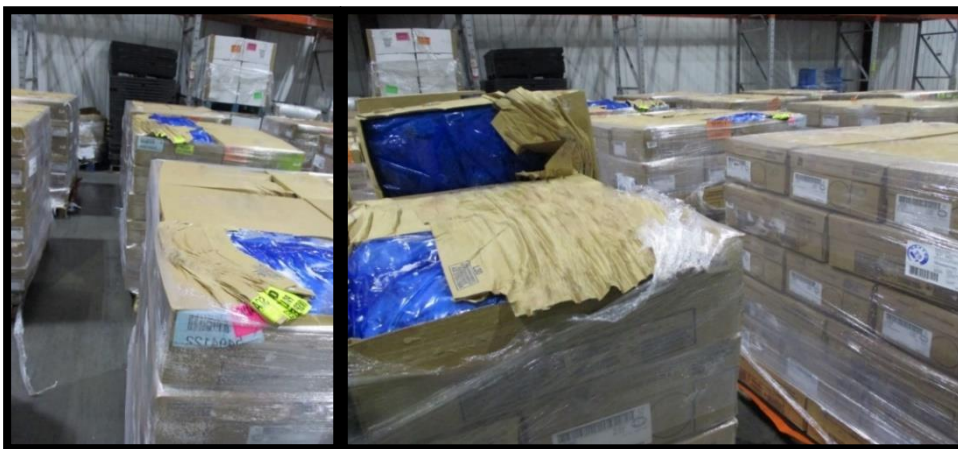
Figure 18 - Cartons damaged by forklift picking up pallet stacked on top of them.
