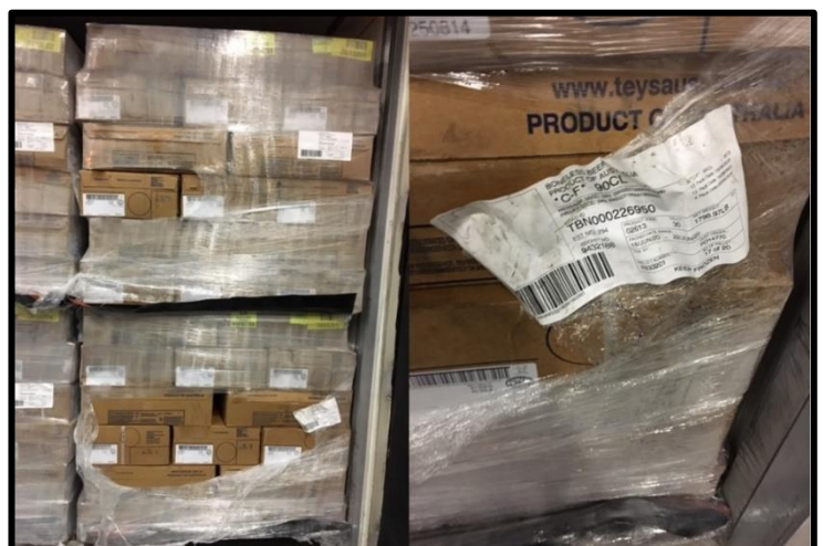
Figure 19 Images of pallet wrap being torn off, damaging SSCC placards.
