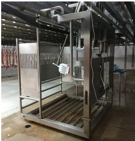
Figure 1 – Production Prototype installed in the chiller. The pusher arm is in the centre of the photo. The Marbl™ sensor is partially obscured.
