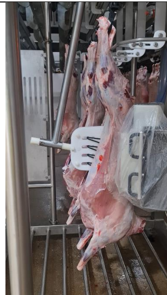
Figure 2 – View of measurement being made, with a lamb carcass being pressed up against the Marbl™ sensor by the pusher arm.
