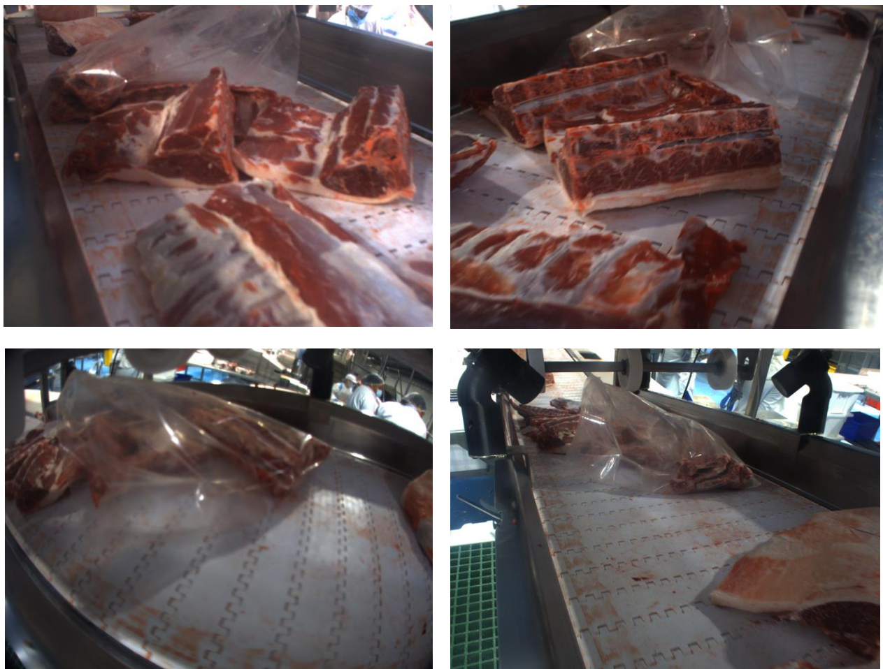
Figure 9: Captured frames at the prediction zone, showing a naked rack obscured from six cameras. Top, L-R: Camera 1 & 2, naked rack obscured by bag; Middle, L-R: Camera 3 & 4, naked rack partially obscured by naked loins; Bottom, L-R: Camera 5 & 6, naked rack obscured by bag.
