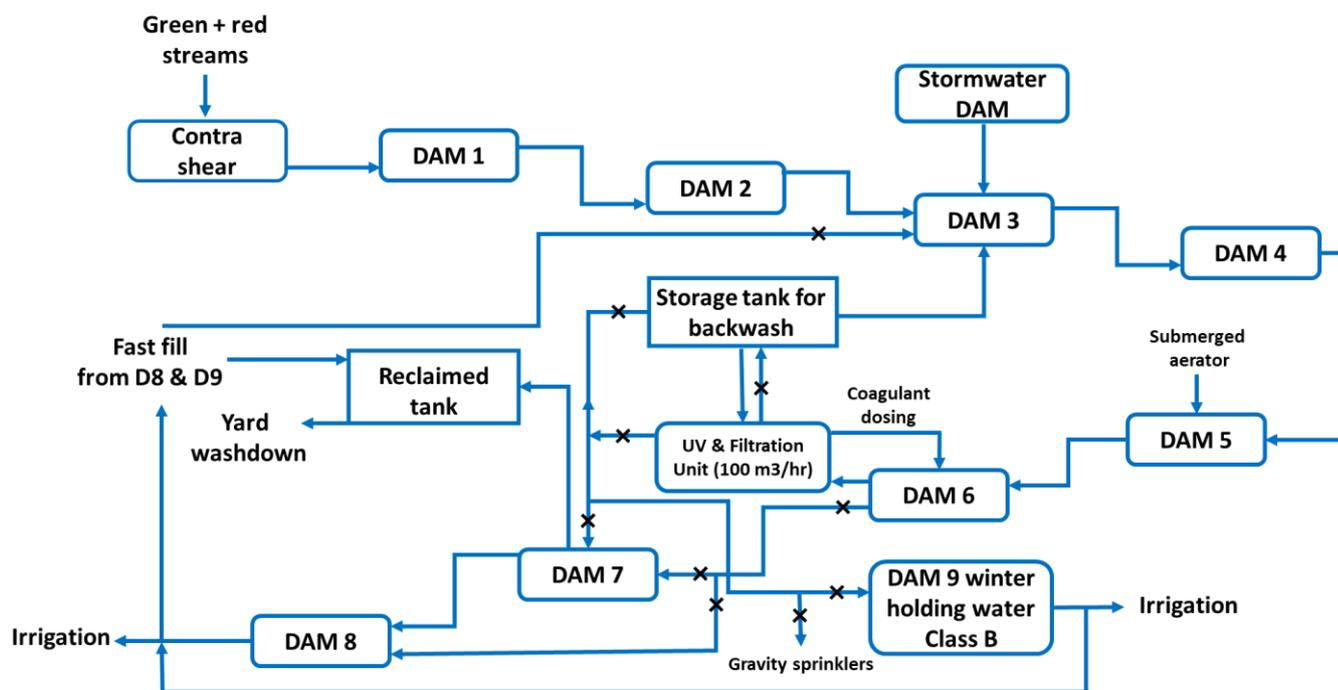
Figure 1: Wastewater process flowchart for abattoir V1. Feed from dam 7 to dam 9 and from dam 6 to dam 8 not shown for simplicity. 'x' indicates flow valves. Flowchart with full detail can be seen in Appendix 1
