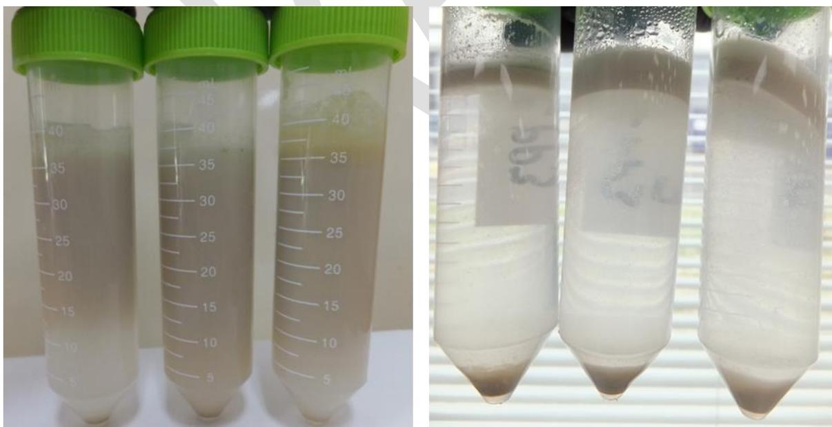
Figure 76: Three samples from the pre-PP3 black pit originating from the tallow rendering centrifuge wastewater without heating (left) and after centrifugation at room temperature (3200 rpm, 1717g for 3 min) (right).
