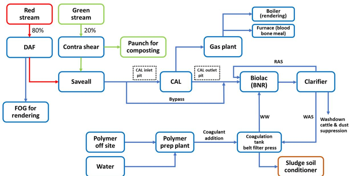
Figure 14: Wastewater process flow chart for abattoir Q1 showing water treatment processing technologies such as dissolved air floatation (DAF), covered anaerobic lagoon (CAL), Biolac biological nutrient removal (BNR), clarifier, coagulation tank and belt filter press. WW=wastewater, WAS=waste activated sludge and RAS=return activated sludge
