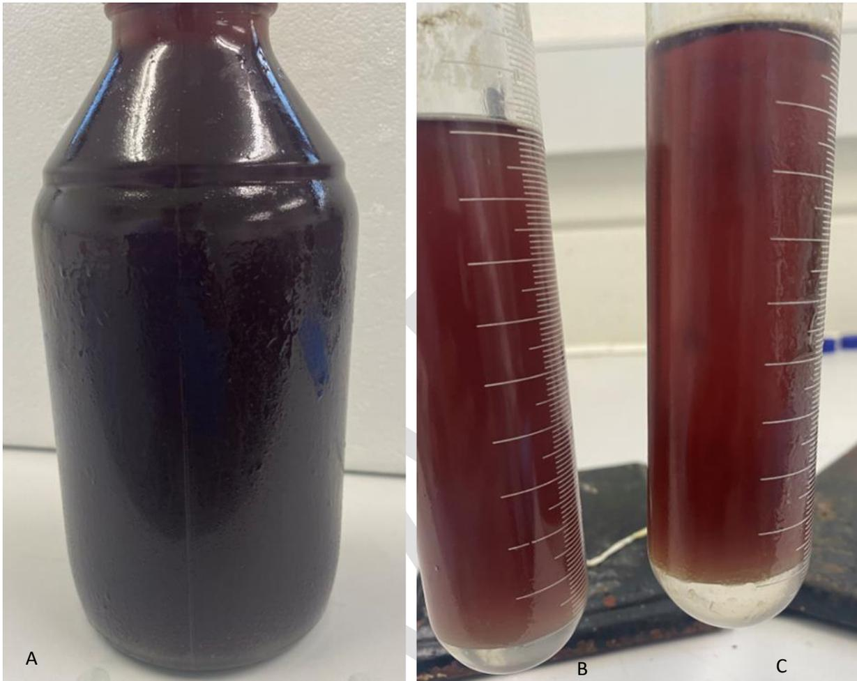
*Figure 75: PP3 black pit (from rendering centrifuge wastewater) FOG taken from the surface of the pit (A), heated non-MS control (B) and MS treated sample (C, 55 °C, 600 kHz, 20 min)*
