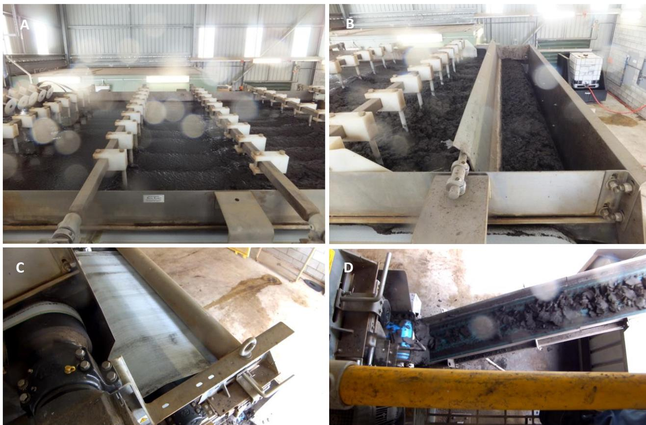
*Figure 20: Clarifier (Komline-Sanderon ROTO-KONE® High rate drainage system) main tank with flocculated sludge (A), end prior to the press showing sludge separated from water prior to filter press (B), dewatering filter press (C), and conveying of pressed sludge (D)*
