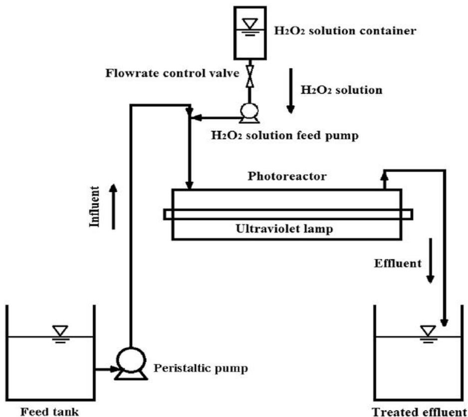
Figure 53: Schematic diagram of a single lamp UV/H<sub>2</sub>O<sub>2</sub> photoreactor [46]
