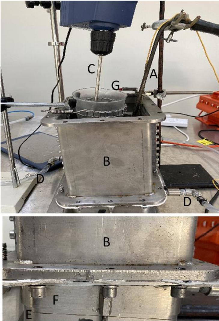
Figure 63: Experimental setup for megasonic treatment using a 600 kHz transducer array (SONOSYS®) mounted on the bottom for transmission from the bottom., A: electrical heater; B: megasonic reactor; C: electrical stirrer D: cooling hoses; E: transducer array plate; F: cooling jacket; G: glass tube
