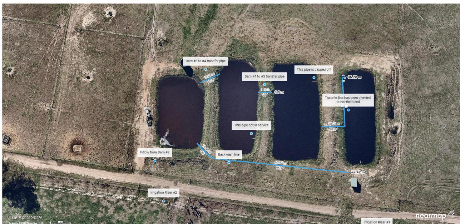
Figure 6: An aerial view of dams 3-6 which comprises the core of the water treatment dams downstream to dam 2, the second from the right (dam 5) is the aerated dam and the last (dam 6) is chlorinated and dosed with coagulant (polyaluminium chloride, PACL), UV treated and filtered
