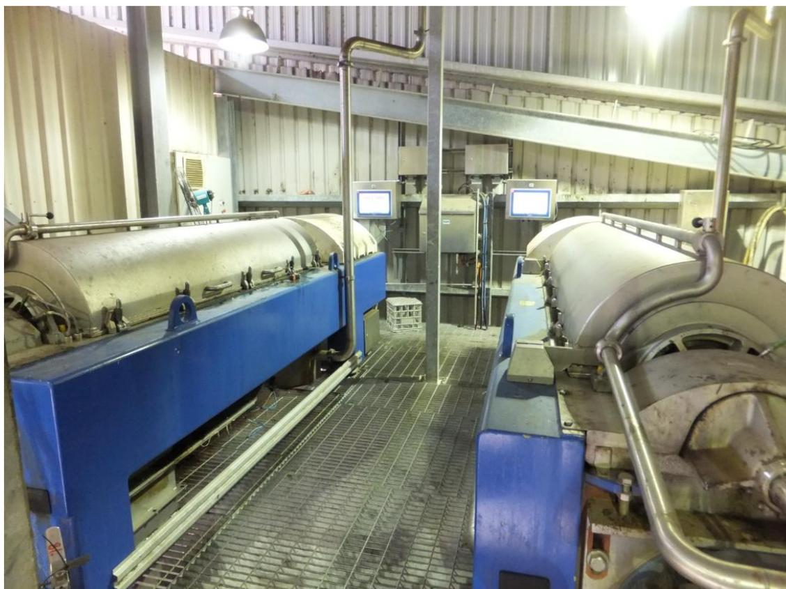
*Figure 43: Three phase decanters (tricanter) for separation of low-grade tallow sludge, dewatered sludge solids and centrate (water)*
