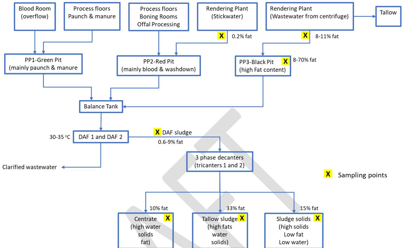
Figure 60: Process flow diagram of major FOG containing wastewater streams in Victorian abattoir V2
