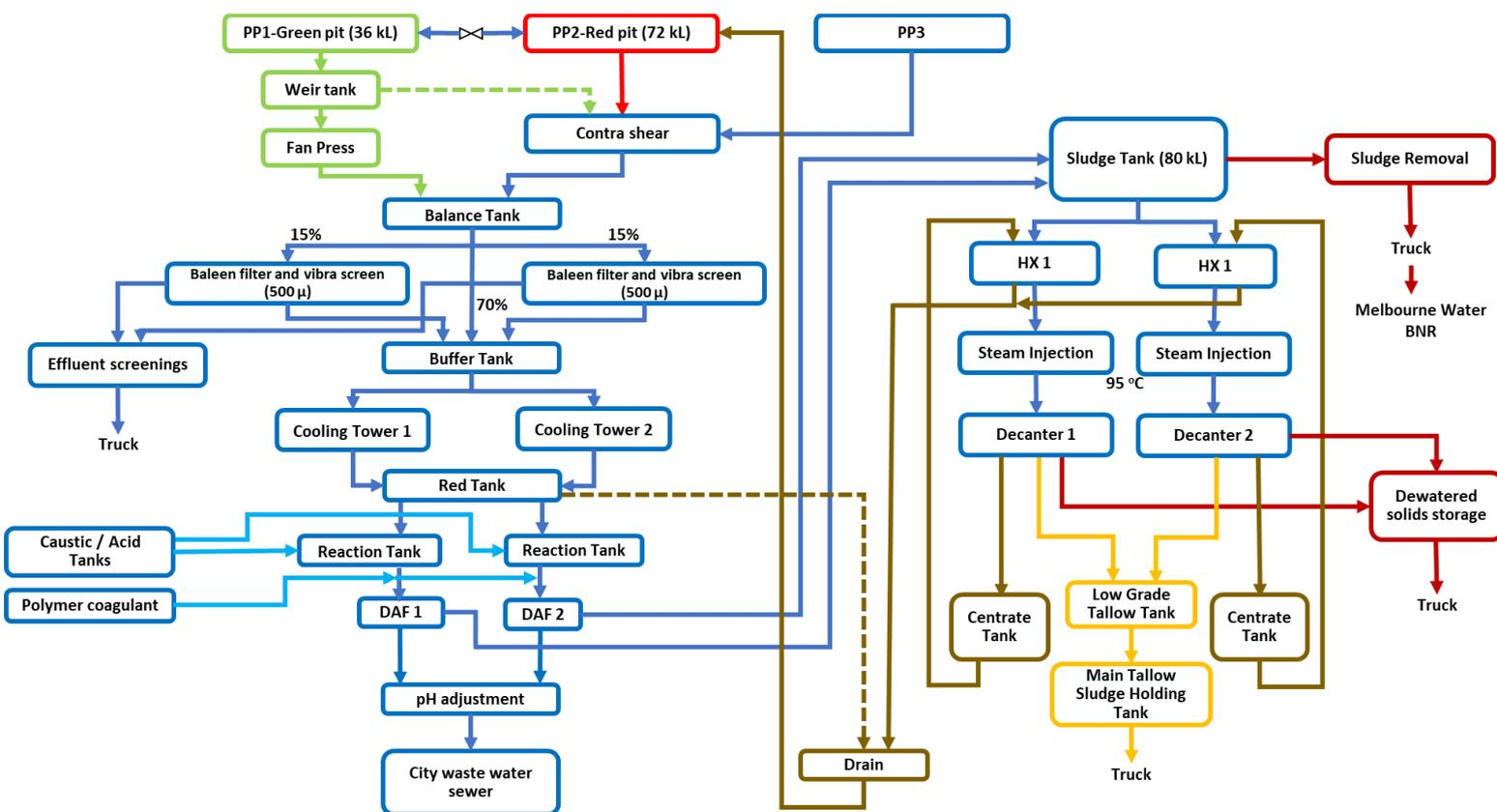
Figure 34: The wastewater process flow diagram for V2
