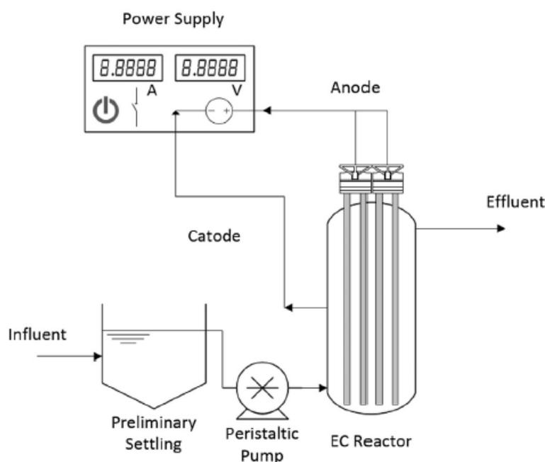
Figure 49: Electrocoagulation reactor [15]
