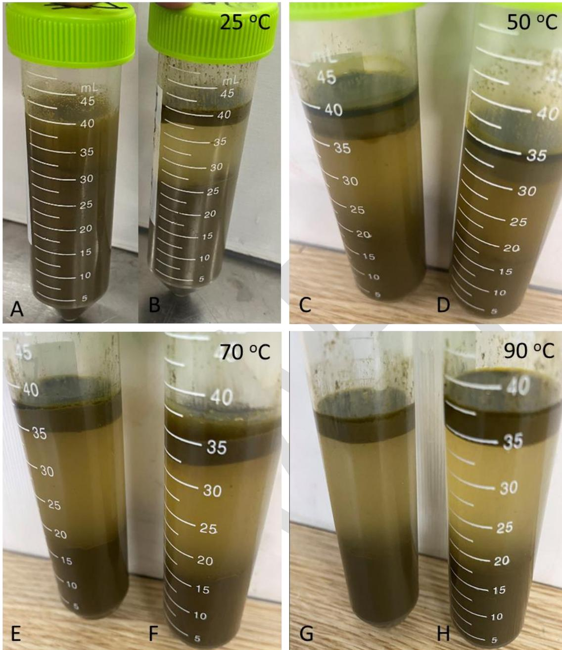
*Figure 66: DAF 1 sludge sample, control (A), megasonic (MS) treatment (B) at 25 °C; control (C), MS treatment (D) at 50 °C; control (E), MS treatment (F) at 70 °C; control (G), MS treatment (H) at 90 °C with 600 kHz from the bottom for 20 min followed by centrifugation at 3200 rpm (1717 g) for 5 min.*
