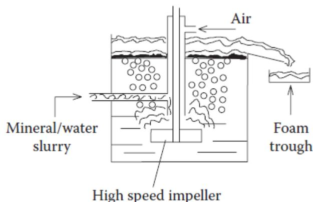
Figure 48: High speed impeller froth floatation [1]
