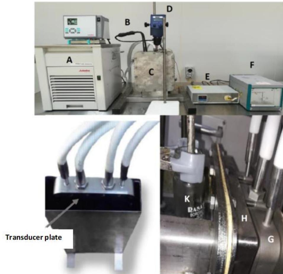
Figure 62: Experimental setup for megasonic treatment using a 2 MHz transducer array (SONOSYS®) vertically bolted for transmission from the side., A: cooling system; B: electrical heater; C: megasonic reactor, D: electrical stirrer; E: temperature control; F: generator; G: transducer array plate; H: cooling jacket; K: glass tube
