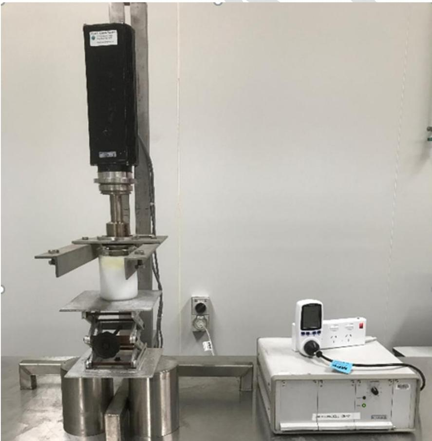
Figure 65: 20 kHz ultrasound sonication sonotrode (Heischer UIP1000) for mid temperatures up to 65 °C
