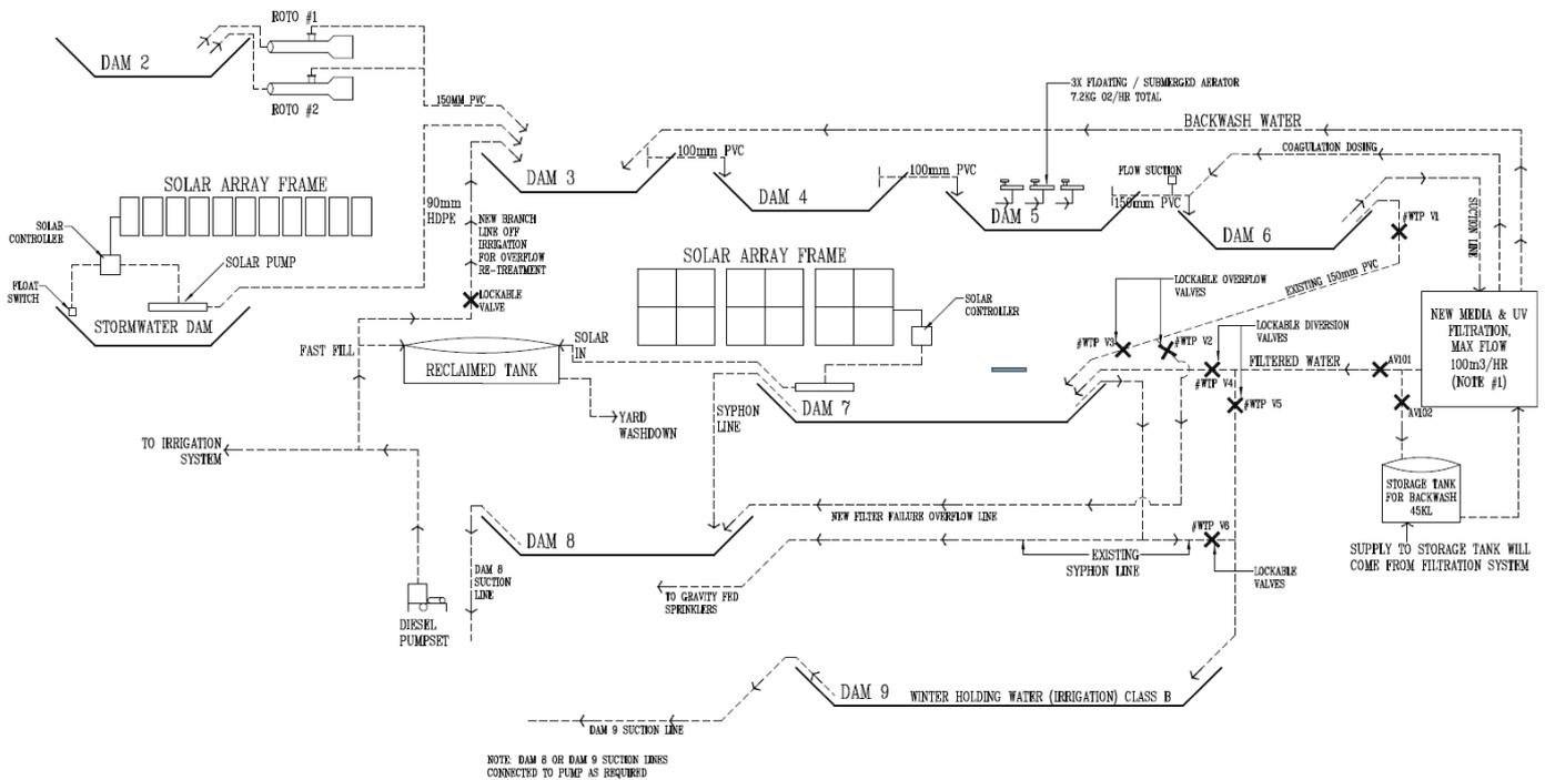
Figure 1. Detailed process flow diagram for abattoir V1
