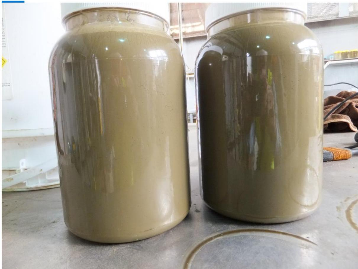
*Figure 45: Centrate water showing thick emulsion likely to contain large amounts of solids (FOG) as well as some unseparated sludge*
