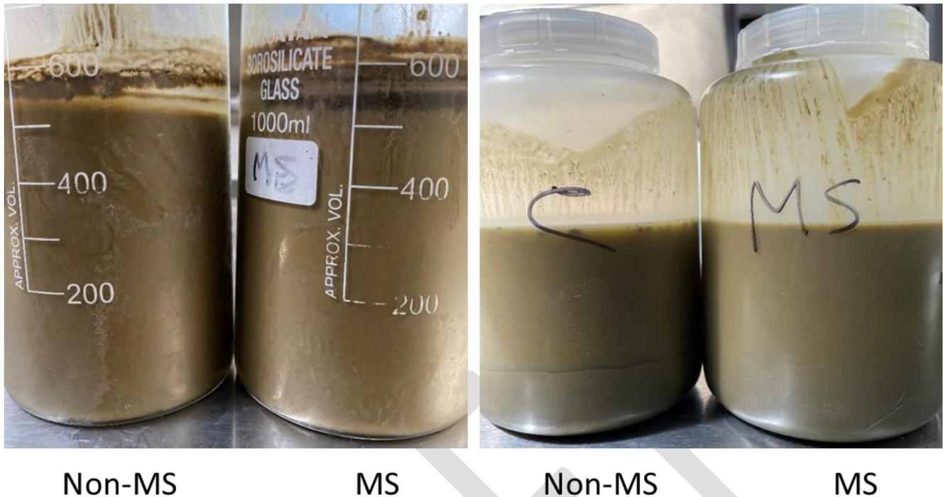
Figure 70: Decanter centrate without and with MS treatment (600 kHz from the bottom, 20 min, 50 °C) with mixing, before (left) and after centrifugation (right, 3200 rpm, 1717 g, 12 min)
