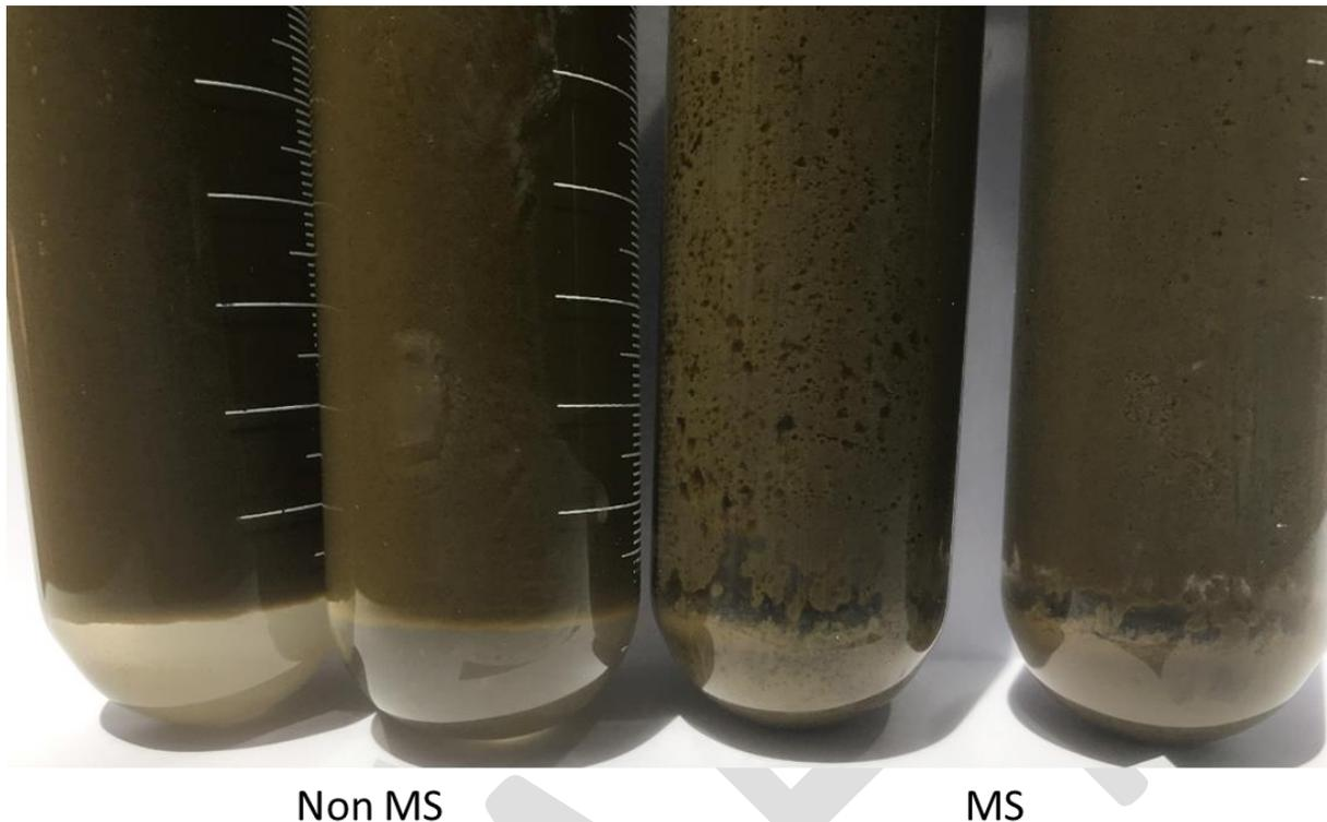
*Figure 72: Decanter tallow sludge from abattoir V2 subjected to megasonic treatment at 60 °C for 20 min with side on irradiation using 600 kHz transducer array*
