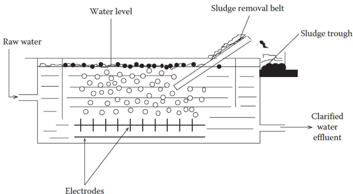
Figure 46: Electro-floatation tank [15]
