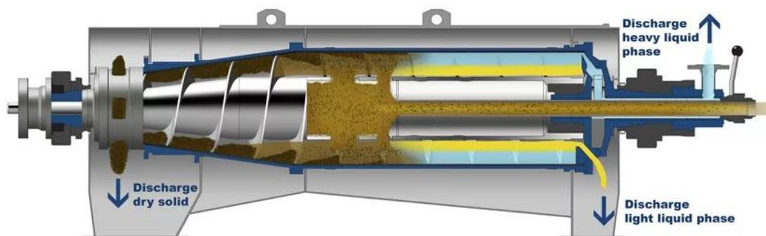
Figure 54: Three-phase centrifuge (decanter) separation of water, oil and solids with the Flottweg Tricanter® (<https://www.flottweg.com/product-lines/tricanter/>)
