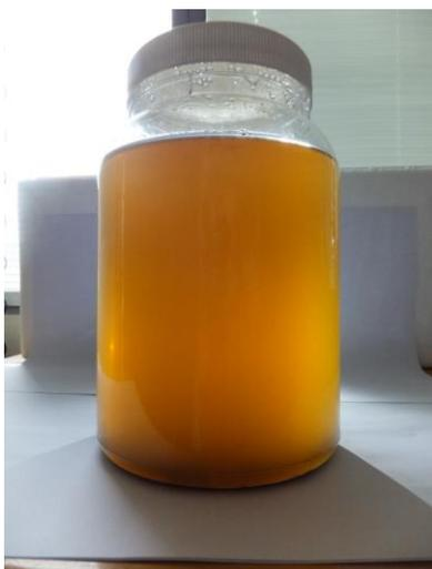
Figure 5: Sample of surface water with scum showing fine particles settling out with time and very little if any floating FOG
