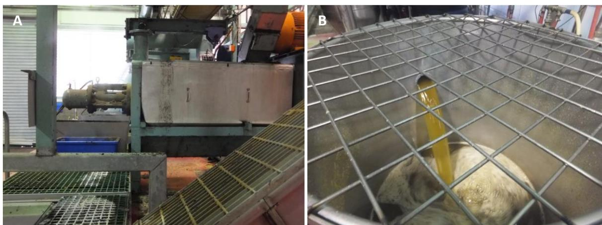
Figure 22: Render press (A) for pressing out residual tallow from bone meal and returned to vibrating screen (Figure 21B), and hot final tallow product (B) after centrifugation of tallow by decanter after crude separation from bone-meal by vibrating screen (Figure 21B)
