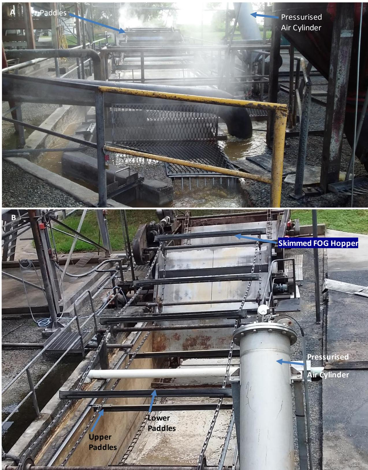
Figure 29: DAF-saveall full and operating with aeration DAF zone front and saveall zone rear (A) and empty (B) showing pressurised air cylinder and chain-driven surface FOG skimming paddles and lower return mixing paddles
