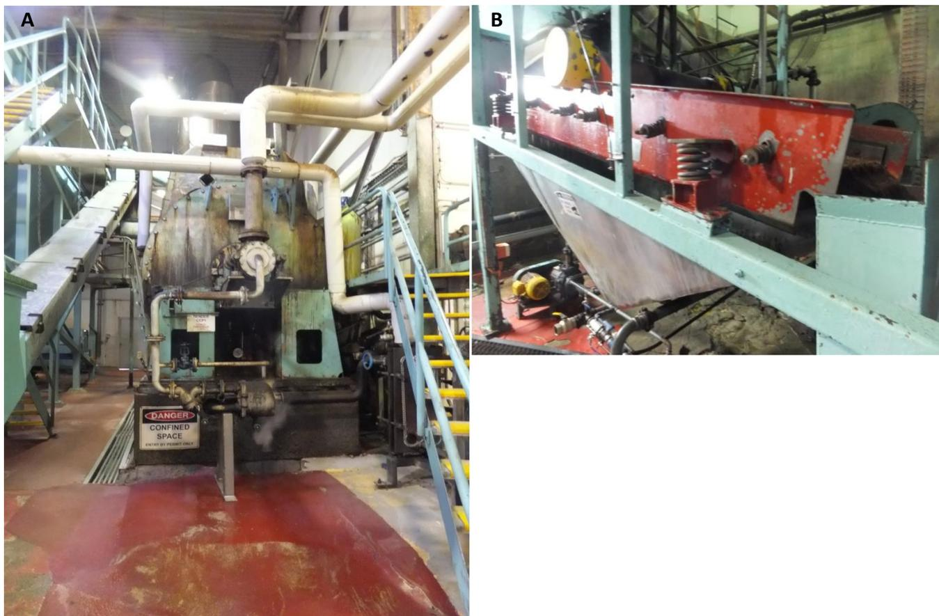
Figure 21: Render cooker (A) and vibrating screen (B) to separate tallow from bone
