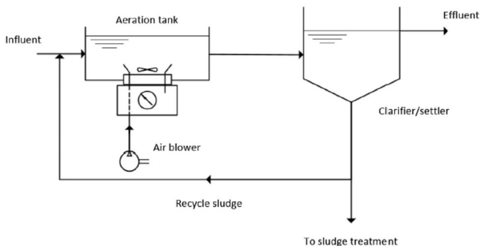
Figure 52: Activated sludge process [1]
