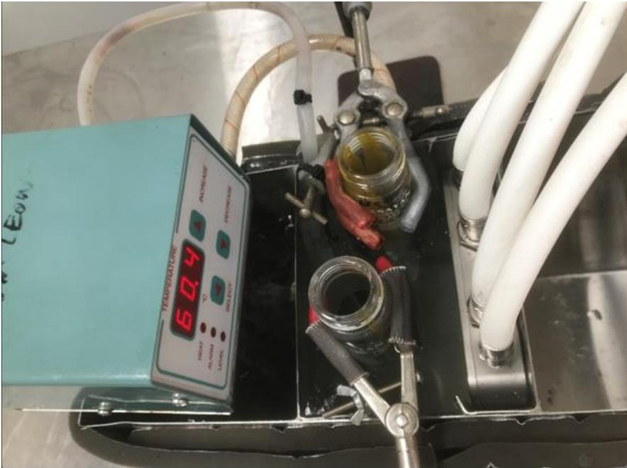
Figure 64: 600 kHz megasonic reactor with horizontal irradiation from transducer array (SONOSYS®) with a recirculating bath temperature control
