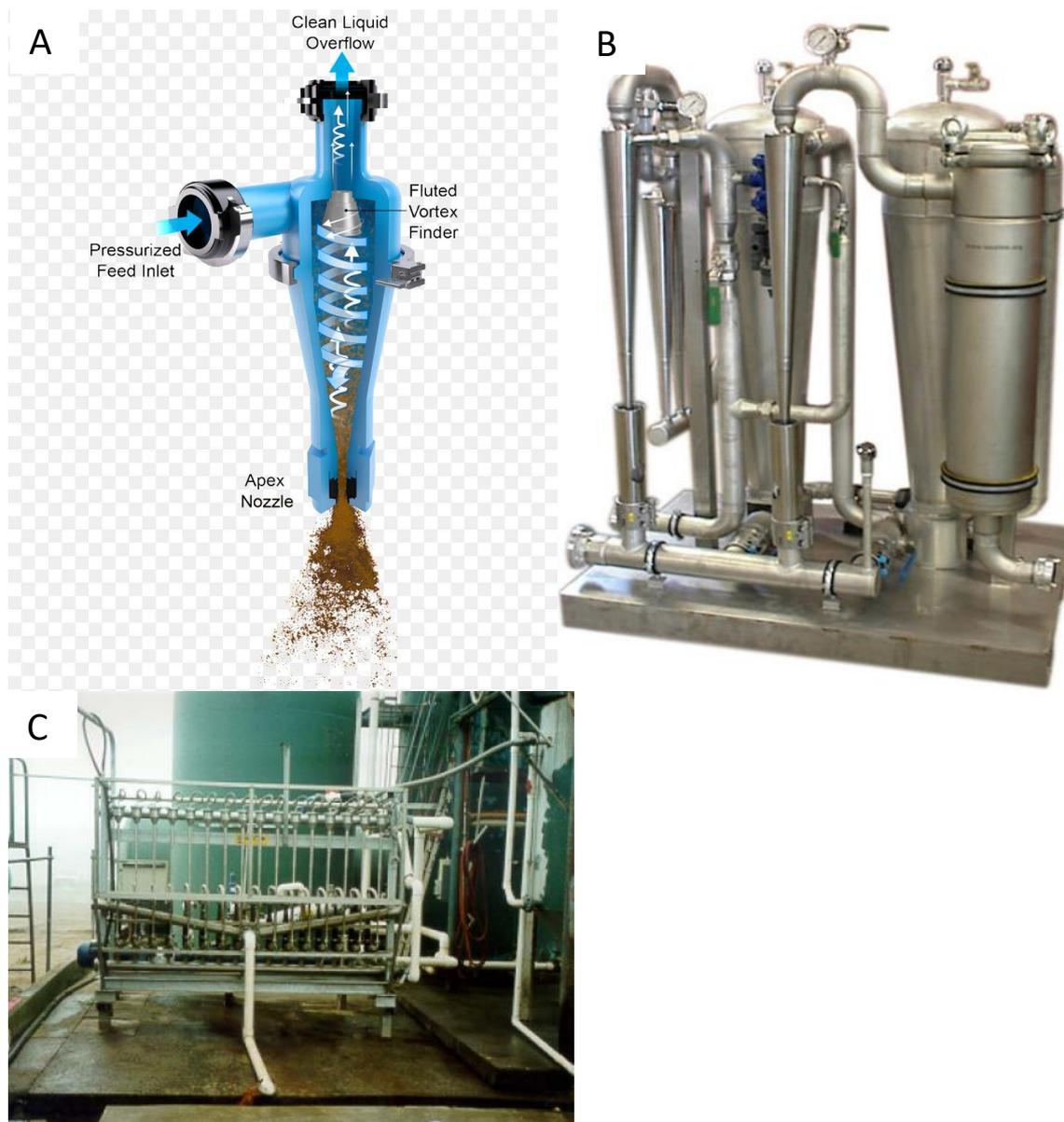
Figure 55: Drawing of interior of a hydrocyclone showing centrifugal vortices for separation of solids water and fats (A) <https://www.pngwave.com/png-clip-art-wetjd>, larger scale unit (B) sold by WyanaSep [https://wyunasep.com/lib\\_docs/WyanaSep\\_Meatwork\\_Brochure.pdf](https://wyunasep.com/lib_docs/WyanaSep_Meatwork_Brochure.pdf), and an operational hydrocyclone installation at a meat processing plant (C) [75]
