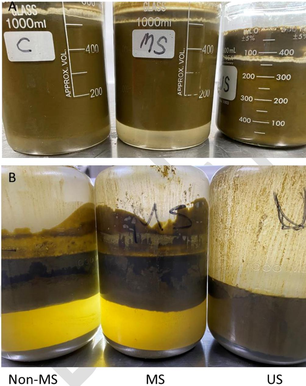
Figure 73: Decanter tallow sludge non-MS heated control, MS treated at 600 kHz from the bottom, 50 °C, 40 min with mixing and ultrasound treated using 20 kHz, 50 °C, 3 min, Standing for 30 min (A) and centrifugation for 12 min at 3200 rpm, 1717g (B)
