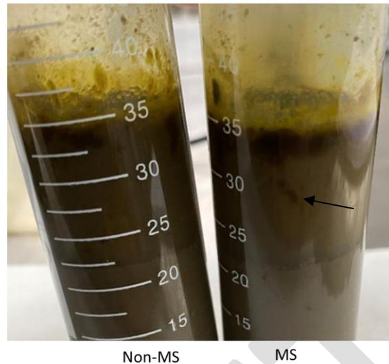
*Figure 69: DAF 1 sludge centrifuged after MS treatment (600 kHz, 20 min, 50 °C) and centrifuge at 3200 rpm, 1717 g for 5 min. Arrow show partially coalesced FOG region in the process of rising to the surface. A partially coalesced FOG pocket is indicated by the arrow*
