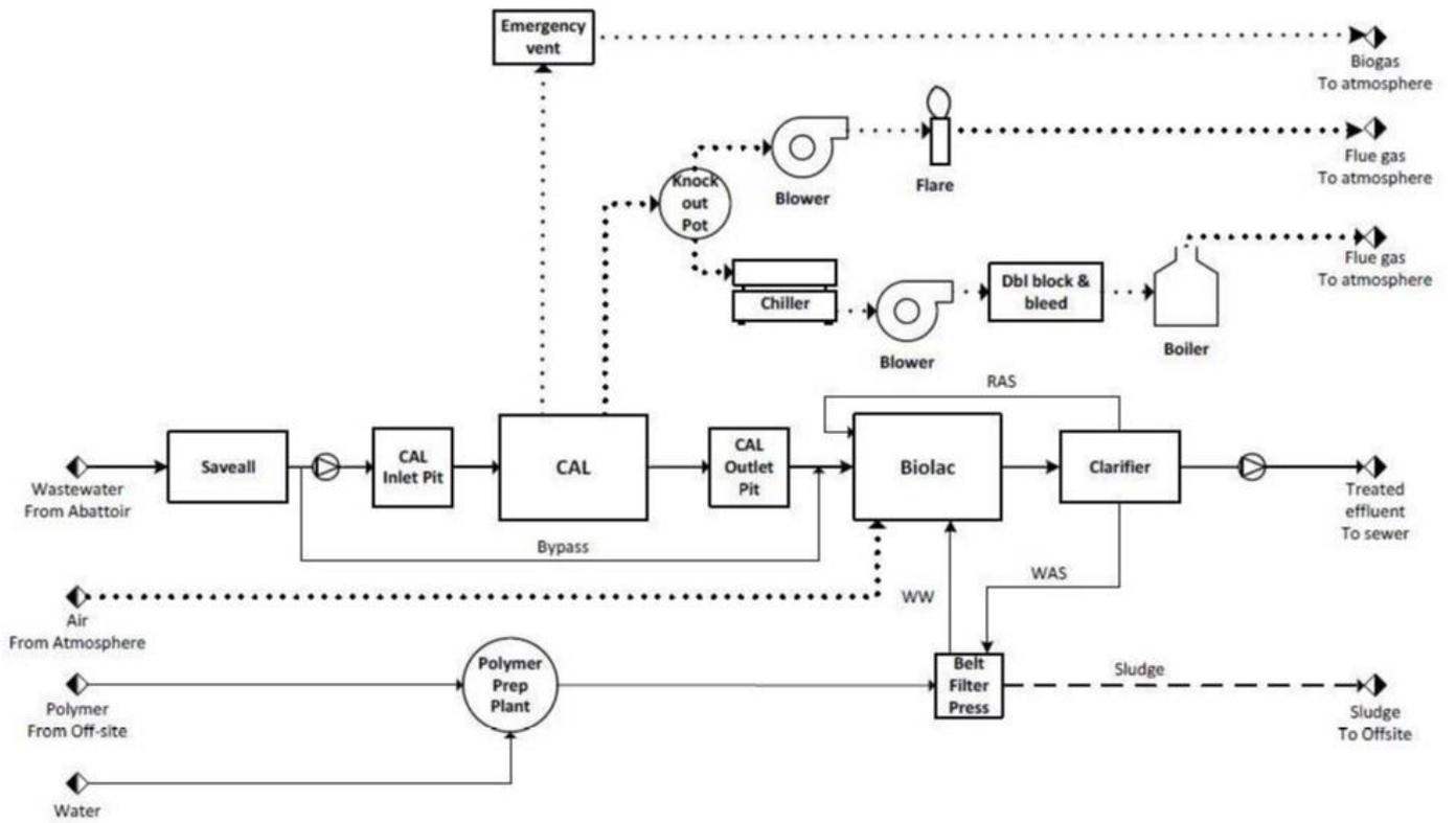
Figure 2. Detailed process flow diagram for abattoir Q1
