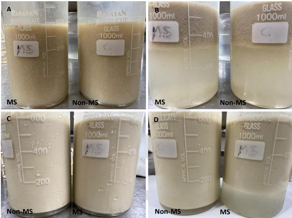
Figure 77: Pre-PP3 black pit, rendering centrifuge wastewater, heated at 55 °C with and without MS (600 kHz from the bottom, 20 min with mixing) (A), after 45 min cooling (B), heated at 25 °C with and without MS (600 kHz from the bottom, 20 min with mixing) (C) and standing at room temperature for 2 hrs (D)
