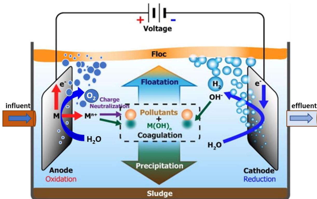
Figure 50: Diagram of electrocoagulation wastewater treatment process (modification of Chanjiang et al. (2017) [28])
