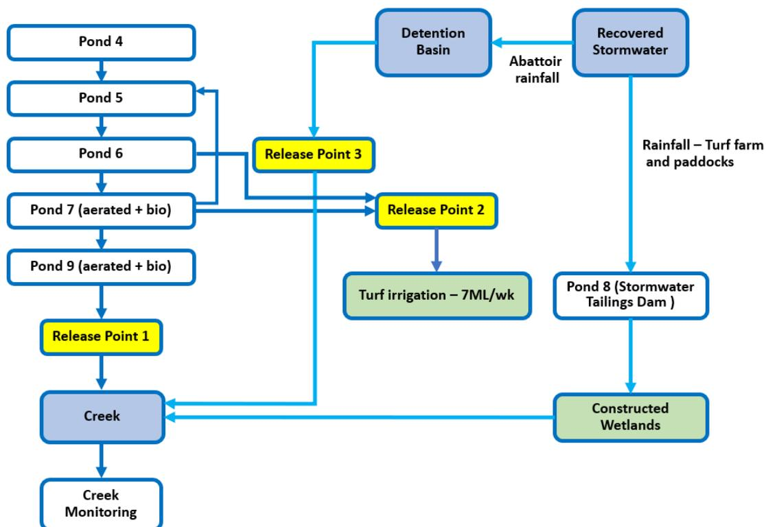
Figure 25: Wastewater treatment flow diagram for Turf farm wastewater system and release of treated water to constructed wetlands and the nearby creek
