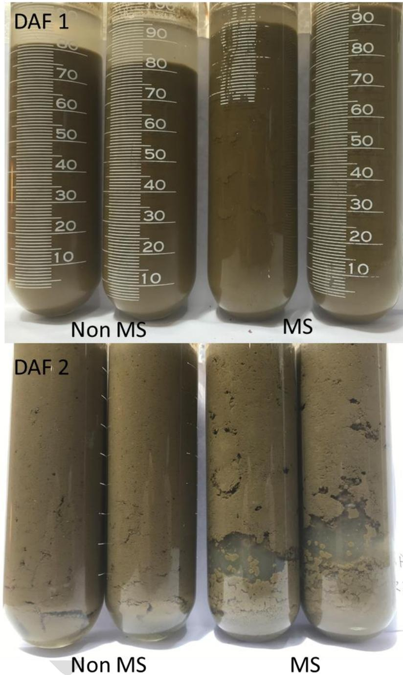
Figure 68: DAF sludge from DAF 1 and DAF 2 subjected to megasonic treatment at 60 °C for 20 min with side on irradiation using 600 kHz transducer array
