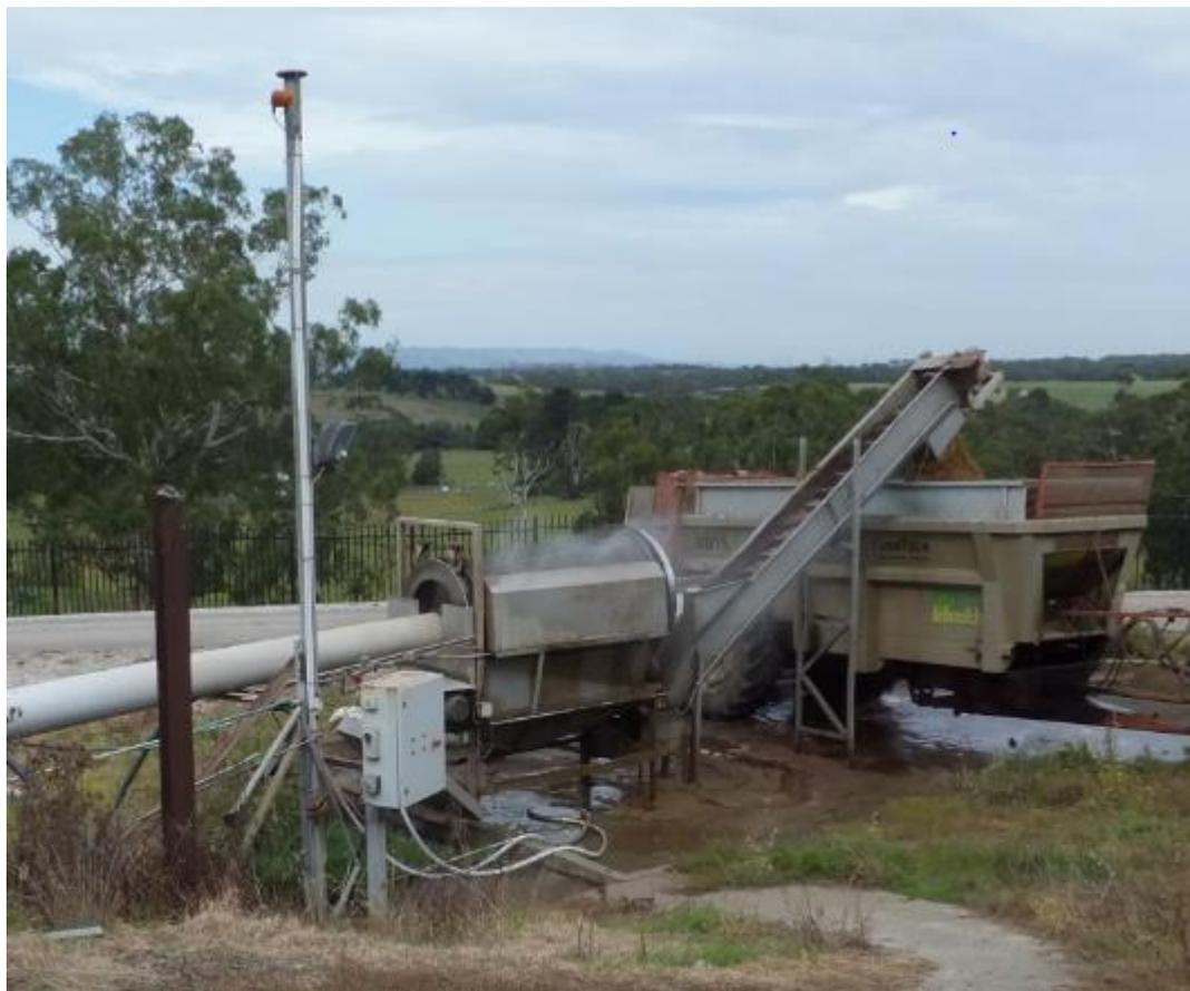
*Figure 2: Rotary sieved drum (Contra shear) with an inclined auger for separation and removal of paunch from combined red and green wastewater streams*
