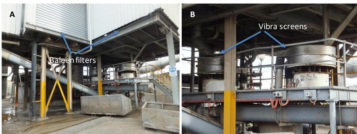
Figure 38: Level 2 shows building housing Baleen filters (A) and partially filtered wastewater sent to the Vibra screens (below) for further filtering (B)
