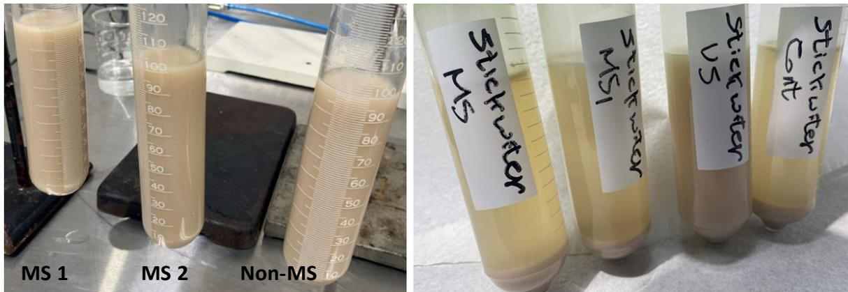
Figure 79: PP2 red pit rendering stickwater with megasonic (MS) treatment (600 kHz, 50 °C, 20 min) and non-MS treatment (left) and MS and ultrasound treatment (US, 20 kHz, 50 °C, 2 min) and non-MS treatment after centrifugation, 3200 rpm, 1717g, 5 min (right)
