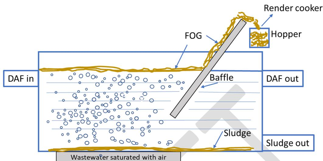
Figure 61: Diagram of dissolved air flotation (DAF) tank showing floatation of FOG float and sedimentation of sludge on bottom
