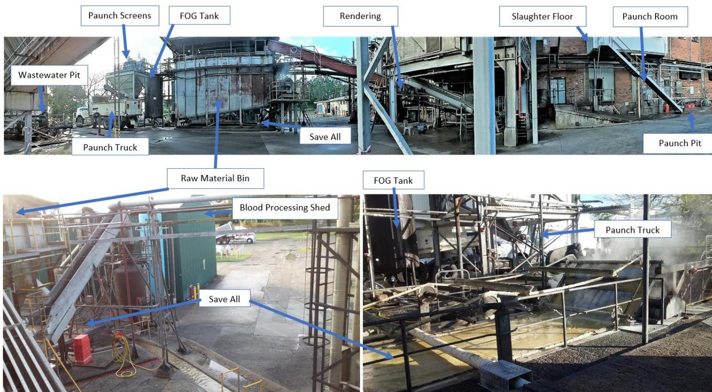
Figure 28: Major areas and processes of interest in abattoir and wastewater treatment prior to pond system including red and green wastewater stream, separation of paunch, DAF-saveall and wastewater pit
