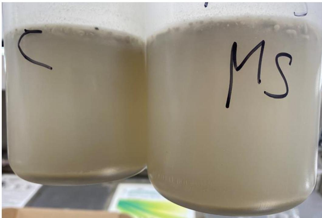
Figure 78: pre-PP3 black pit rendering centrifuge wastewater without and with MS treatment (600 kHz, from the bottom at 50 °C for 20 min with mixing) after cooling for 45 min (refer to Figure 77B) after centrifuging at 3200 rpm, 1717 g, 12 min
