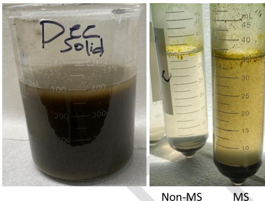
Figure 71: Decanter sludge solids diluted with water (5:1 v/w, left), without MS and with MS treatment (600 kHz, 20 min, 60 °C) with mixing, after centrifugation (right, 3200 rpm, 1717 g, 5 min)
