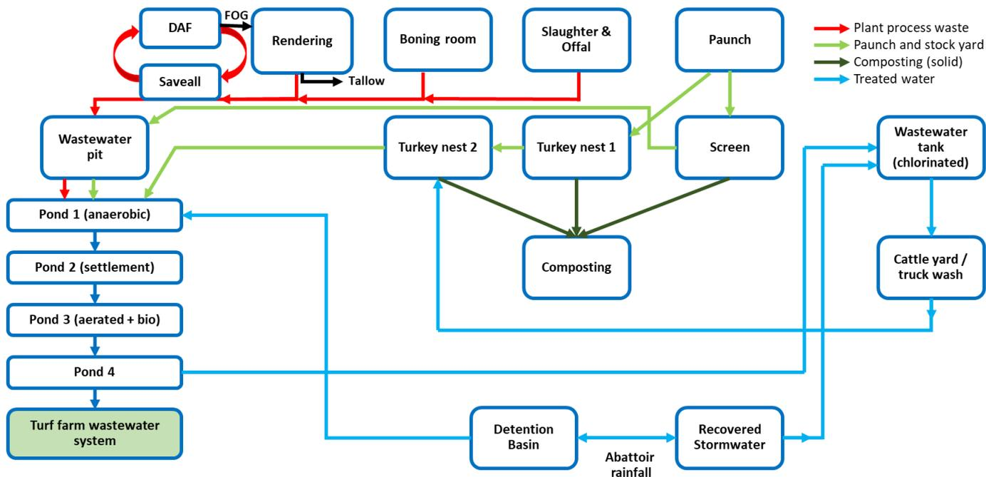
Figure 24: Green and red wastewater stream process flow diagram prior to further treatment, use in turf farm and release of treated water into the environment (Figure 25)
