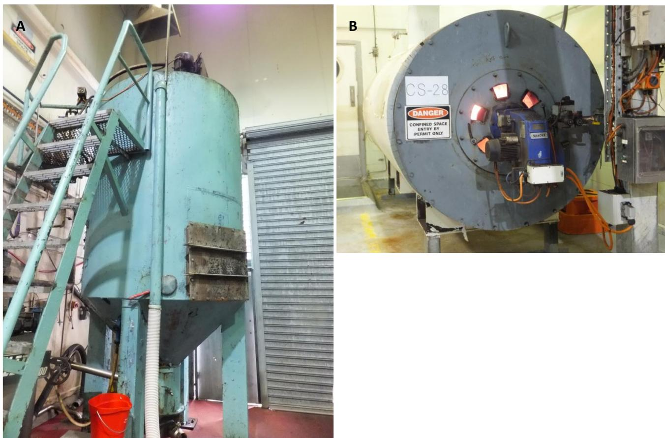
Figure 23: Raw blood storage tank (A) and raw blood dryer (B)
