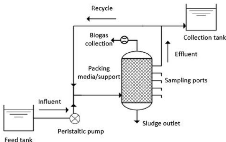
Figure 51: Anaerobic filter [40]
