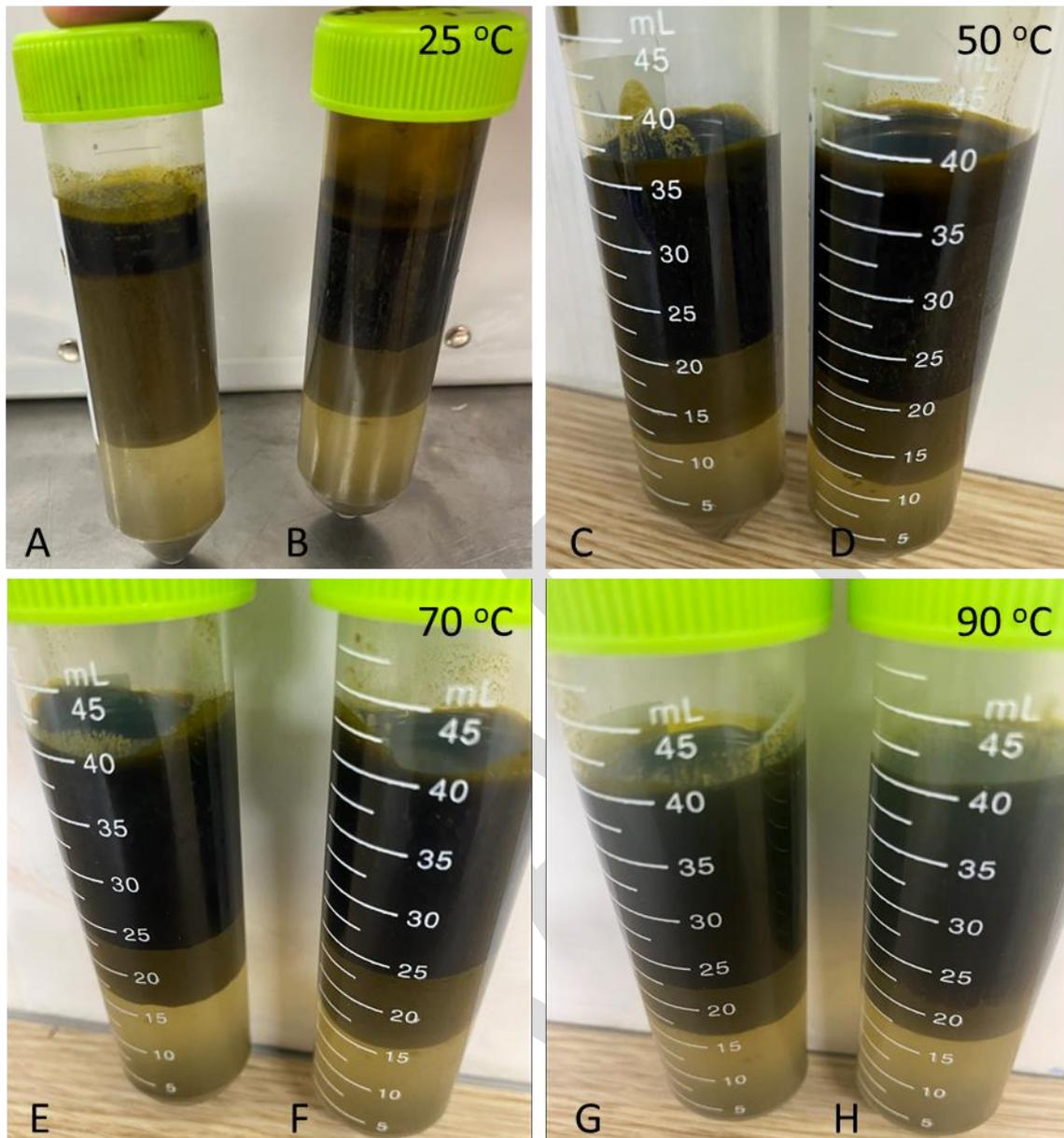
Figure 67: Decanter tallow sludge sample, control treatment (A), (B) megasonic (MS) at 25 °C; control (C), MS treatment (D) at 50 °C; control (E), MS treatment (F) at 70 °C; control (G), MS treatment (H) at 90 °C with 600 kHz for 20 min followed by centrifugation at 3200 rpm, 1717g for 5 min.
