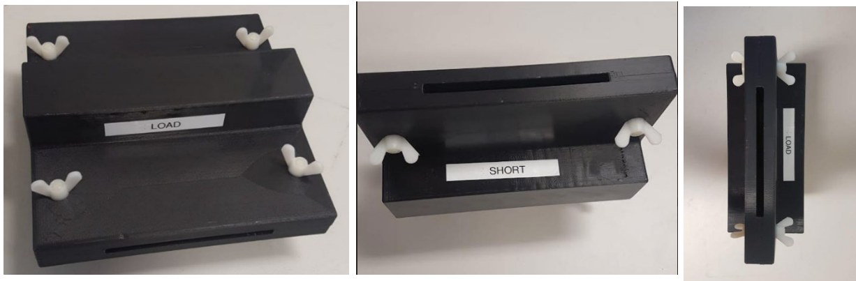
Figure 1 Short and load calibration blocks for the Vivaldi Patch Antenna
