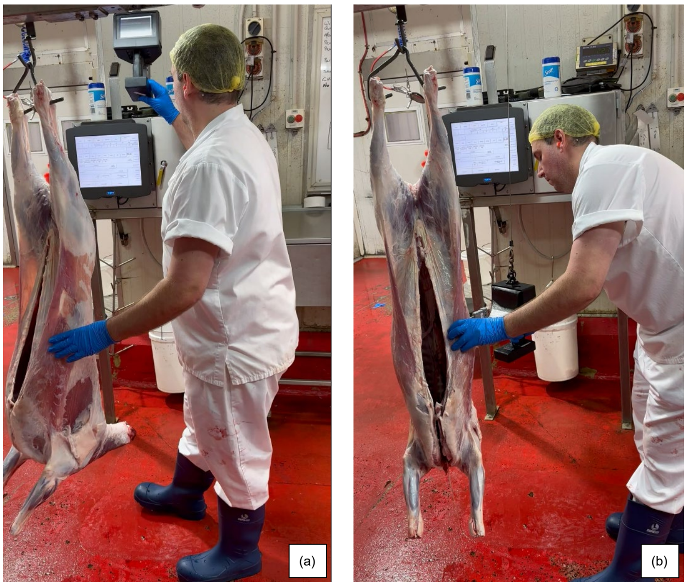
Figure 15 (a) MiS device location on chain when not in use. (b) MiS measuring hot carcass GR tissue depth
