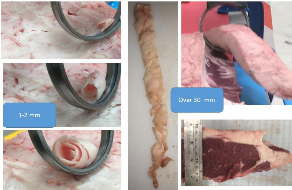
Figure 18: Trimming capability test reaching the range 1 mm – 30 mm.
