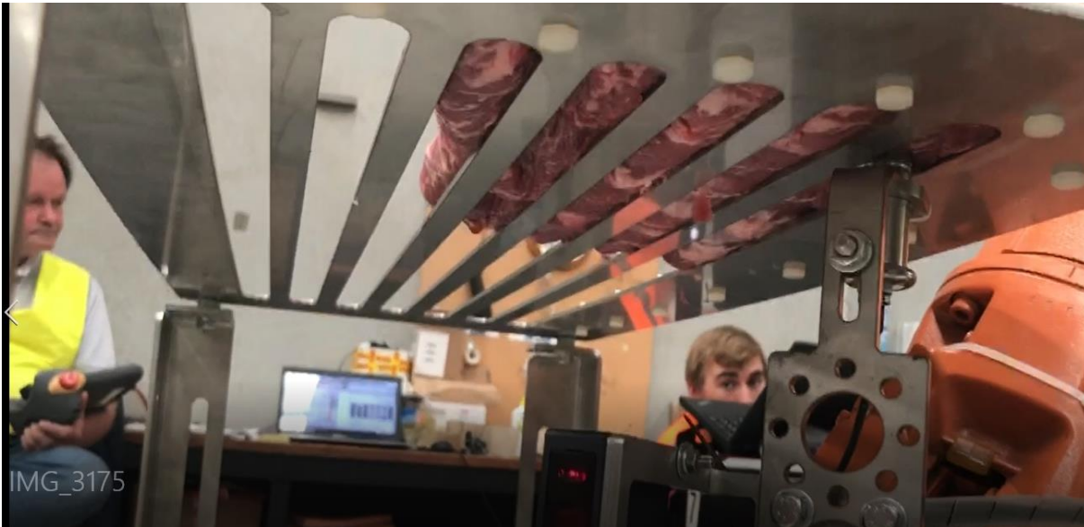
Figure 28: Measuring MT (Meat Thickness) with ultrasonic sensor from below.
