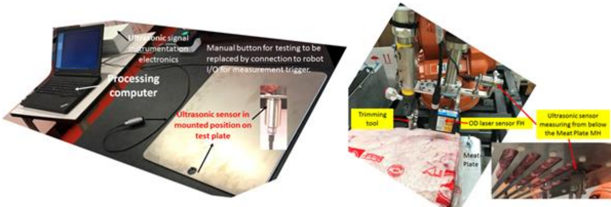
Figure 4: Ultrasonic and laser measurements arrangements.
