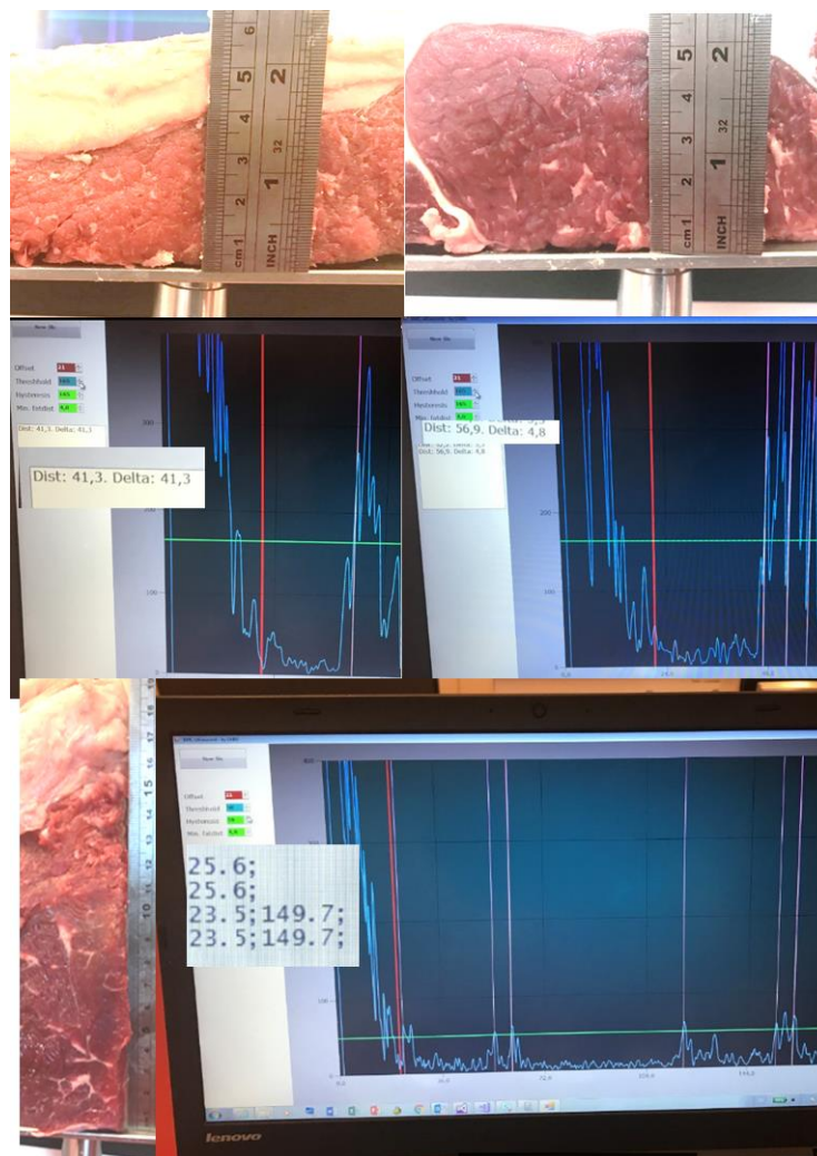
Figure 12: Ultrasonic sensing test results for the range of striploin thicknesses.
