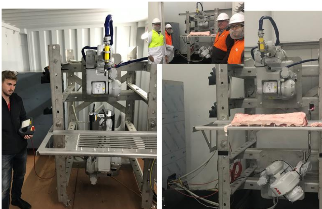
Figure 5: Two-arm robot arrangement at USQ (left) and in plant trials (right).
