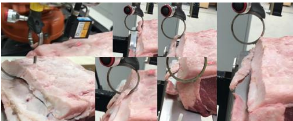
Figure 31: First test of the physically integrated end-effector with IRB 140.
