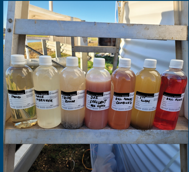
Figure 1 Red and green streams sampled to assess viability in a water recycling plant.
