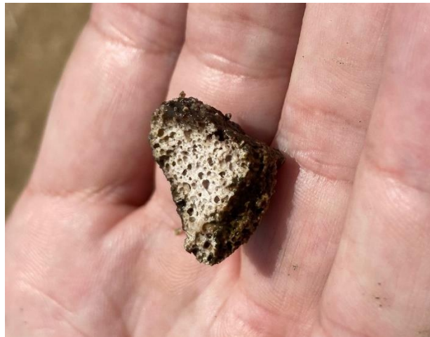
Figure 4-3: Hebel™ Media Showing Initial Bacterial/Algal Growth
