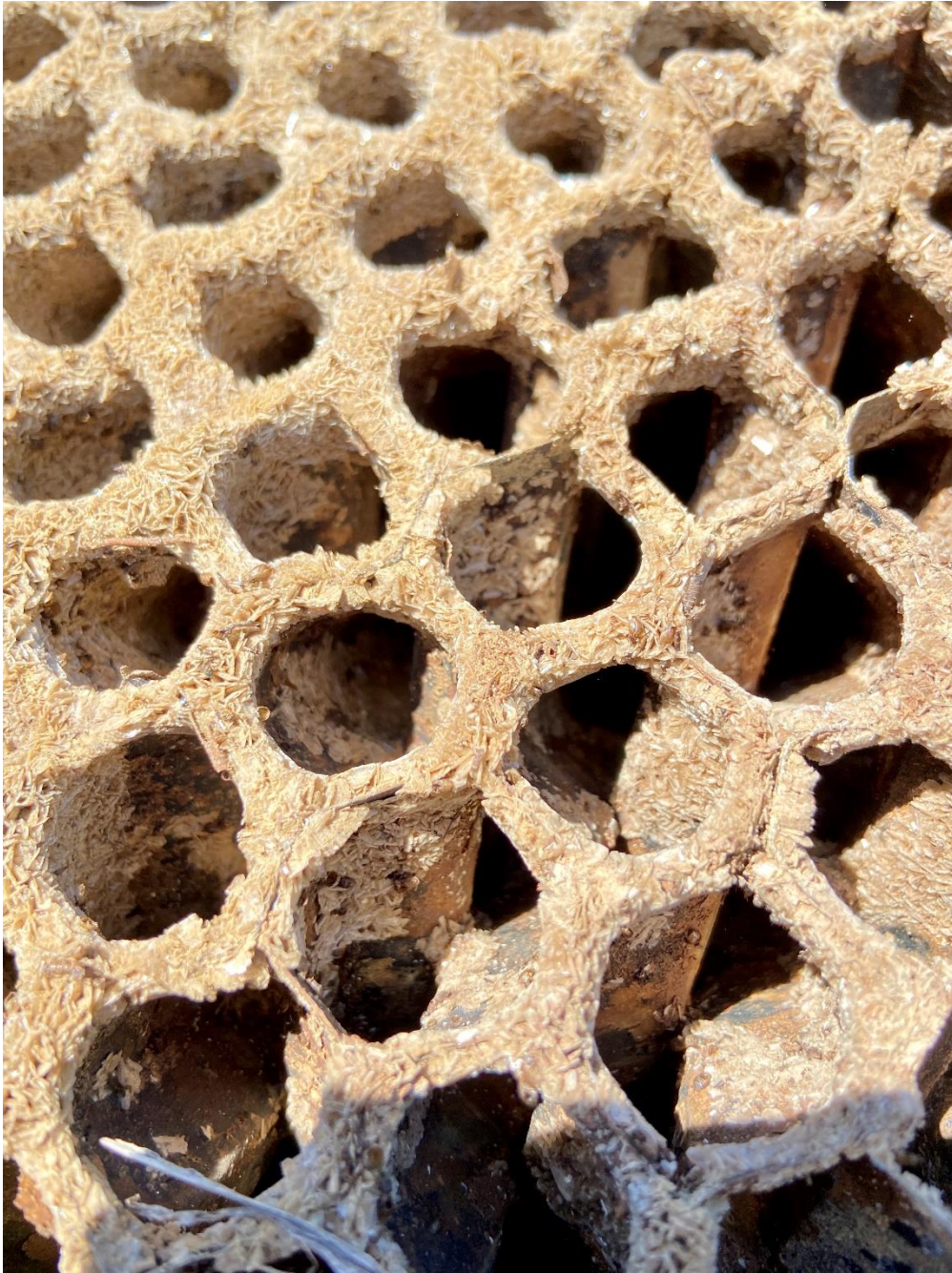
Figure 5-1: Crystalline Build-up (Struvite) on Plastic Media
