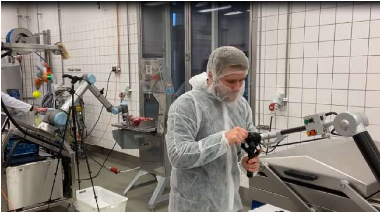
Figure 1. Cutting 50mm 1 shank cuts on bandsaw by means of a telemanipulator and a robotic arm
