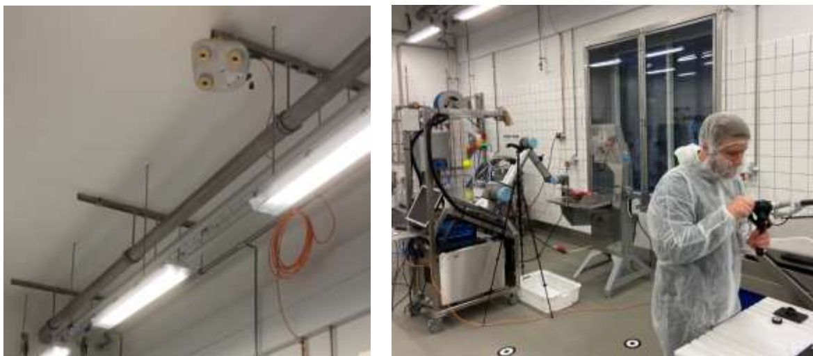
Figure 5 and 6: Pilz safety system in ceiling(left), an Pilz zone in pointers on floor, traffic light behind, yellow camera above robot provides close up monitoring on a screen for the operator using the Virtuose 6D manipulator
