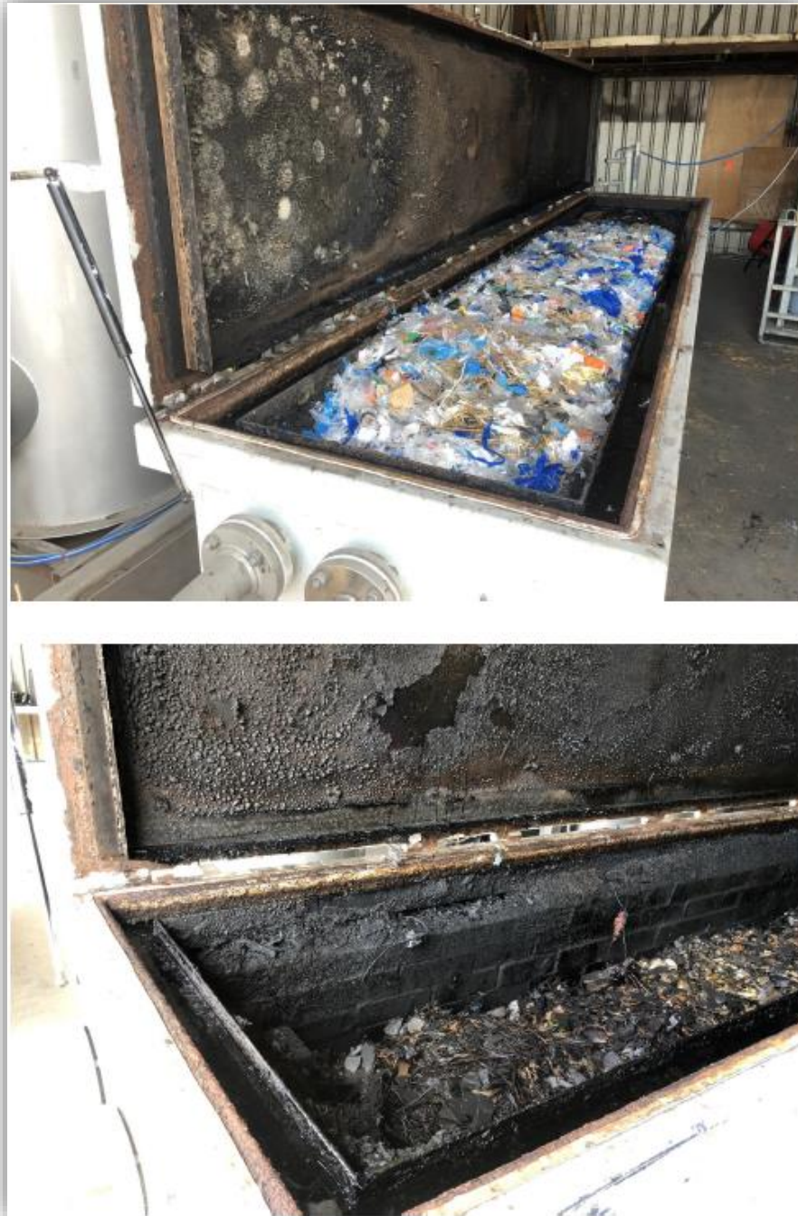
Figure 20: Run 1 showing compacted feedstock and remaining char/slag
