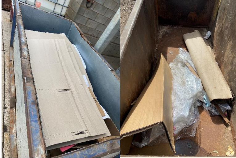
Figure 11: Contaminated cardboard and plastic. Noted was the need to shred large sheets to improve packing density along with available surface area for gasification
