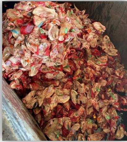
Figure 12: Ears and tags. Tags will be an ideal gasification substrate, whereas ears may contain a prohibitively high moisture content. If possible, these should be separated, or blended with drier feedstocks.
