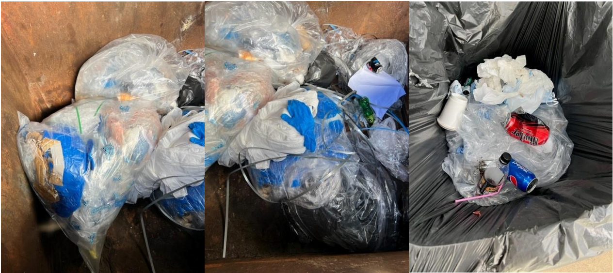
Figure 17: Production and change room waste. Where possible, inerts such as aluminium cans should be removed as they produce no benefit in gasification and instead may present issues with materials handling and heat transfer
