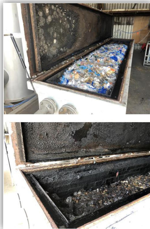
Figure 1: Gasification reactor showing mulched mix of paper, cardboard, and plastic, and residual char
