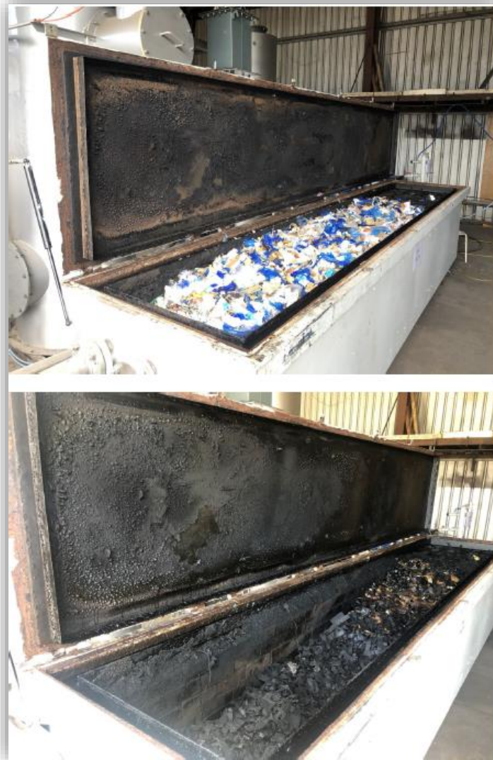
Figure 25: Run 2 showing compacted feedstock and remaining char/slag
