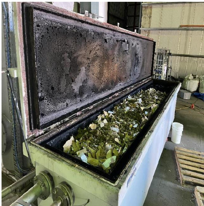
Figure 28: MIHG reactor packed with non-recyclable organics, inorganics, and paunch
