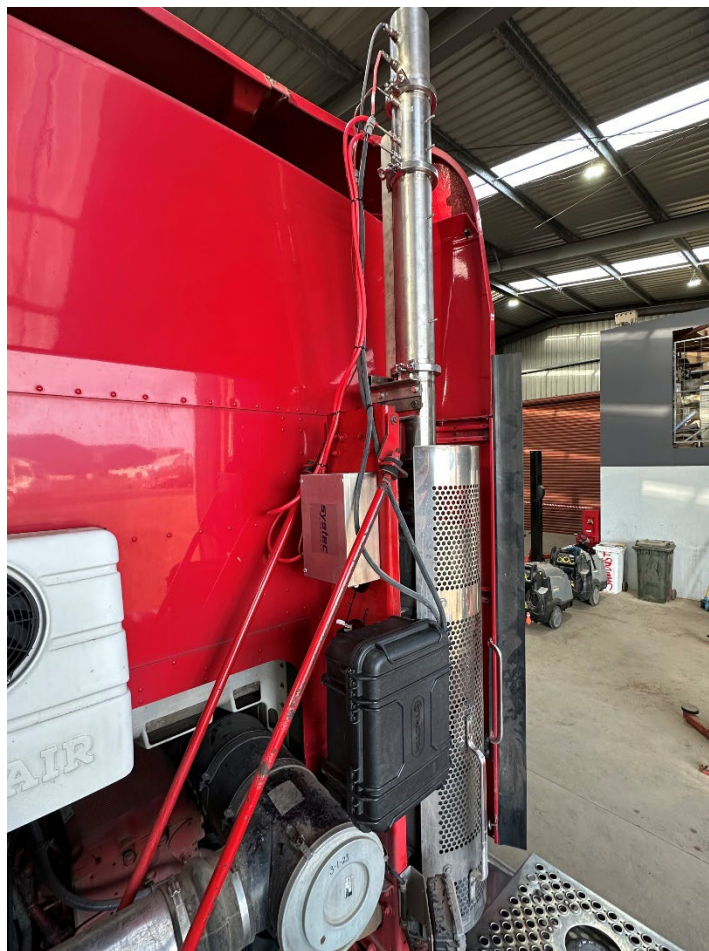
Figure 11: Completed mini PEMS installation.
