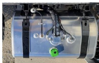
Parallel B100 Tank and Heat Exchanger
