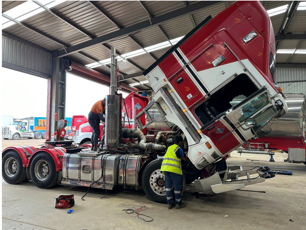
Figure 10: mini PEMS installation and wiring.
