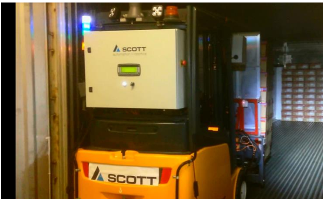
Figure 26: The AGV enters the container and positions the stack, sideshifting to place adjacent to container wall
