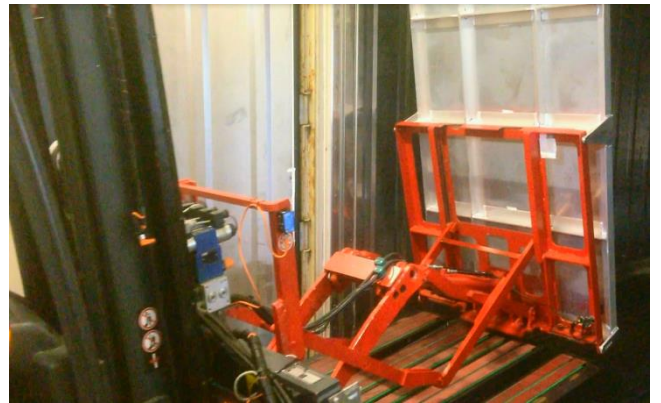
Figure 31: The AGV reversing out of the container, with pusher plate still in the extend position
