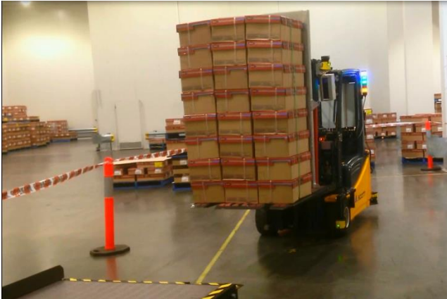
Figure 25: The AGV reverses and lowers the stack before moving towards the designated container
