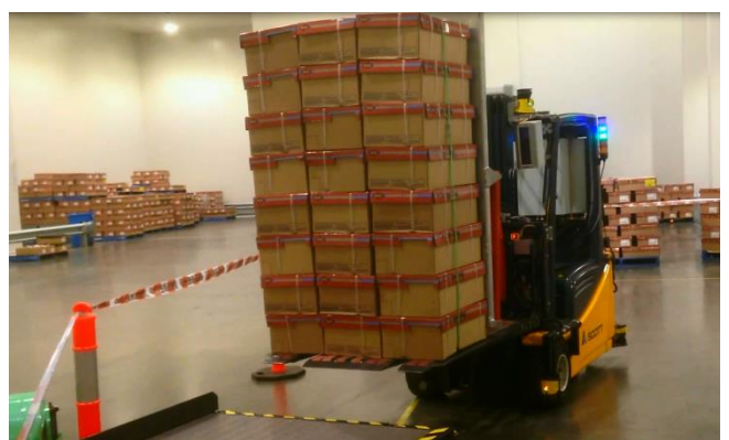
Figure 24: The AGV simultaneously raises the stack and reverses
