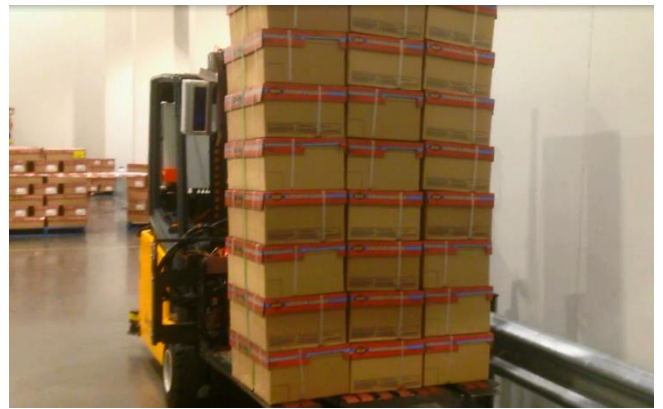
Figure 25: The AGV reverses and lowers the stack before moving towards the designated container
