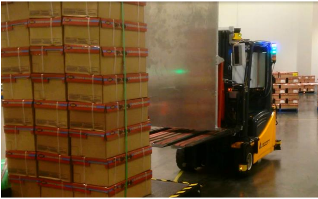
Figure 22: The AGV lowers the tynes to the height of the powered conveyor table
