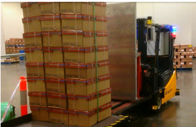
Figure 23: The powered conveyor table operates moving the stack onto the AGV tynes
