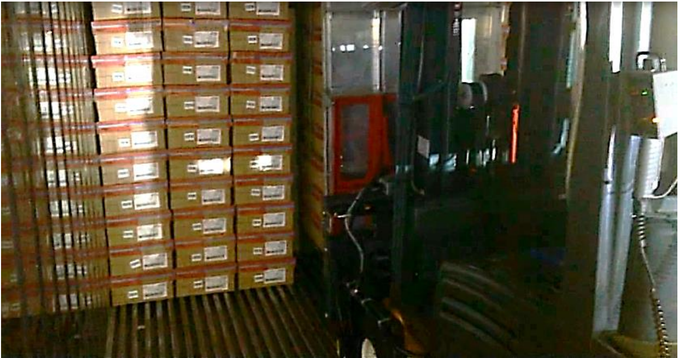
Figure 34: Placement of an adjacent stack within the container
