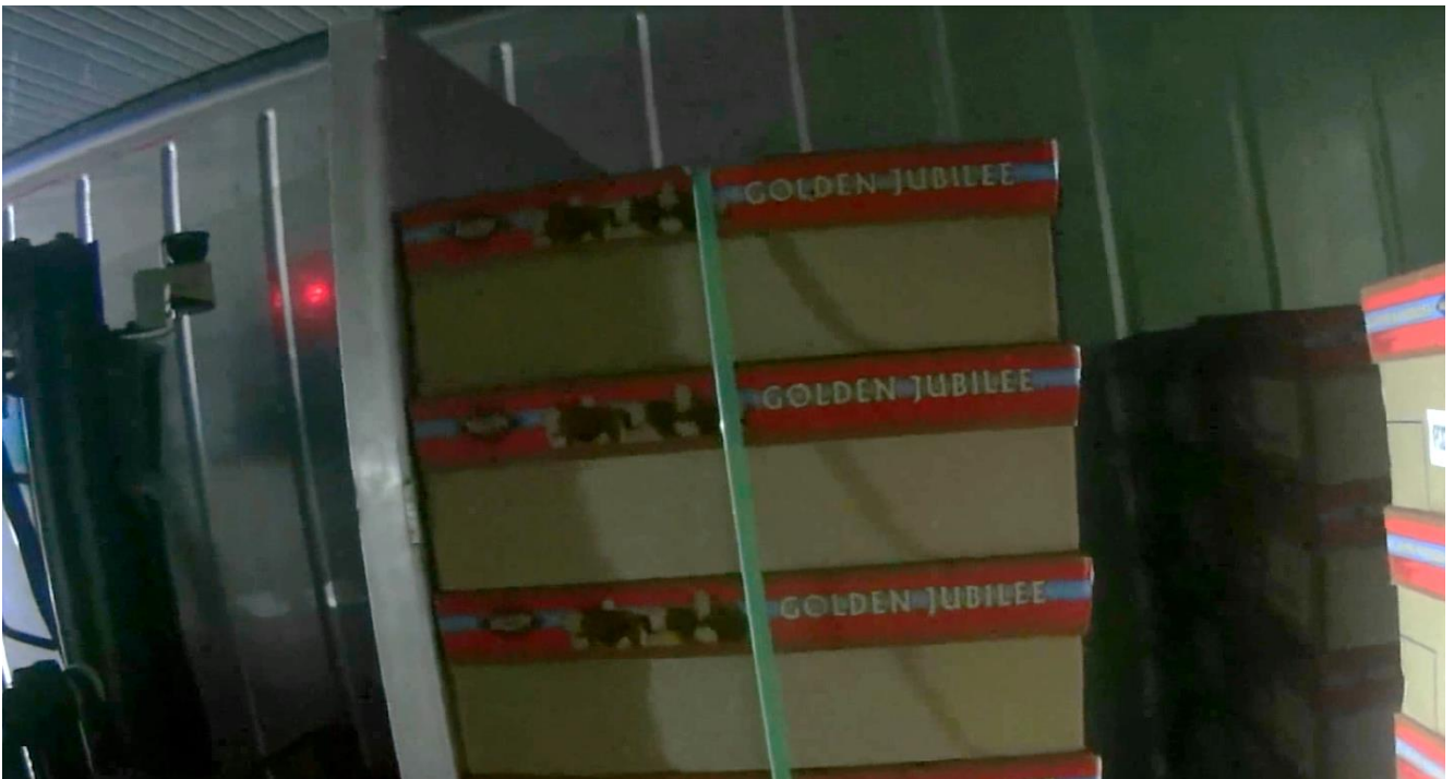
Figure 29: AGV approaches existing stack within container. Stack is side shifted, lowered and placed up against the existing stack
