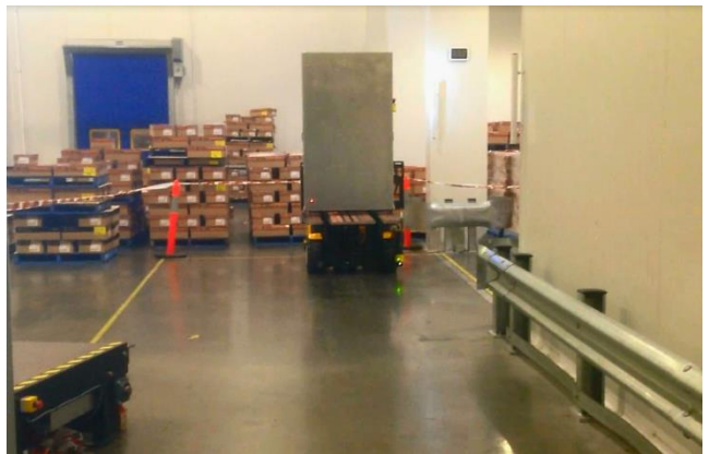
Figure 32: As the AGV returns to the home position the tynes and pusher plate reset into the start position
