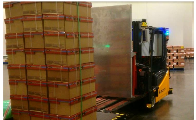
Figure 22: The AGV lowers the tynes to the height of the powered conveyor table
