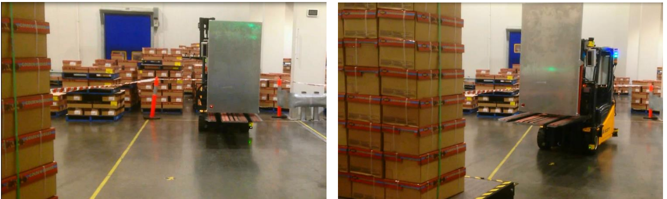
Figure 21: From the starting position the AGV approaches the stack
