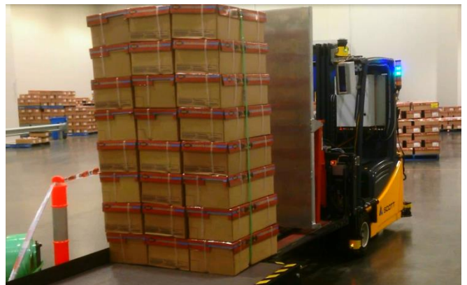
Figure 23: The powered conveyor table operates moving the stack onto the AGV tynes
