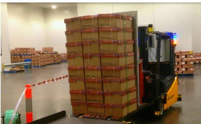
Figure 24: The AGV simultaneously raises the stack and reverses
