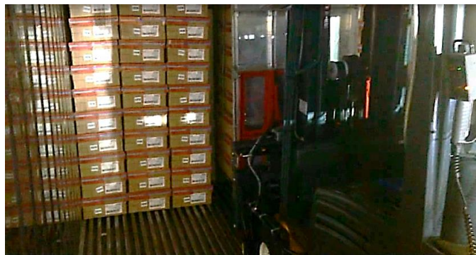
Figure 1: Placement of an adjacent stack within the container using the current Scott Automated Guided Vehicle (AGV)
