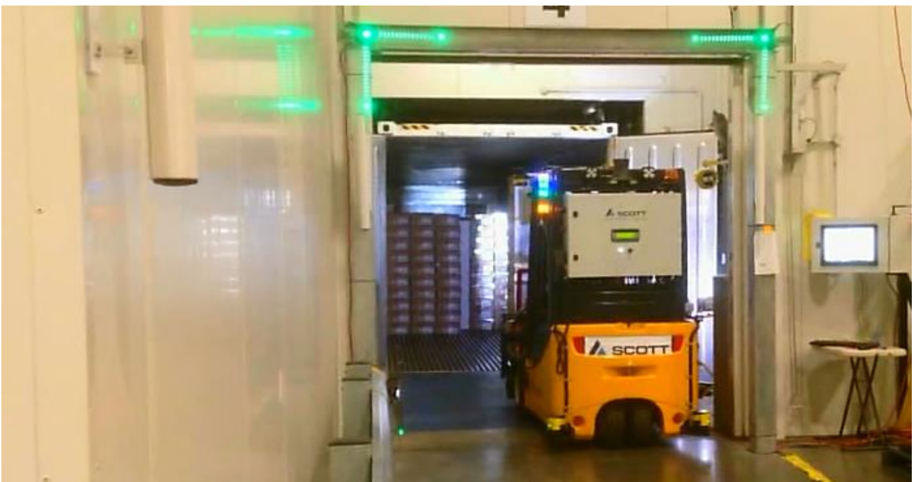
Figure 33: The AGV returning to the container to position the adjacent stack
