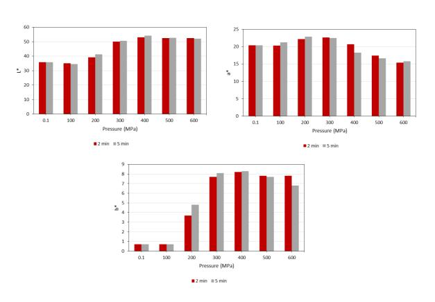
**Figure 1.** Colour parameters (L\*, a\* and b\*) of beef striploin muscle after treatment (Control, 0.1 MPa vs 100, 200, 300, 400, 500, 600 MPa HPP at ambient temperature for 2 and 5 min) using a Minolta CR-400 (n=6).
