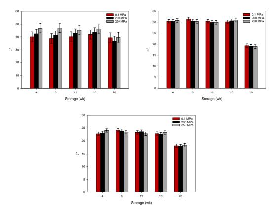
**Figure 4.** Effect of high pressure processing (HPP) at 0.1, 200 and 250 MPa and storage for 0, 4, 8, 12, 16 and 20 weeks at -1°C on surface colour of beef striploin muscle. Top left, lightness (L\*); top right, redness (a\*); and bottom, yellowness (b\*).
