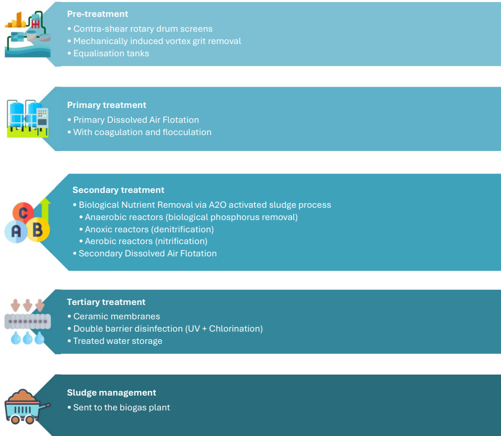
Figure 4. Summary of the WWTP design
