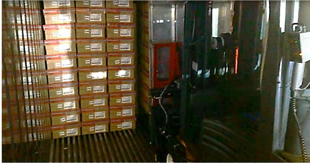
Figure 2: Placement of an adjacent stack within the container using the current Scott Automated Guided Vehicle (AGV)
