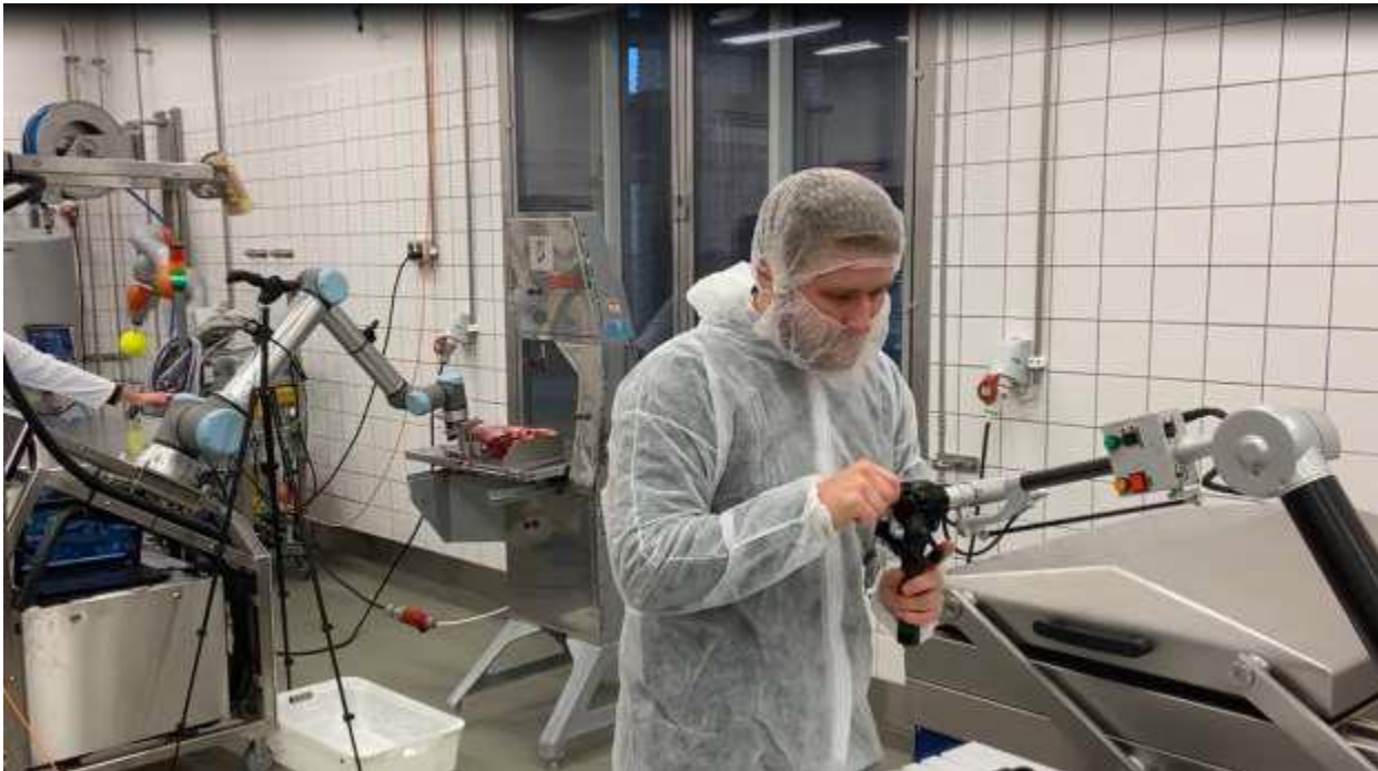
Figure 2. Remote cutting of shanks, monitoring the process on a screen.
