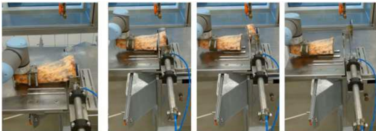
Figure 2. Cutting of slices in steps, with the actuator both serving as land and to push out the product after cutting.
