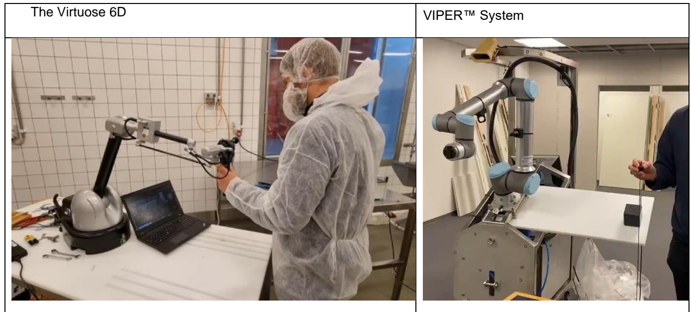
Figure 1. Telemanipulators used in project.
