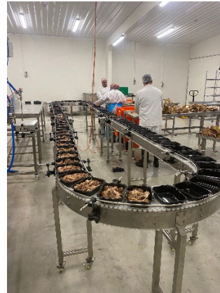
Carousel Conveyor improved work efficiency and hygiene of trays.
