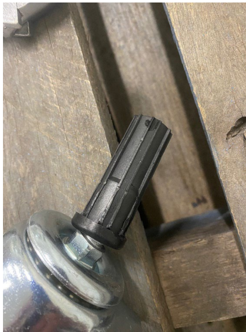
Castor failure for product trolley.
