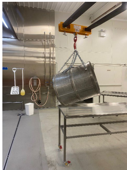
Experimenting with tipping basket onto sorting table after cooking.
