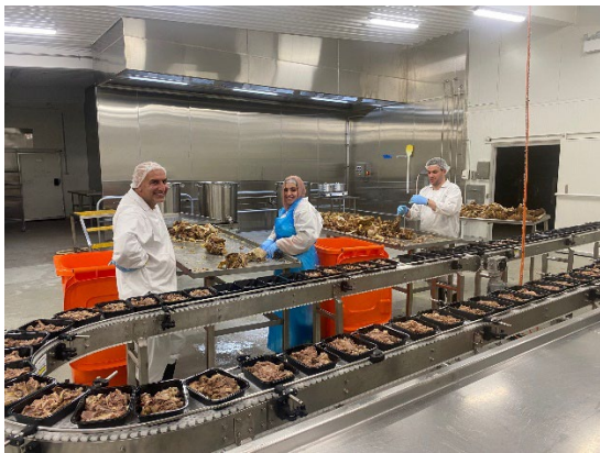
Carousel conveyor implemented to improve pack off efficiency and hygiene of trays.
