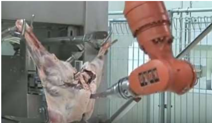
Figure 5.7: Leg deboning by Scott Technology.
