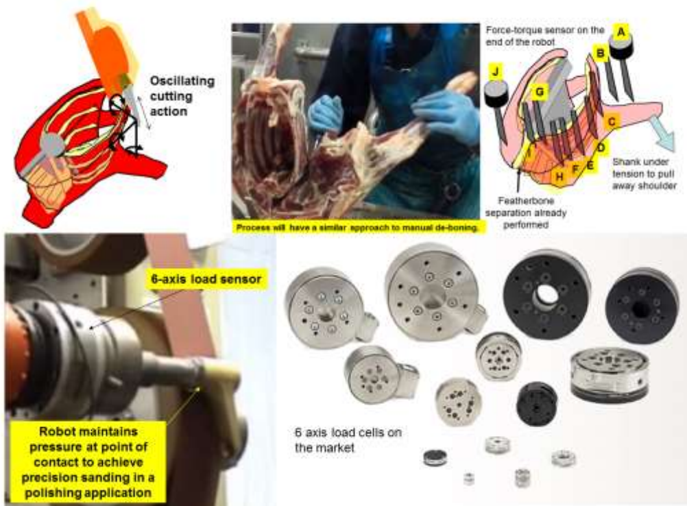
Figure 5.16: Force control using standard 6-axis load cell between the robot tool flange and the knife (see Figure 5.15B).
