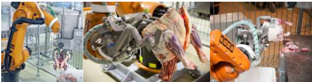
Figure 5.6: Robot holds shoulder primal, driving it against fixed blades to perform de-boning (Scott Technology solution).
